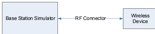
Figure 8-1 Power Measurement Setup
