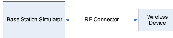
Figure 8-2 Power Measurement Setup
