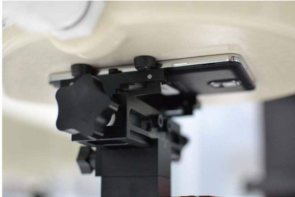
SAR Test Setup Photo 6: Front Side at 0.0 cm
