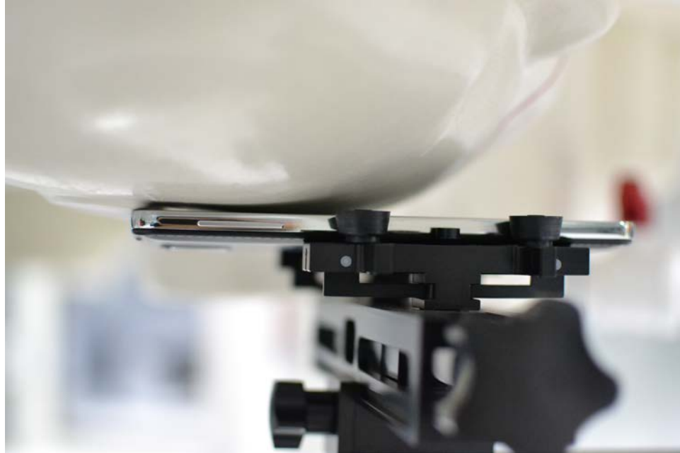
SAR Test Setup Photo 1: Right Cheek
