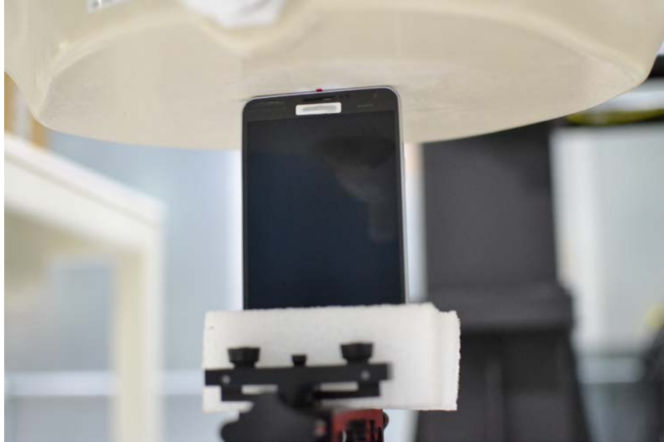
SAR Test Setup Photo 7: Top Edge at 0.0 cm
