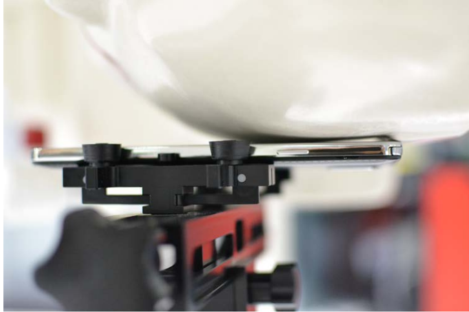
SAR Test Setup Photo 3: Left Cheek
