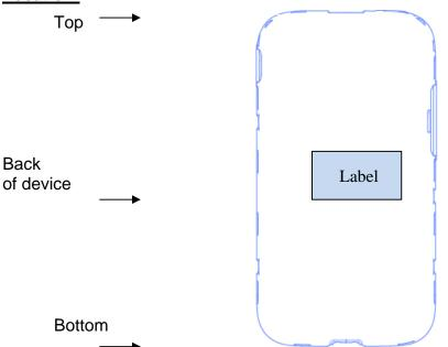
Label is placed inside of the battery compartment.
