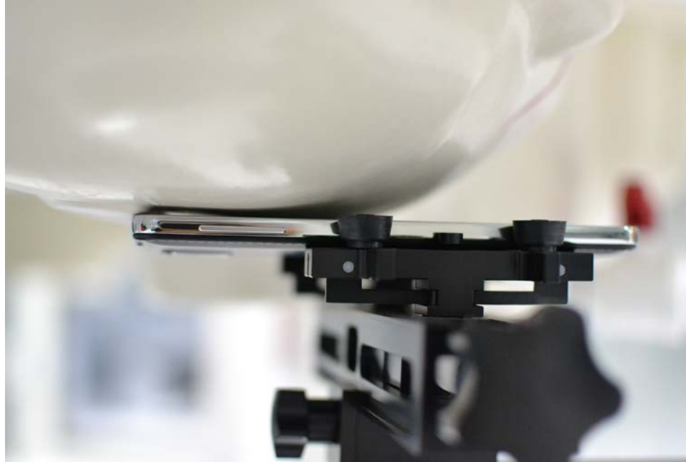
SAR Test Setup Photo 1: Right Cheek
