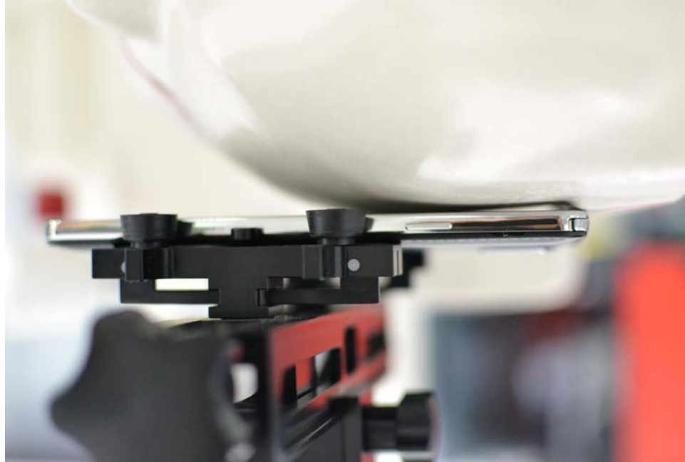
SAR Test Setup Photo 3: Left Cheek
