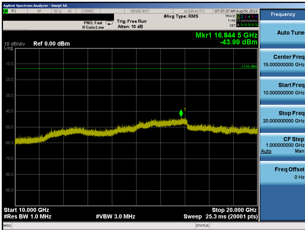
Plot 8-10. Conducted Spurious Plot (5.0MHz QPSK – RB Size 1, RB Offset 0 – High Channel)
