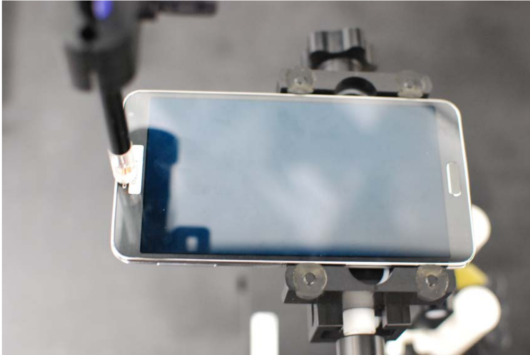
Figure 13-1 Test Setup for Wireless Device
