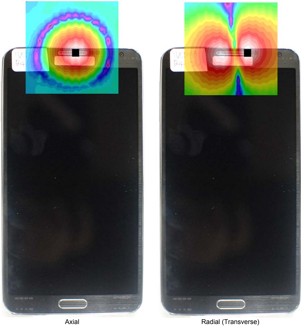
Figure 13-3 T-Coil Scan Overlay Magnetic Field Distributions
