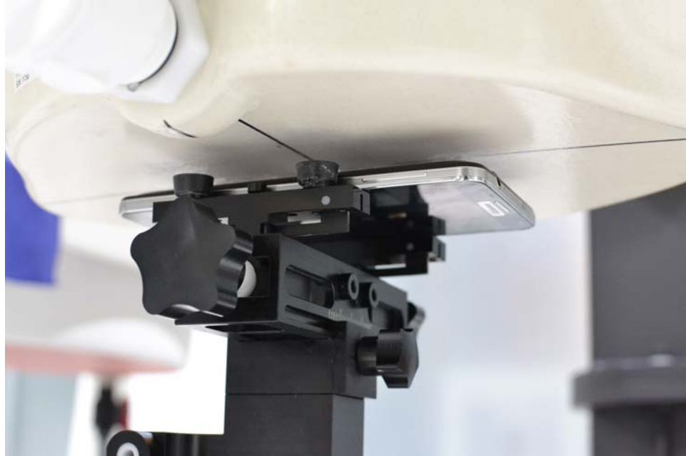
SAR Test Setup Photo 7: Back Side at 1.0 cm with Wireless Charging Cover
