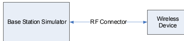
Figure 9-1 Power Measurement Setup
