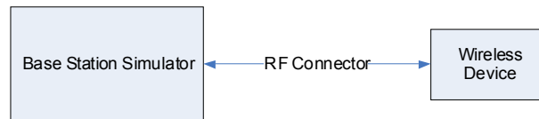
Figure 9-2 Power Measurement Setup
