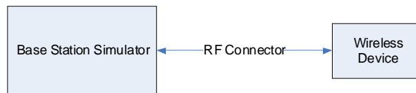
Figure 9-2 Power Measurement Setup
