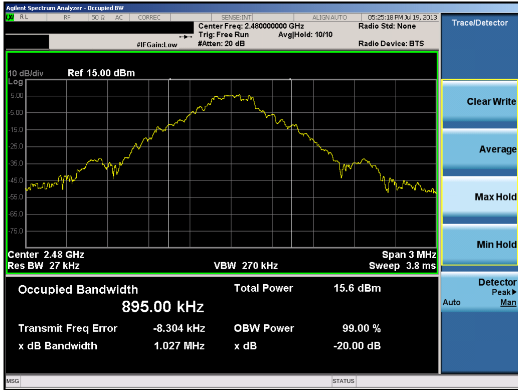
Plot 6-3. 20dB Bandwidth Plot (Bluetooth, 1Mbps – Ch. 78)
