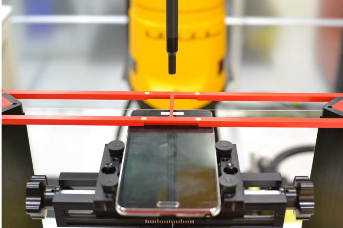
Figure 18-1 Ear Reference Point HAC Phantom Alignment
