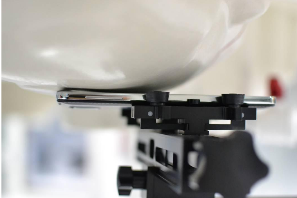
SAR Test Setup Photo 1 – Right Cheek
