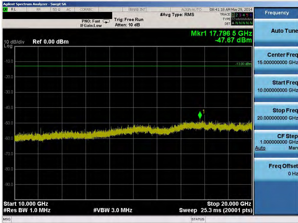
Plot 7-34. Conducted Spurious Plot (15.0MHz QPSK – RB Size 1, RB Offset 0 – Low Channel)
