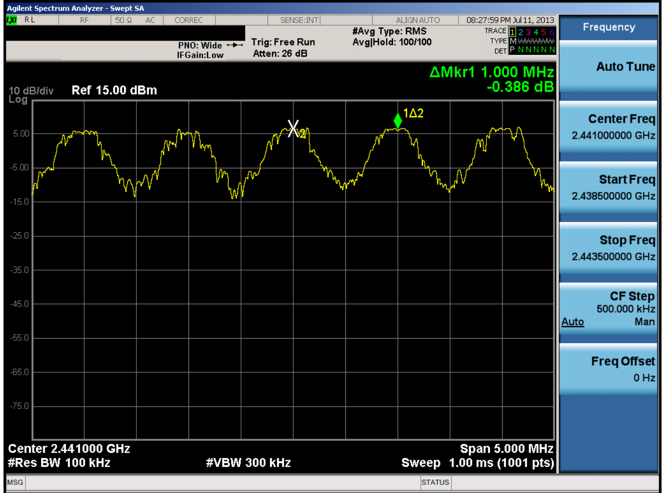
Plot 6-32. Channel Spacing Plot (Bluetooth)
