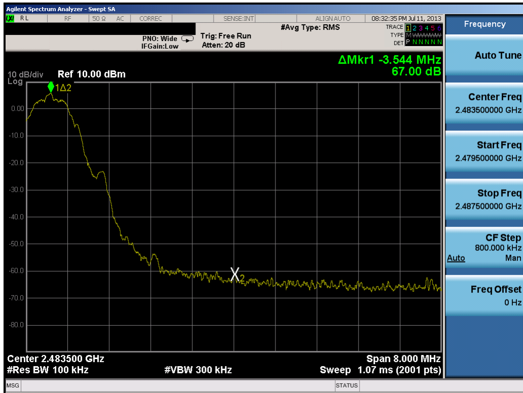
Plot 6-11. Band Edge Plot (Bluetooth (LE) – Ch. 39)
