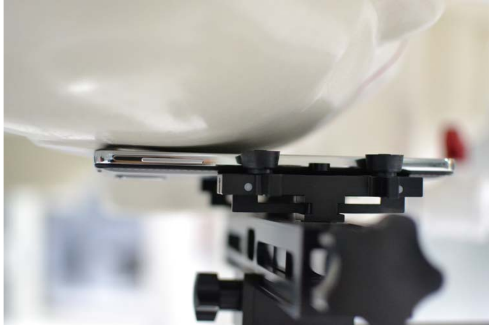
SAR Test Setup Photo 1: Right Cheek
