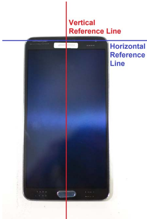
SAR Test Setup Photo 9: Horizontal and Vertical Reference Lines
