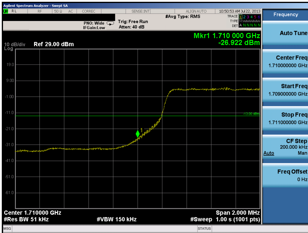
Plot 9-29. Lower Band Edge Plot (5.0MHz QPSK – RB Size 25)
