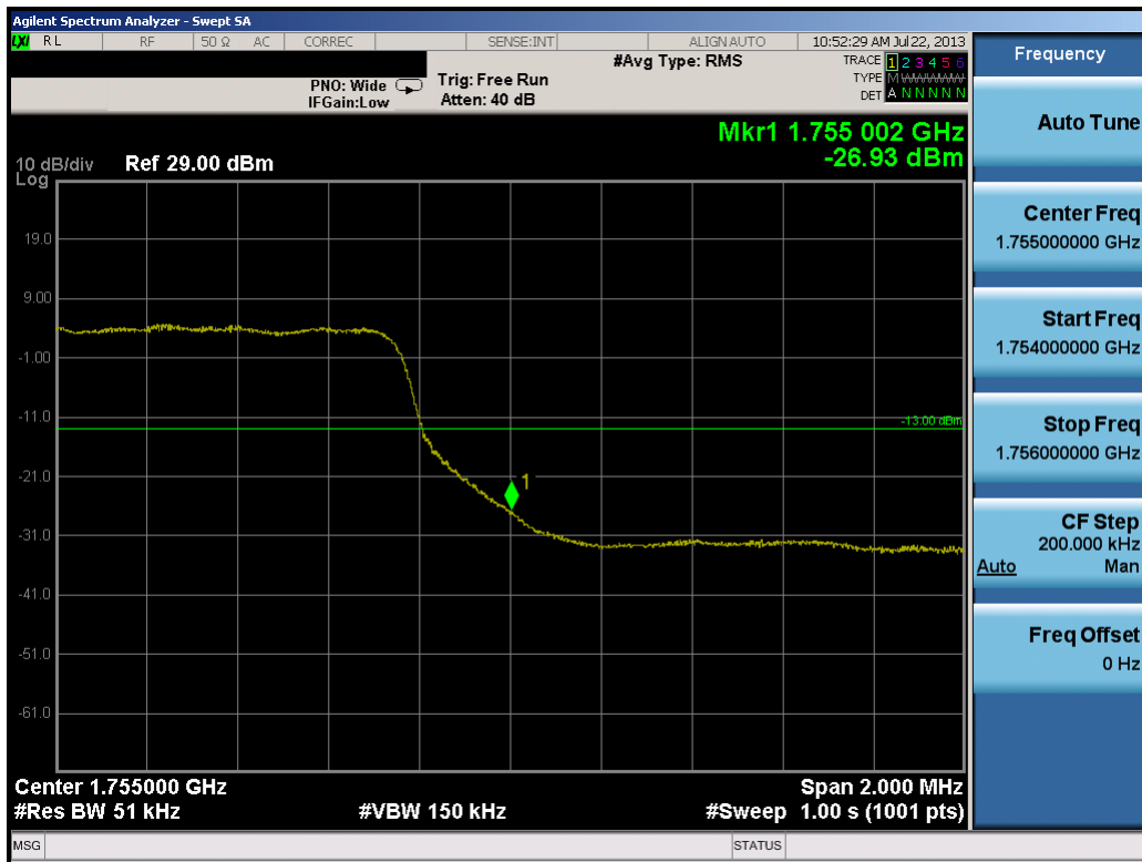
Plot 9-39. Upper Band Edge Plot (5.0MHz QPSK – RB Size 25)
