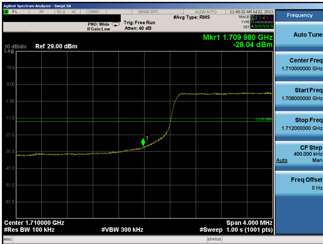
Plot 9-43. Lower Band Edge Plot (10.0MHz QPSK – RB Size 50)
