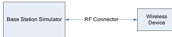
Figure 8-1 Power Measurement Setup
