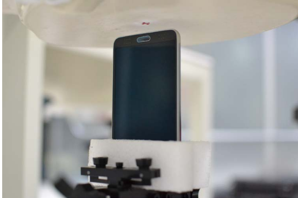
SAR Test Setup Photo 11: Bottom Edge at 1.0 cm
