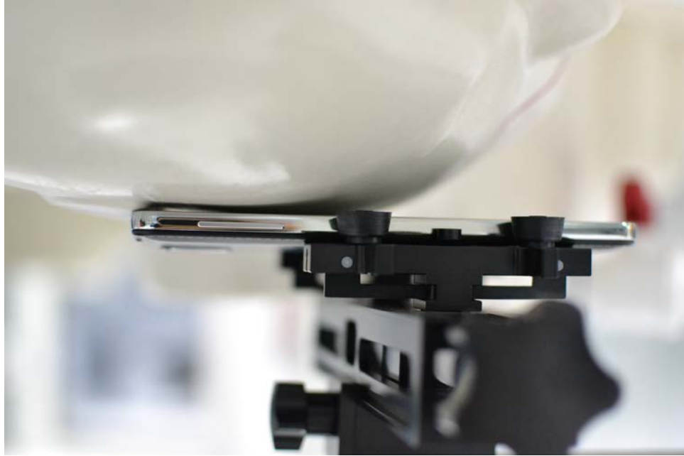
SAR Test Setup Photo 1: Right Cheek
