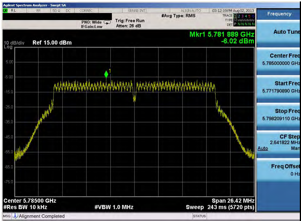
Plot 6-33. Power Spectral Density Plot (20MHz BW 802.11n (5.8GHz) – Ch. 157)
