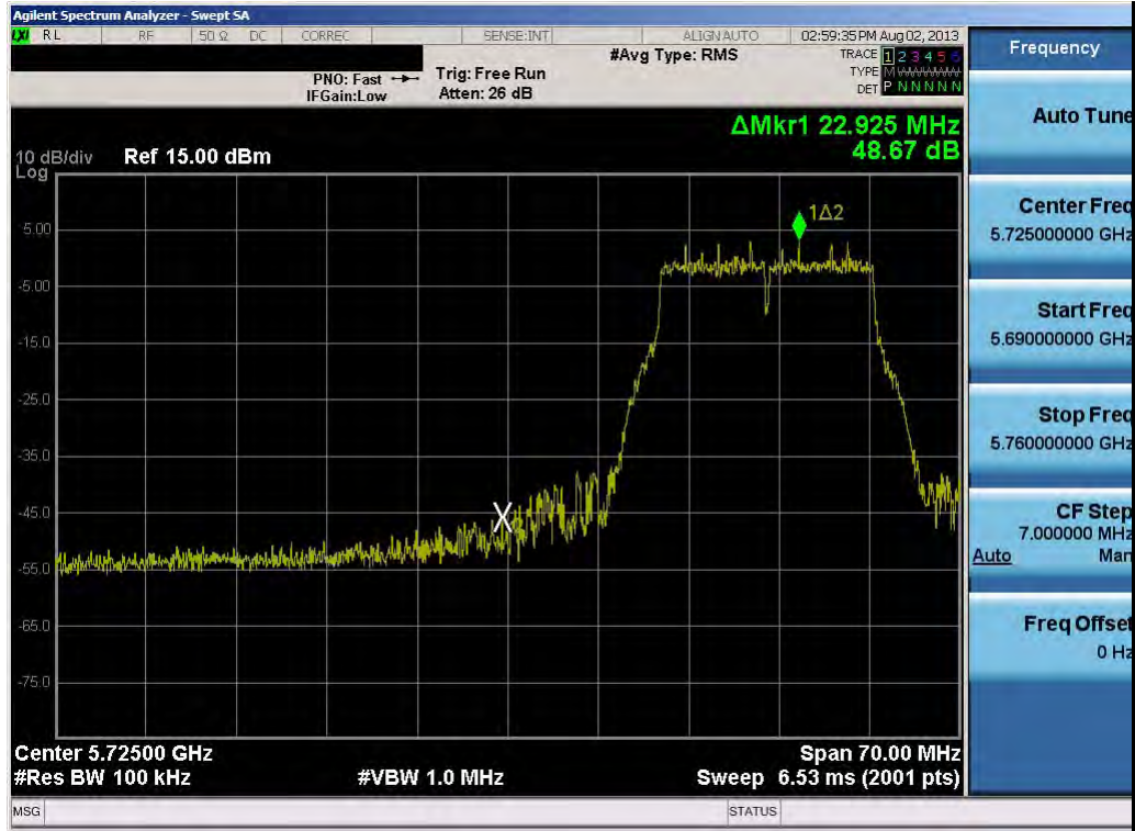
Plot 6-45. Band Edge Plot (802.11a – Ch. 149)
