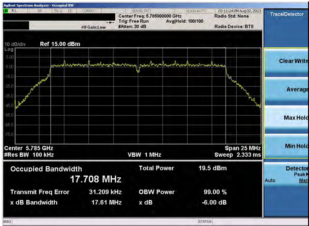
Plot 6-14. 6dB Bandwidth Plot (20MHz BW 802.11n (5.8GHz) – Ch. 157)
