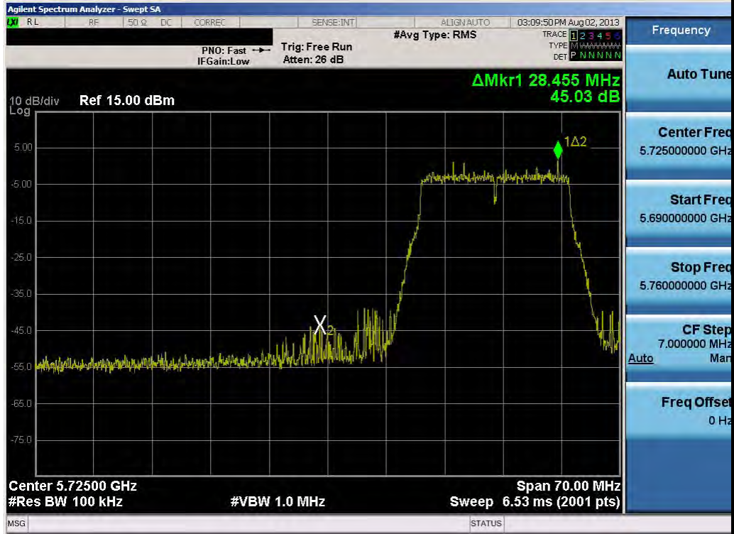
Plot 6-47. Band Edge Plot (20MHz BW 802.11n (5.8GHz) – Ch. 149)
