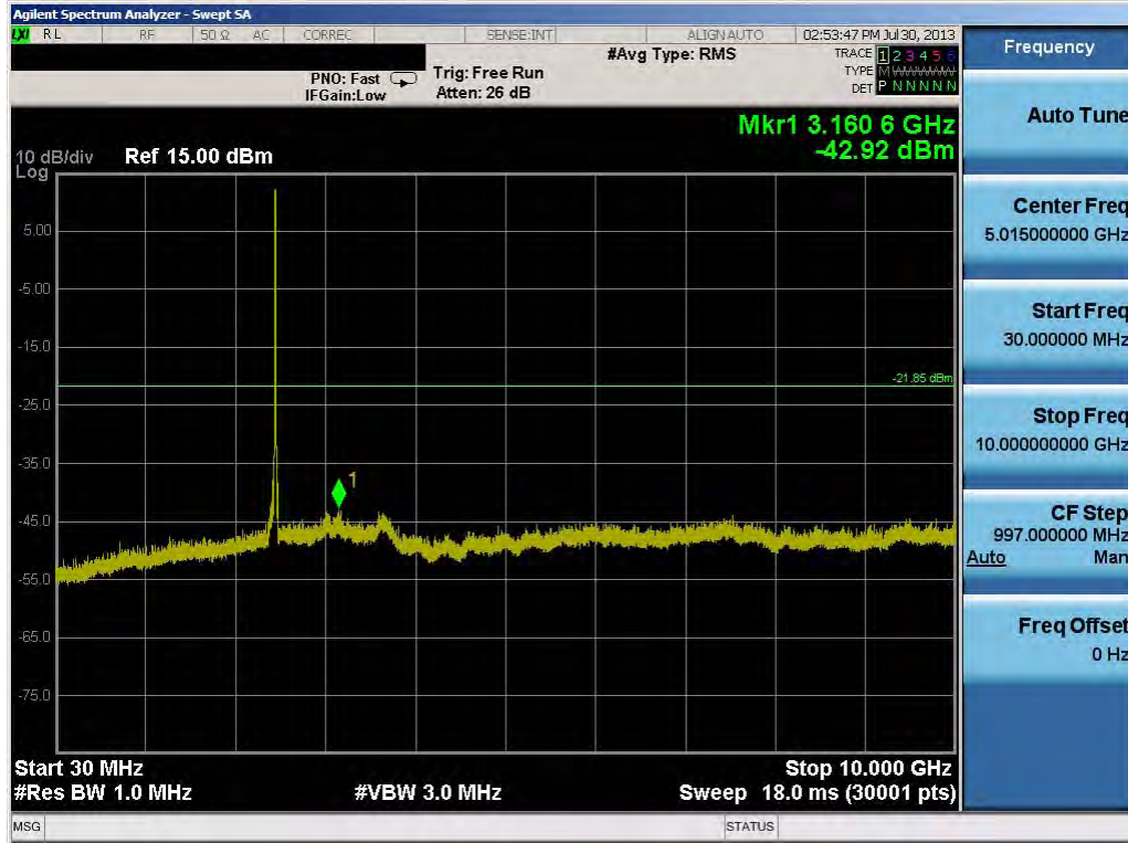
Plot 6-57. Conducted Spurious Plot (802.11b – Ch. 11)
