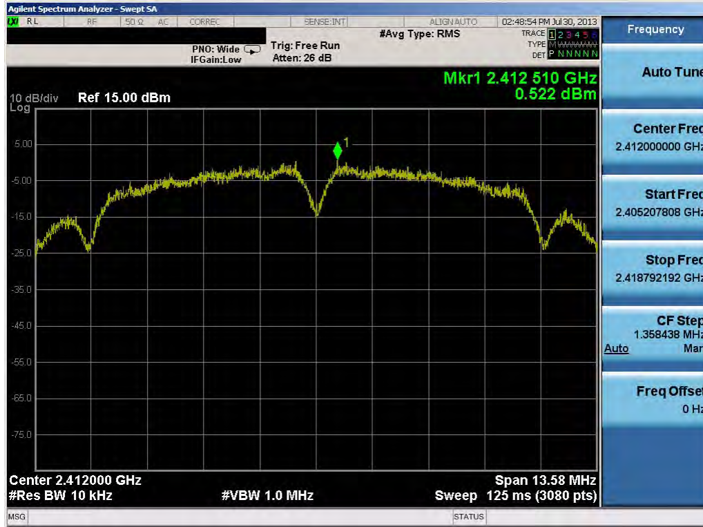
Plot 6-20. Power Spectral Density Plot (802.11b – Ch. 1)
