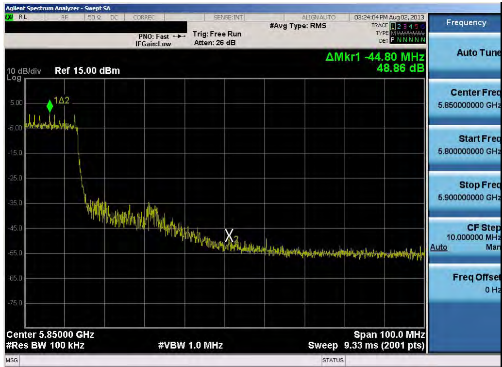
Plot 6-50. Band Edge Plot (40MHz BW 802.11n (5.8GHz) – Ch. 163)
