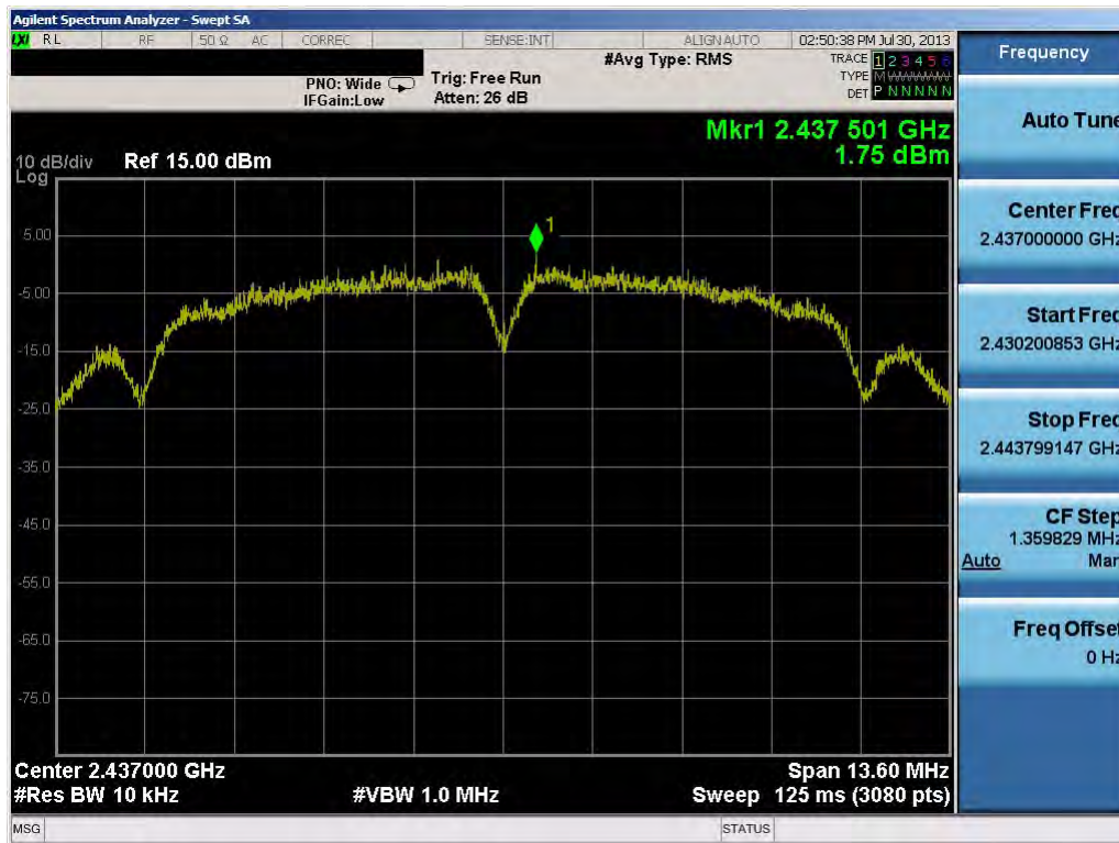
Plot 6-21. Power Spectral Density Plot (802.11b – Ch. 6)
