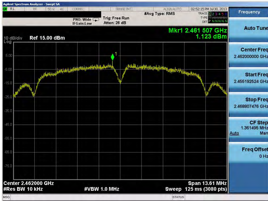
Plot 6-22. Power Spectral Density Plot (802.11b – Ch. 11)
