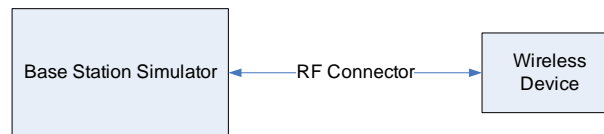
Figure 8-2 Power Measurement Setup
