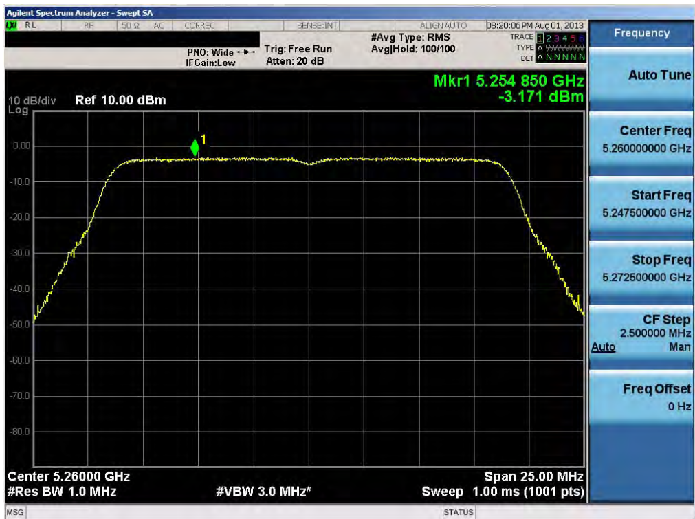
Plot 6-43. Peak Power Spectral Density Plot (20MHz BW 802.11n (UNII Band 2) – Ch. 52)
