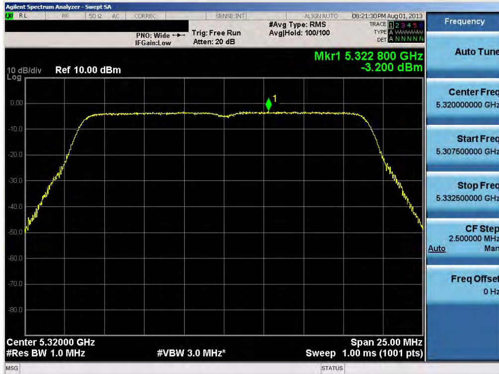
Plot 6-45. Peak Power Spectral Density Plot (20MHz BW 802.11n (UNII Band 2) – Ch. 64)
