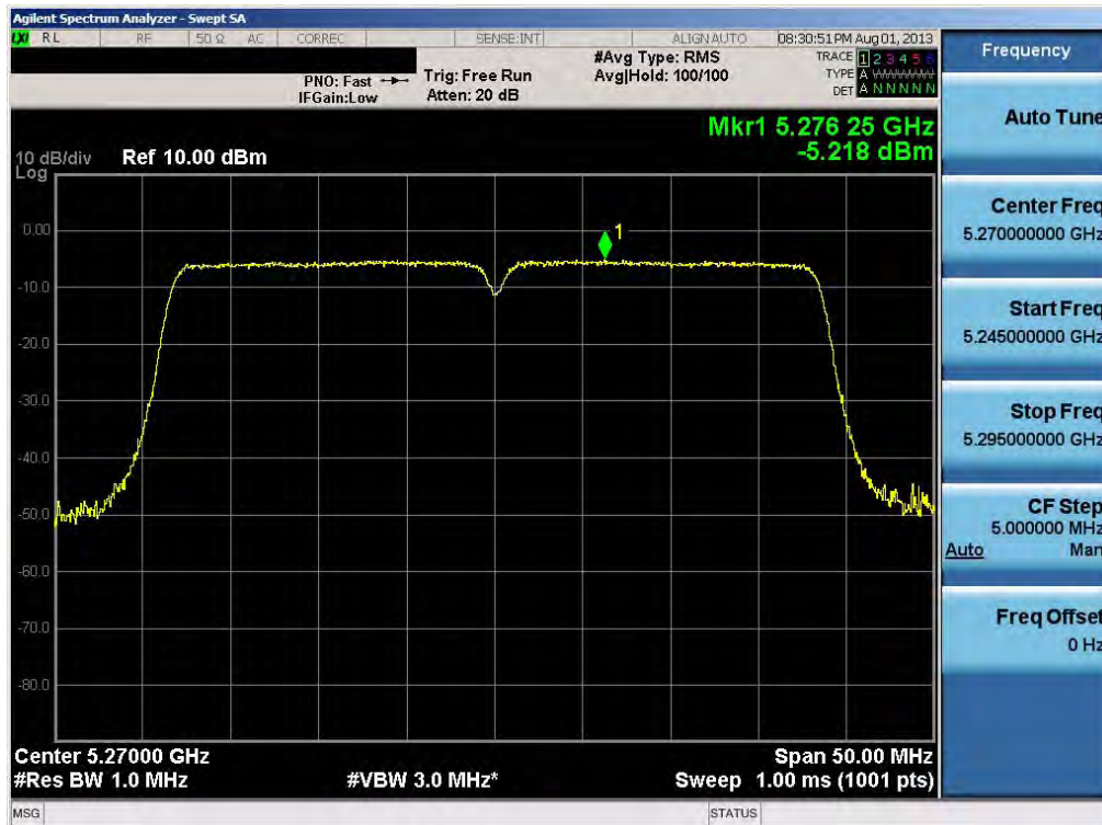
Plot 6-46. Peak Power Spectral Density Plot (40MHz BW 802.11n (UNII Band 2) – Ch. 54)
