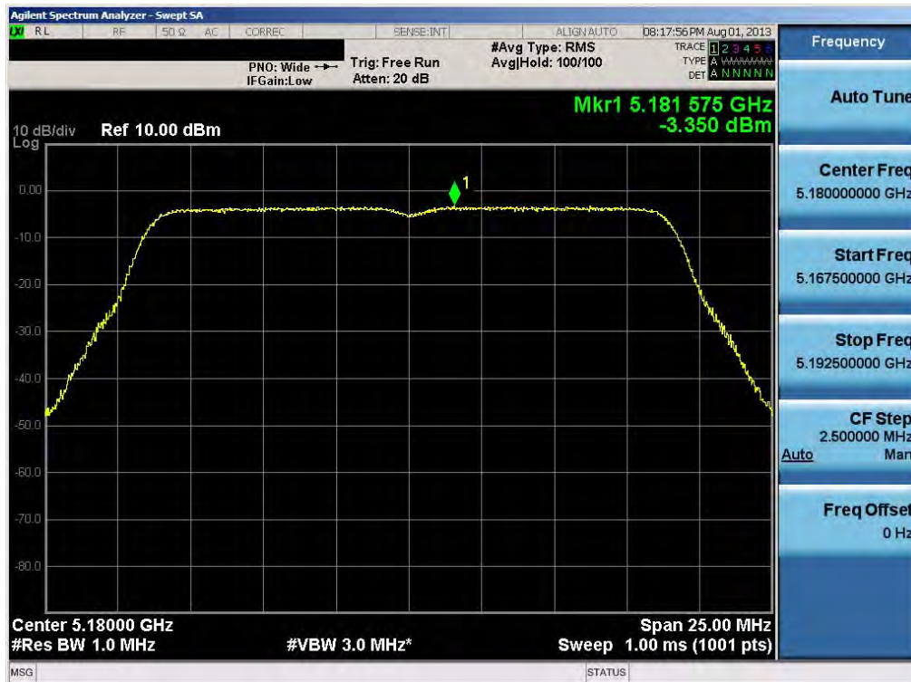
Plot 6-34. Peak Power Spectral Density Plot (20MHz BW 802.11n (UNII Band 1) – Ch. 36)
