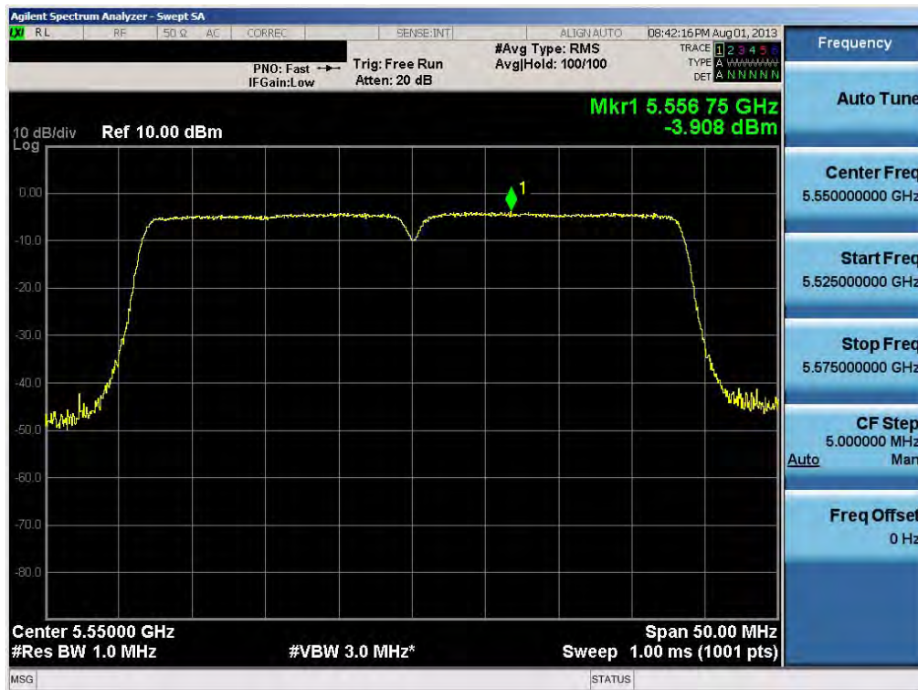
Plot 6-56. Peak Power Spectral Density Plot (40MHz BW 802.11n (UNII Band 3) – Ch. 110)
