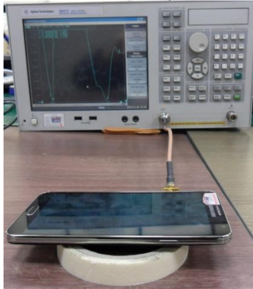
Figures 2-1. Measurement setup of SM-N7506V BT/Wi-Fi antenna.
