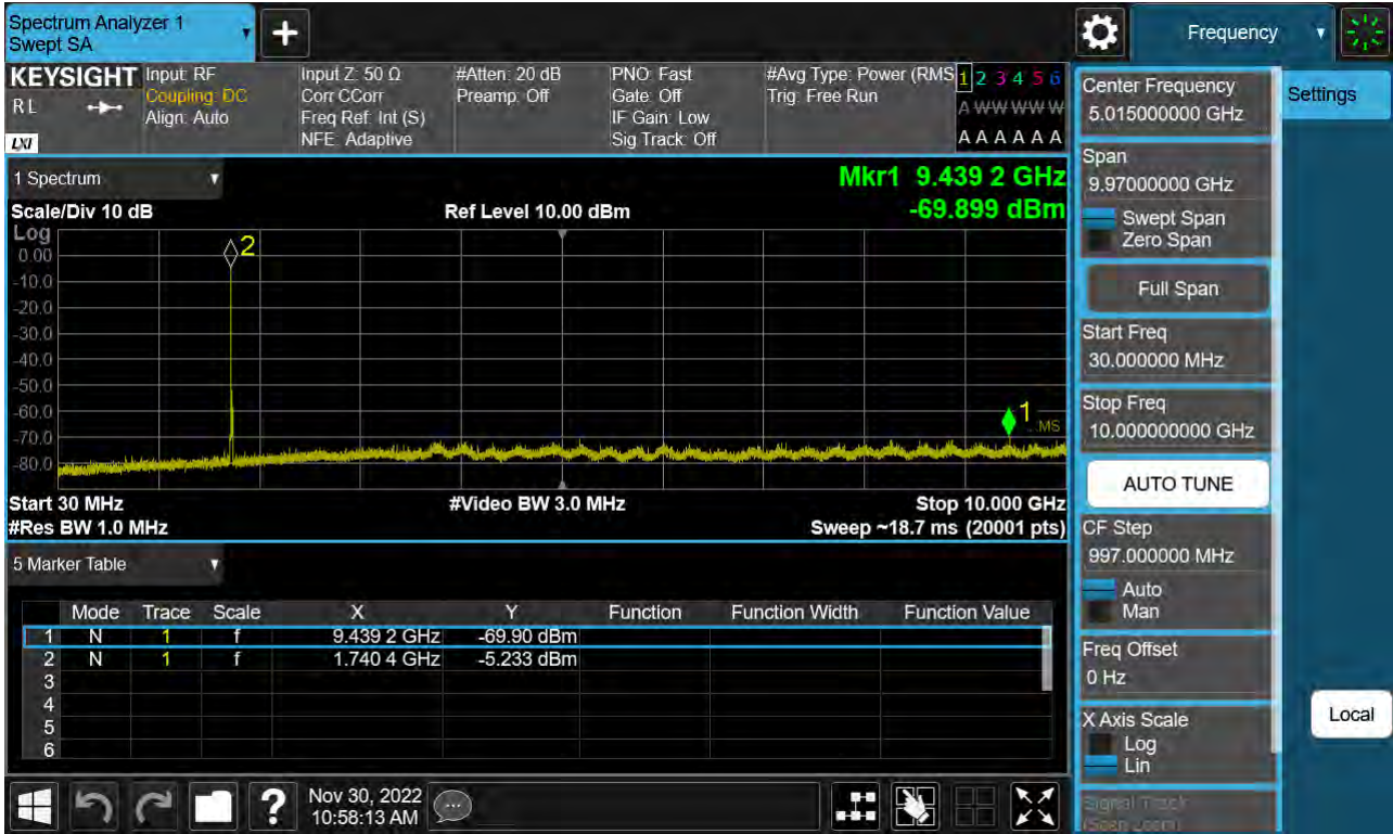
Sub6 n66. Conducted Spurious Plot_1 (349000ch_10 MHz_BPSK_RB 1_1)
