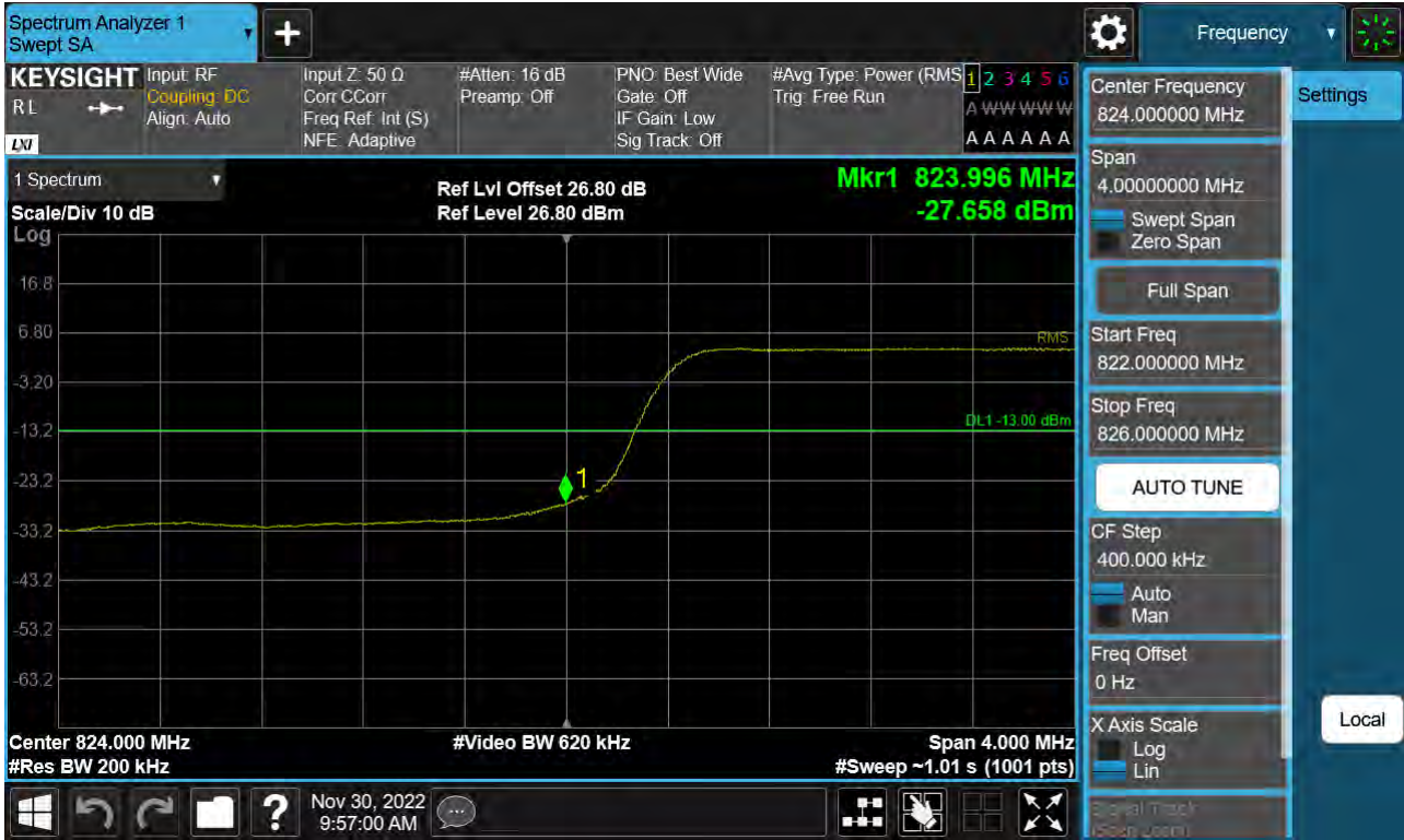
Sub6 n5. Lower Band Edge Plot (20 M BW Ch.166800 BPSK_RB100_Offset 0)
