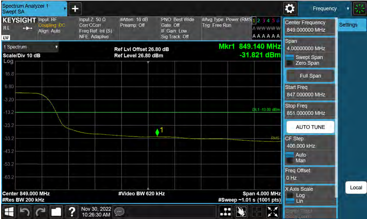
Sub6 n5. Upper Band Edge Plot (20 M BW Ch.167800 BPSK_RB100_Offset 0)
