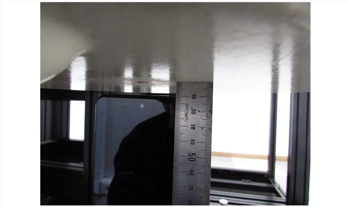
Distance of 10 mm from the EUT
