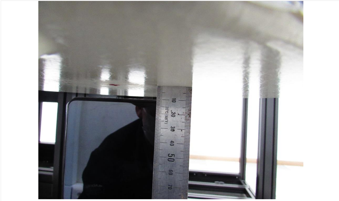
Distance of 10 mm from the EUT
