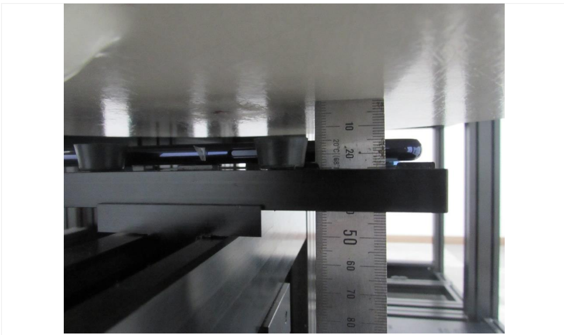
Distance of 15 mm from the EUT
