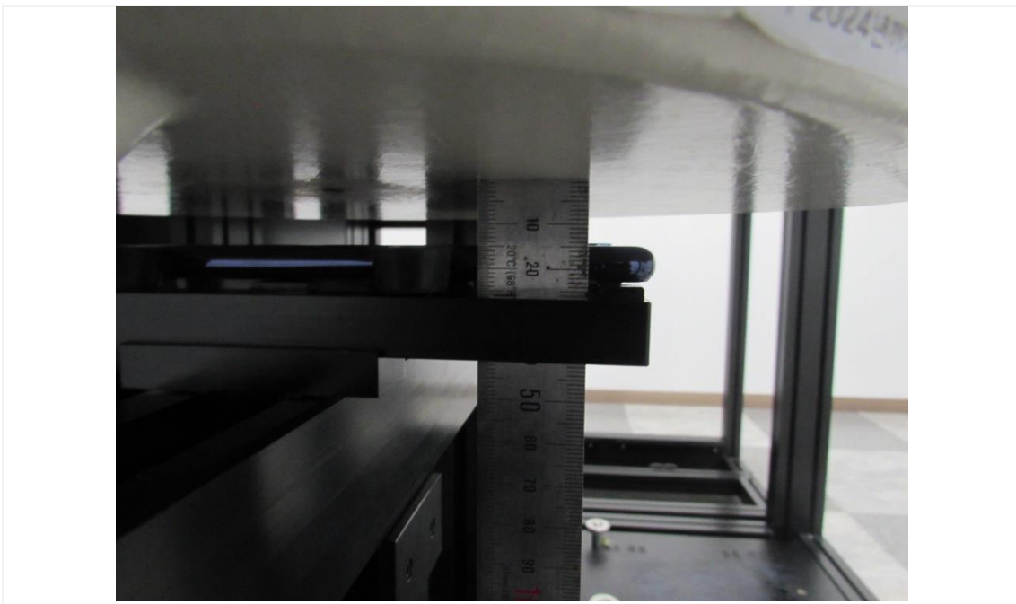
Distance of 15 mm from the EUT
