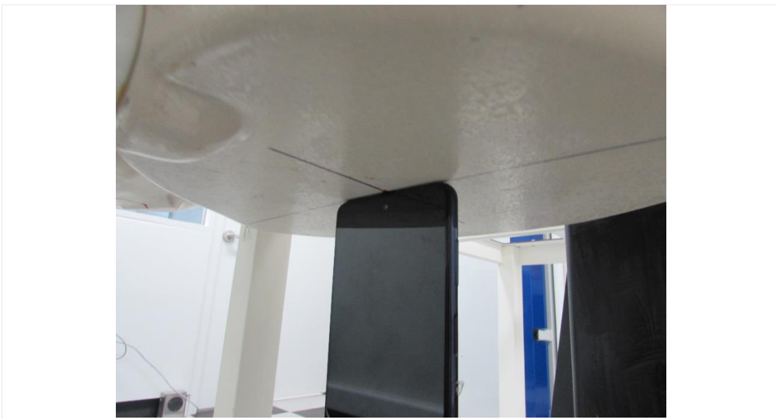
Distance of 0 mm from the EUT
