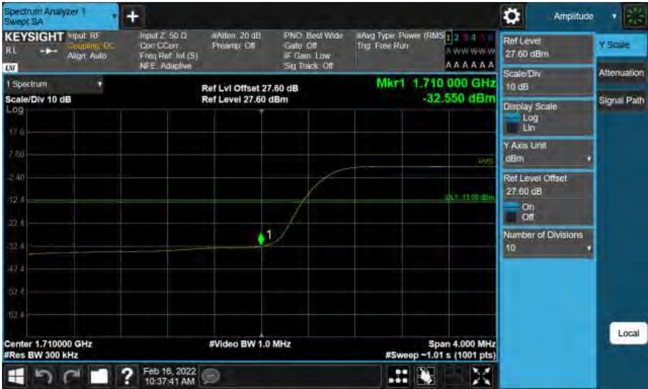
Sub6 n66. Lower Band Edge Plot (30 M BW Ch.345000 BPSK Full RB) -2
