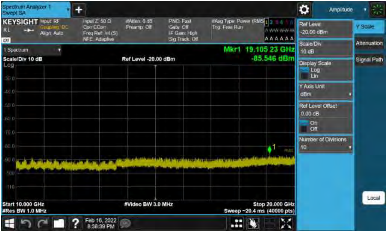
Sub6 n66. Conducted Spurious Plot_2 (349000ch_10 MHz_BPSK_RB 1_1)
