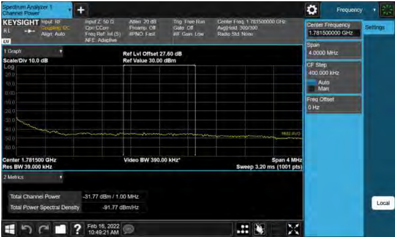
Sub6 n66. Upper Extended Band Edge Plot (40 M BW Ch.352000 BPSK_ Full RB) -3
