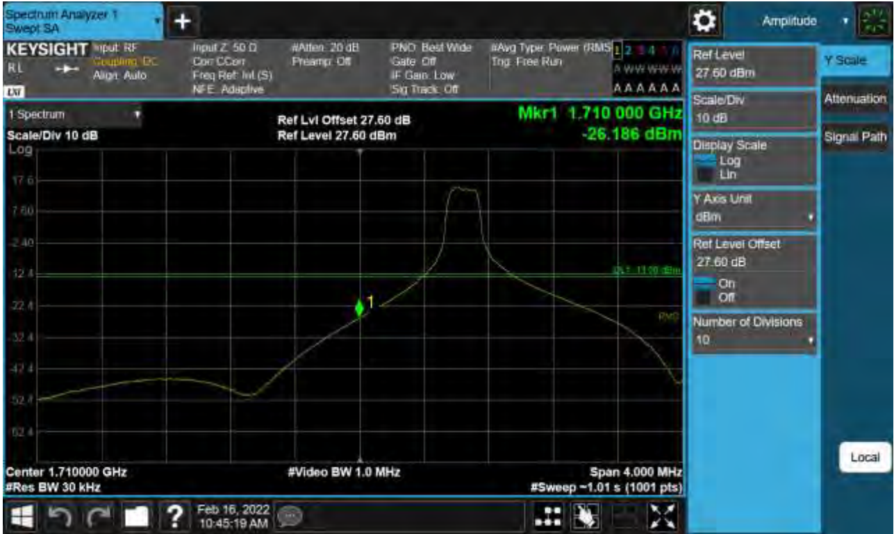
Sub6 n66. Lower Band Edge Plot (40 M BW Ch.346000 BPSK RB 1, Offset 0) -1
