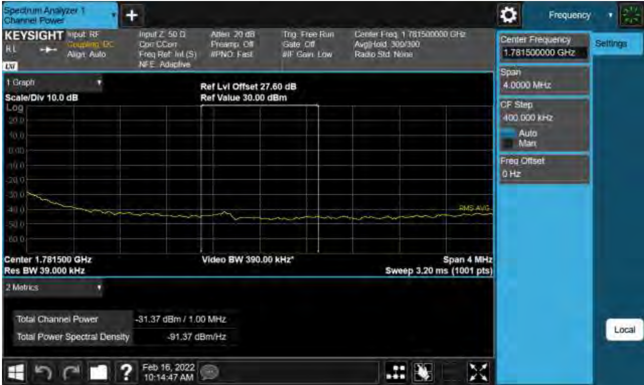
Sub6 n66. Upper Extended Band Edge Plot (10 M BW Ch.355000 BPSK_ Full RB) -3
