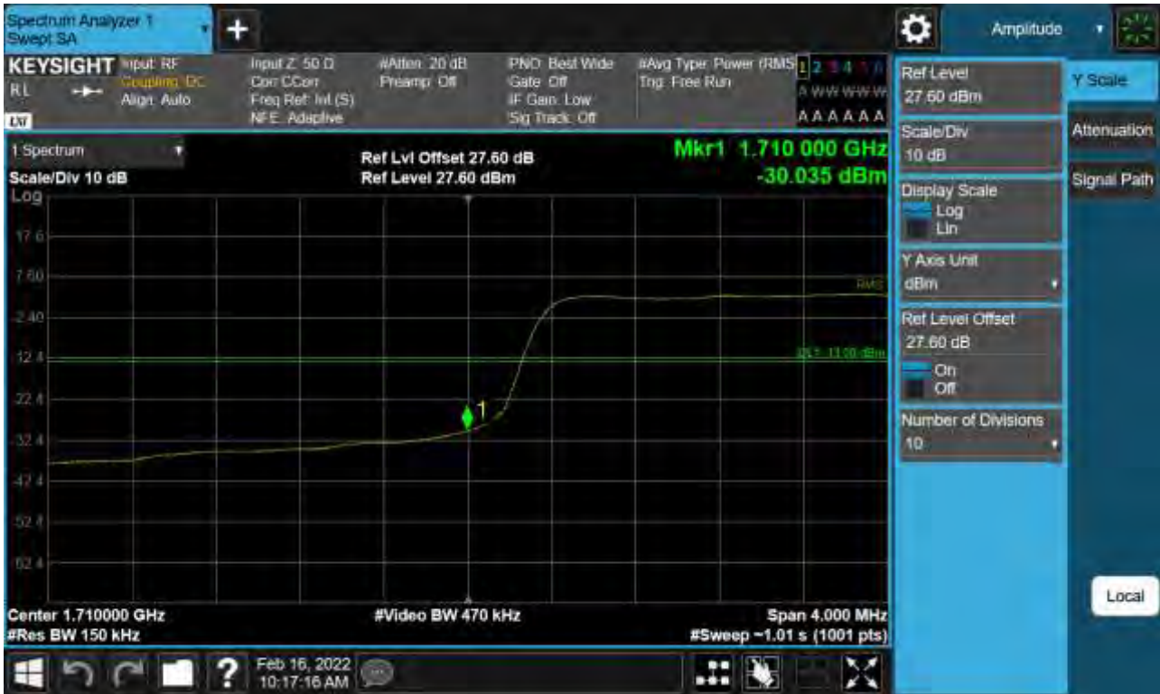
Sub6 n66. Lower Band Edge Plot (15 M BW Ch.343500 BPSK Full RB) -2
