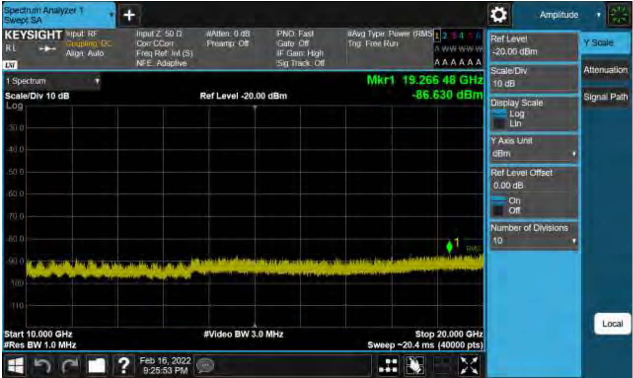
Sub6 n66. Conducted Spurious Plot_2 (349000ch_40 MHz_BPSK_RB 1_1)
