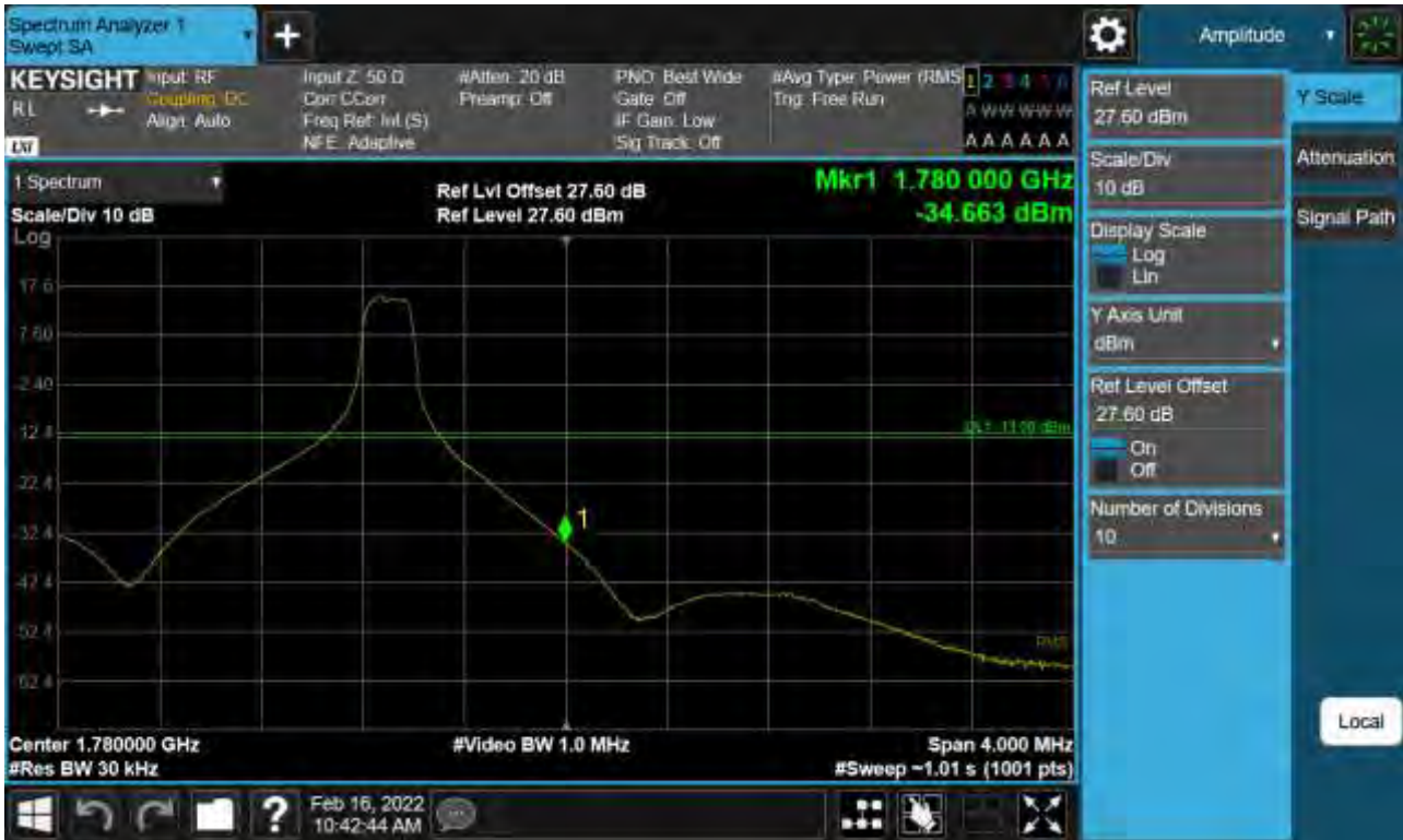
Sub6 n66. Upper Band Edge Plot (30 M BW Ch.353000 BPSK_RB1_Offset 159) -1
