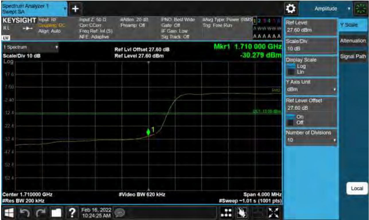
Sub6 n66. Lower Band Edge Plot (20 M BW Ch.344000 BPSK Full RB) -2
