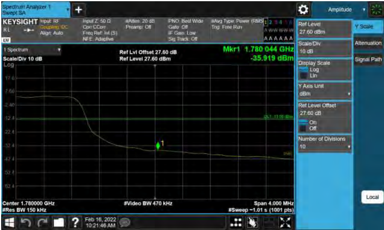
Sub6 n66. Upper Band Edge Plot (15 M BW Ch.354500 BPSK_ Full RB) -2
