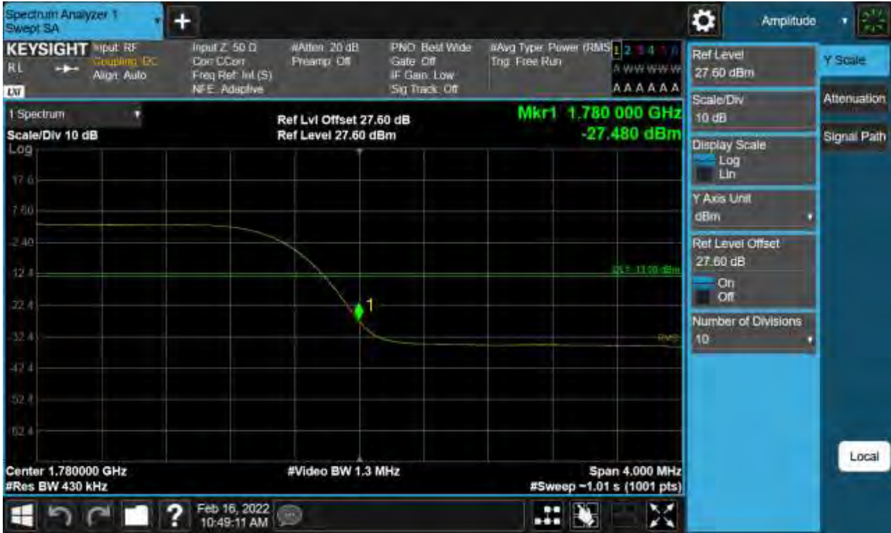
Sub6 n66. Upper Band Edge Plot (40 M BW Ch.352000 BPSK_ Full RB) -2
