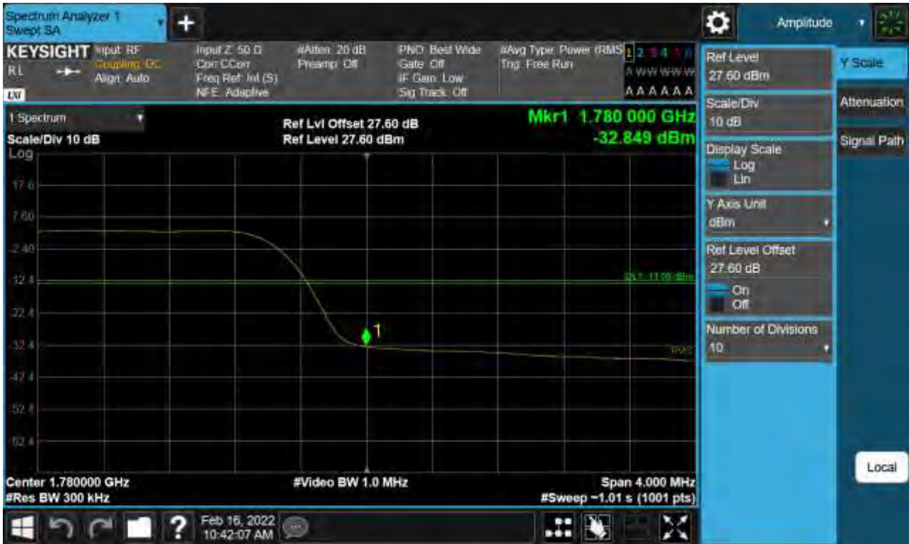
Sub6 n66. Upper Band Edge Plot (30 M BW Ch.353000 BPSK_ Full RB) -2
