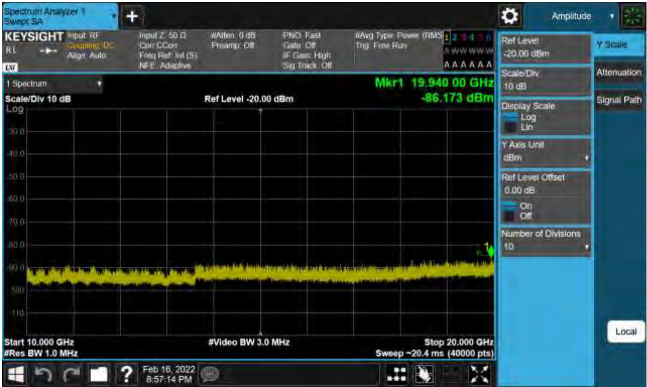
Sub6 n66. Conducted Spurious Plot_2 (354000ch_20 MHz_BPSK_RB 1_1)
