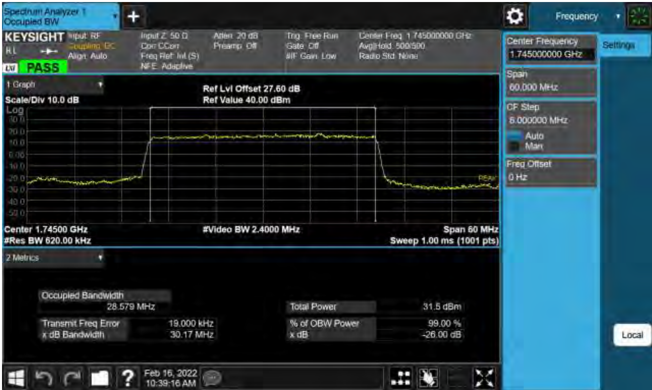
Sub6 n66. Occupied Bandwidth Plot (30 M BW Ch.349000 BPSK Full RB)
