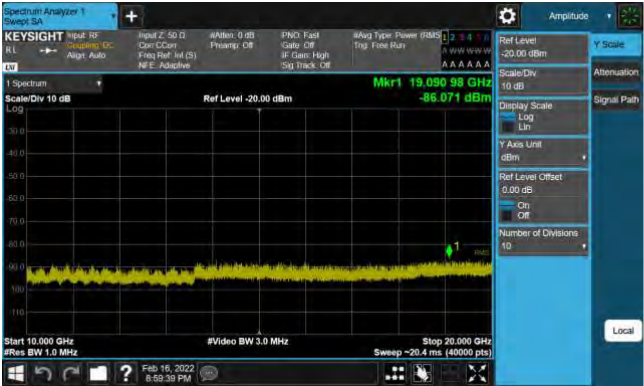
Sub6 n66. Conducted Spurious Plot_2 (344500ch_25 MHz_BPSK_RB 1_1)
