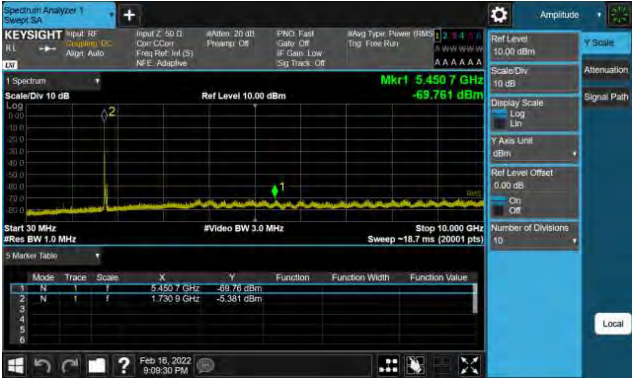
Sub6 n66. Conducted Spurious Plot_1 (349000ch_30 MHz_BPSK_RB 1_1)
