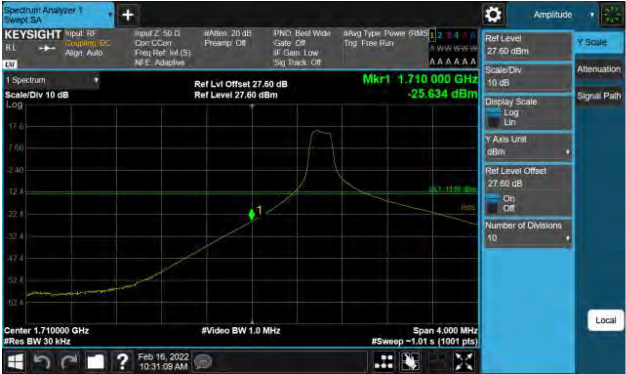
Sub6 n66. Lower Band Edge Plot (25 M BW Ch.344500 BPSK RB 1, Offset 0) -1
