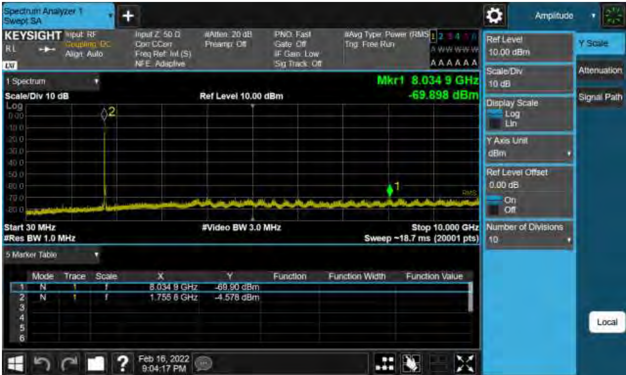
Sub6 n66. Conducted Spurious Plot_1 (353500ch_25 MHz_BPSK_ RB 1_1)
