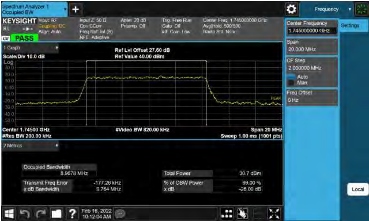
Sub6 n66. Occupied Bandwidth Plot (10 M BW Ch.349000 QPSK Full RB)
