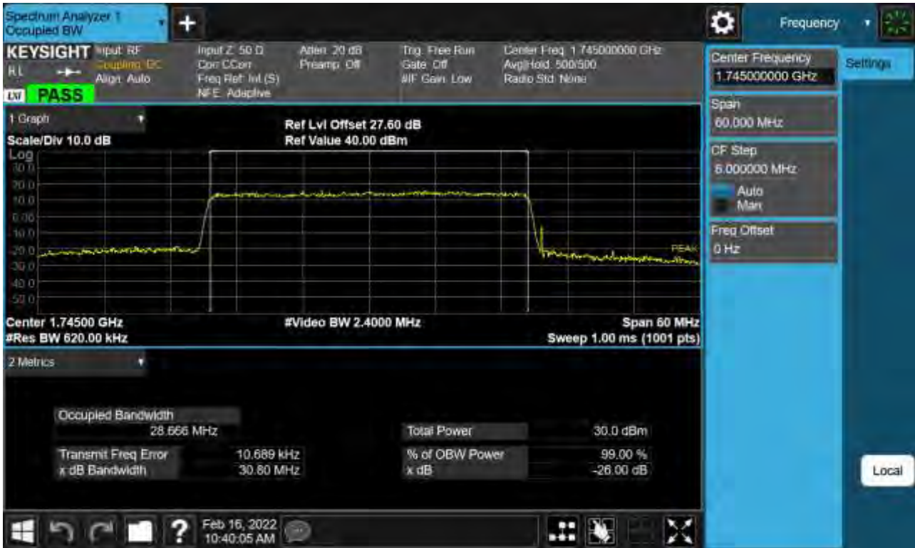
Sub6 n66. Occupied Bandwidth Plot (30 M BW Ch.349000 16QAM Full RB)
