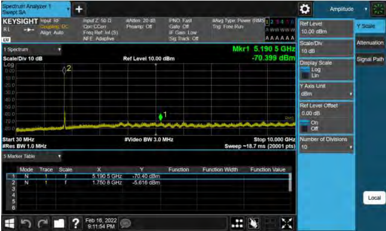
Sub6 n66. Conducted Spurious Plot_1 (353000ch_30 MHz_BPSK_RB 1_1)
