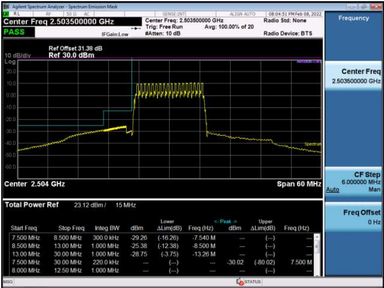
Low Channel Edge Plot (15 MHz Ch.39725 QPSK_RB75_Offset 0)-1
