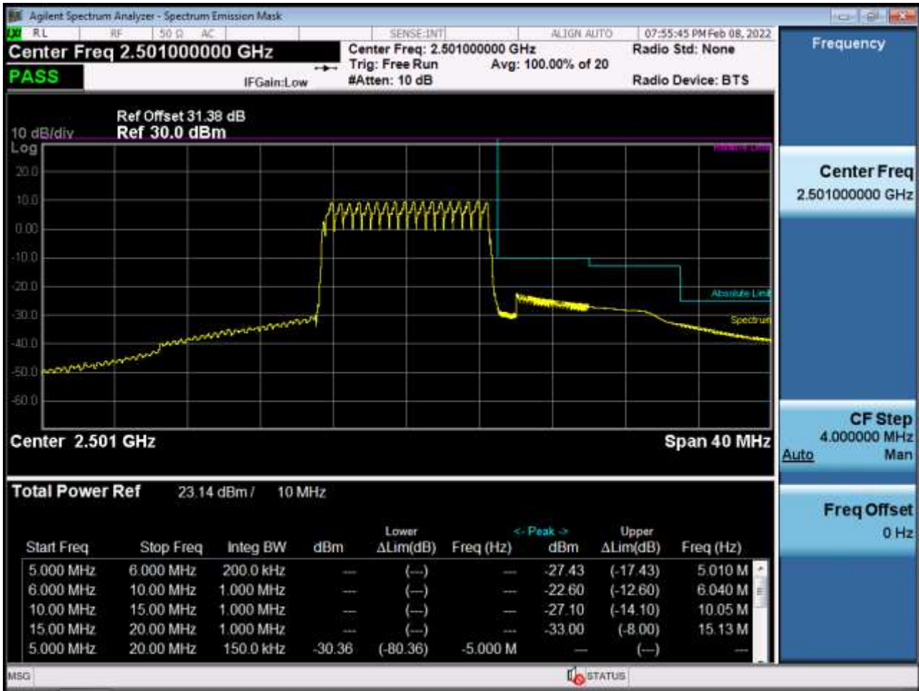
Low Channel Edge Plot (10 MHz Ch.39700 QPSK_RB50_Offset 0)-2
