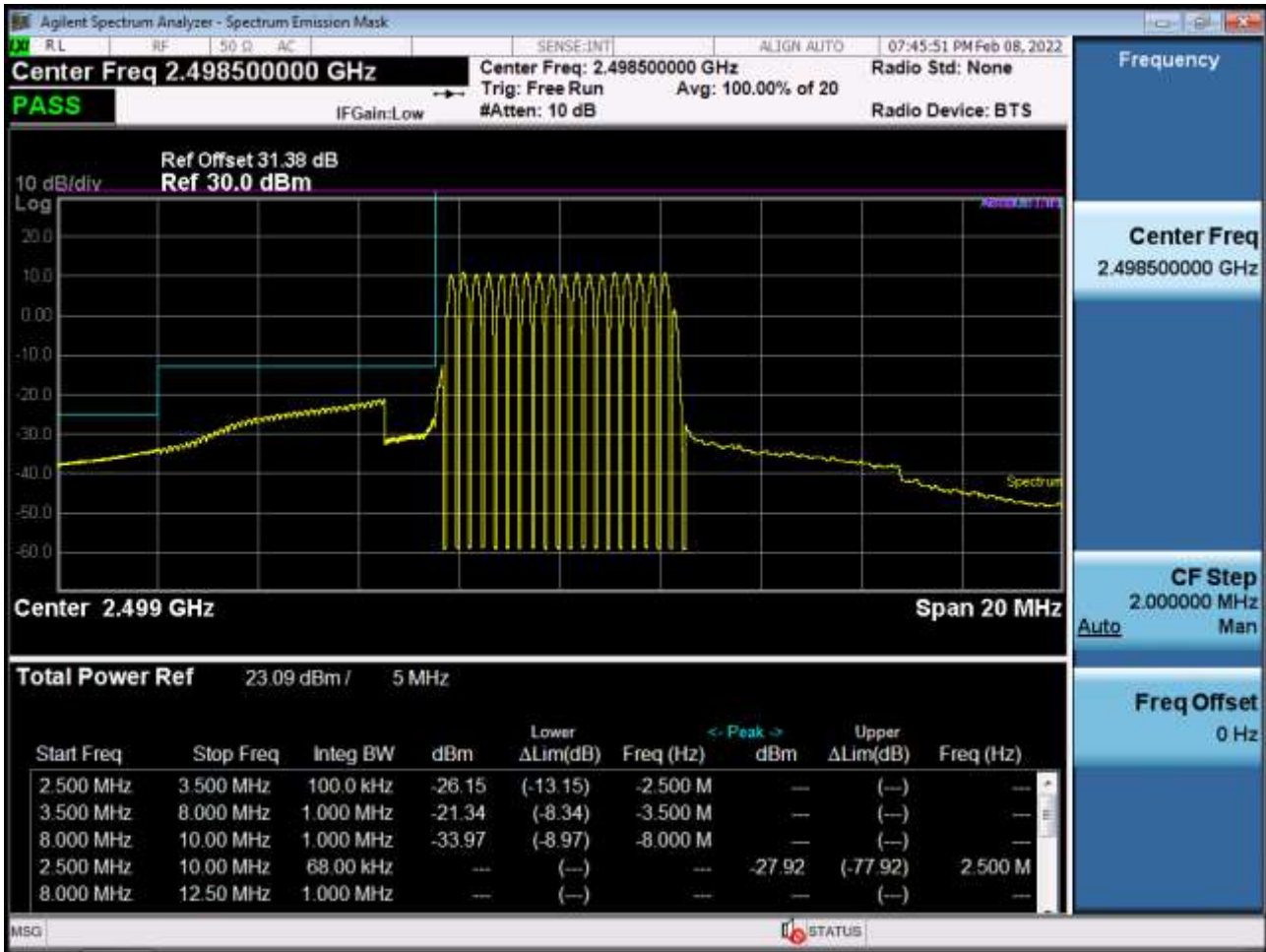
Low Channel Edge Plot (5 MHz Ch.39675 QPSK_RB25_Offset 0)-1
