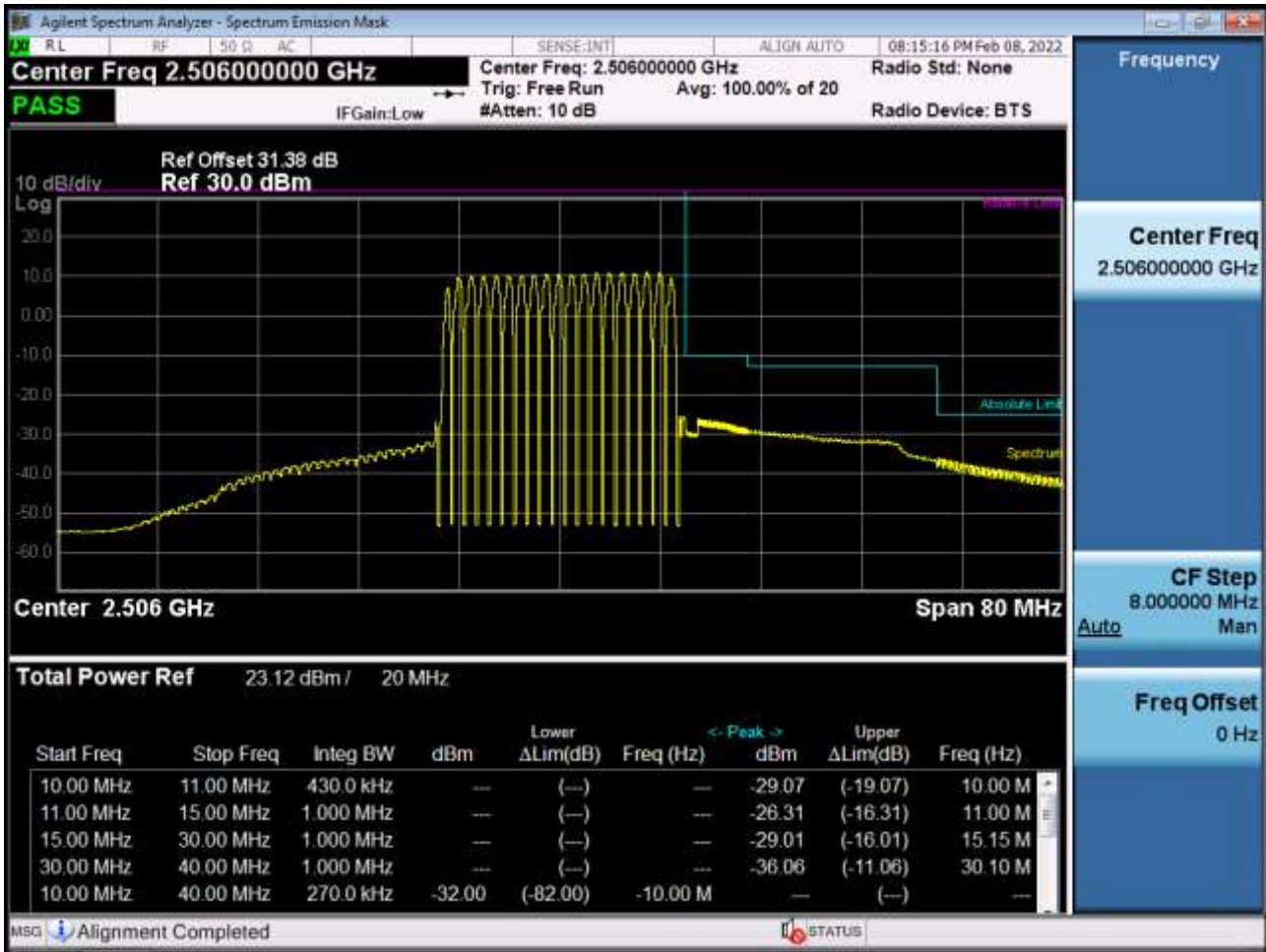
Low Channel Edge Plot (20 MHz Ch.39750 QPSK_RB100_Offset 0)-2
