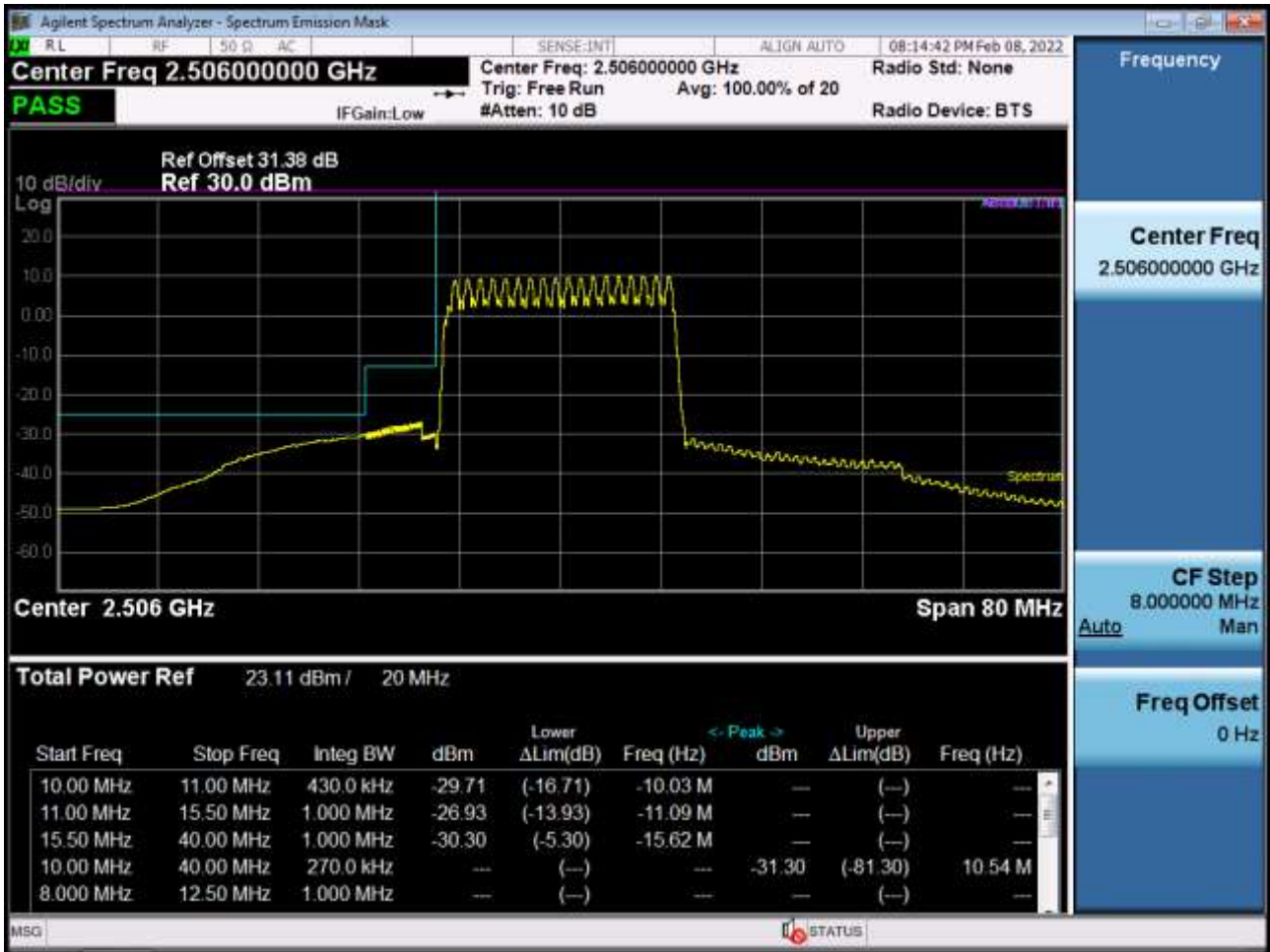
Low Channel Edge Plot (20 MHz Ch.39750 QPSK_RB100_Offset 0)-1
