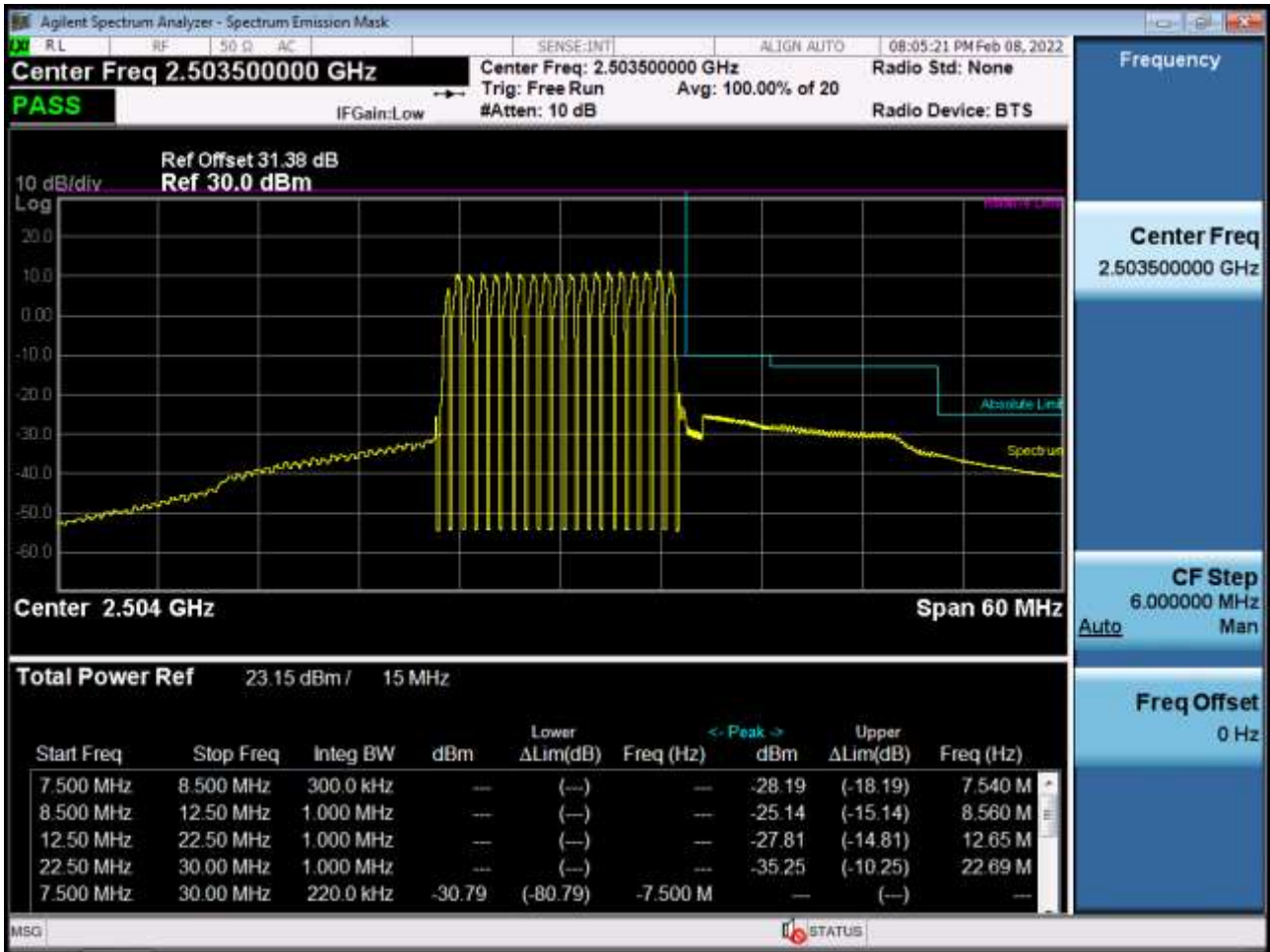
Low Channel Edge Plot (15 MHz Ch.39725 QPSK_RB75_Offset 0)-2
