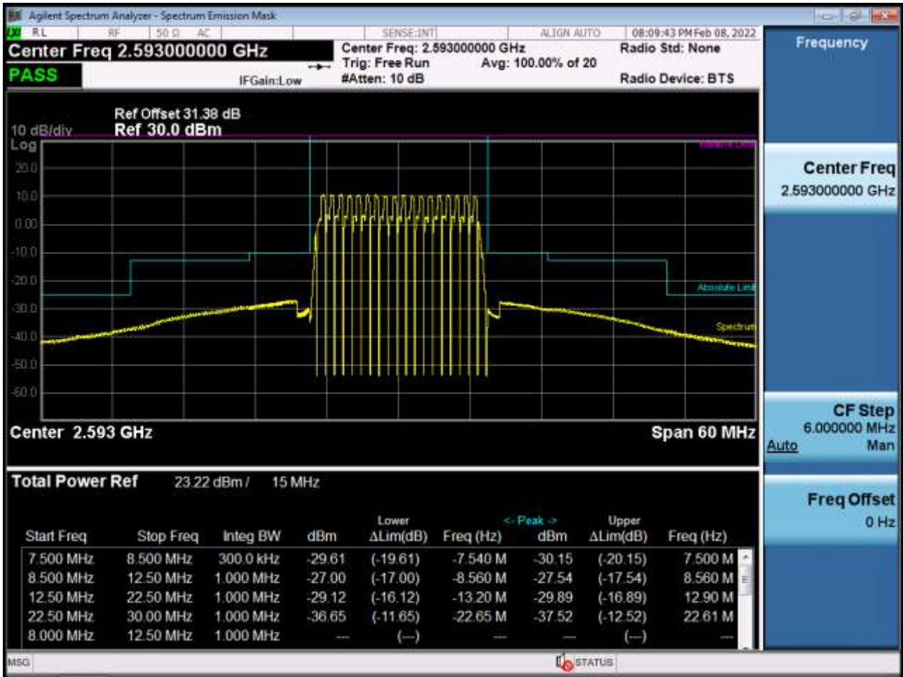
Mid Channel Edge Plot (15 MHz Ch.40620 QPSK RB 75)
