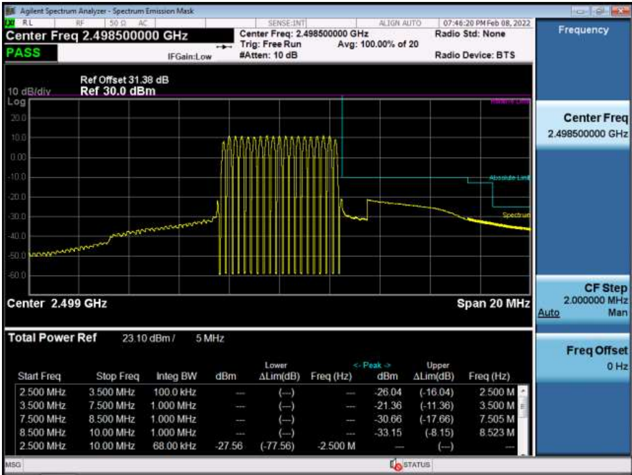
Low Channel Edge Plot (5 MHz Ch.39675 QPSK_RB25_Offset 0)-2
