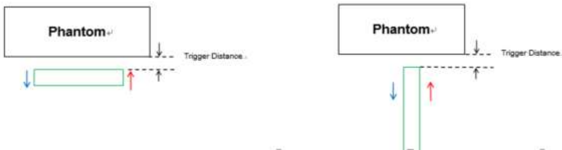
Proximity Sensor Trigger Distance Assessment KDB 616217 D04$6.2 (Rear /Bottom side)
