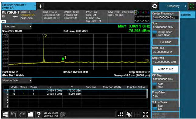
BAND 41. Conducted Spurious Plot 1 (20 MHz Ch.39750 QPSK RB 1, Offset 0)
