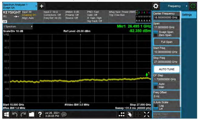
BAND 41. Conducted Spurious Plot 2 (20 MHz Ch. 40620 QPSK RB 1, Offset 0)
