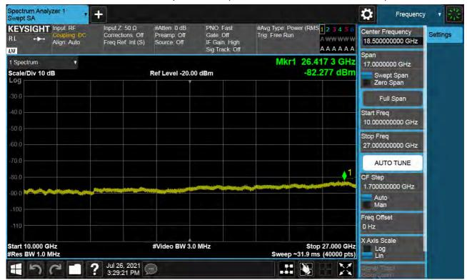
BAND 41. Conducted Spurious Plot 2 (20 MHz Ch. 41490 QPSK RB 1, Offset 0)
