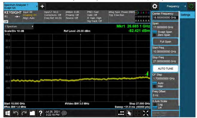
BAND 41. Conducted Spurious Plot 2 (20 MHz Ch. 39750 QPSK RB 1, Offset 0)
