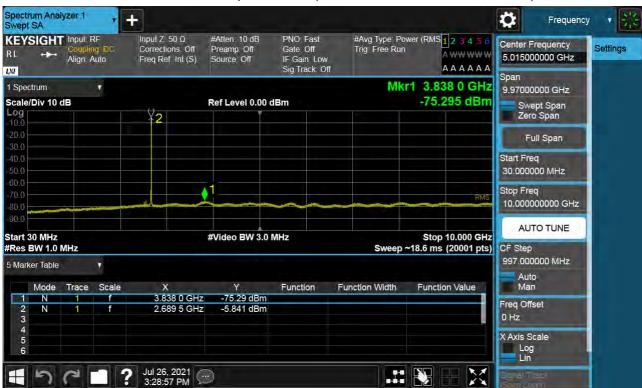
BAND 41. Conducted Spurious Plot 1 (20 MHz Ch.41490 QPSK RB 1, Offset 0)
