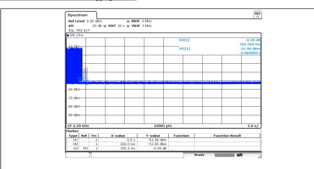
Channel move time = 0.762500 sClosing time =  $0.000625 \text{ s} \times 9 = 0.005625 \text{ s}$
