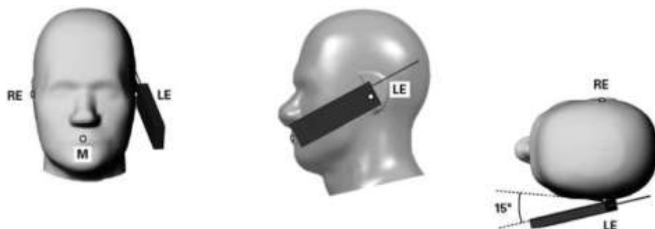
Figure 8.5. Tilt 15° position of the wireless device
