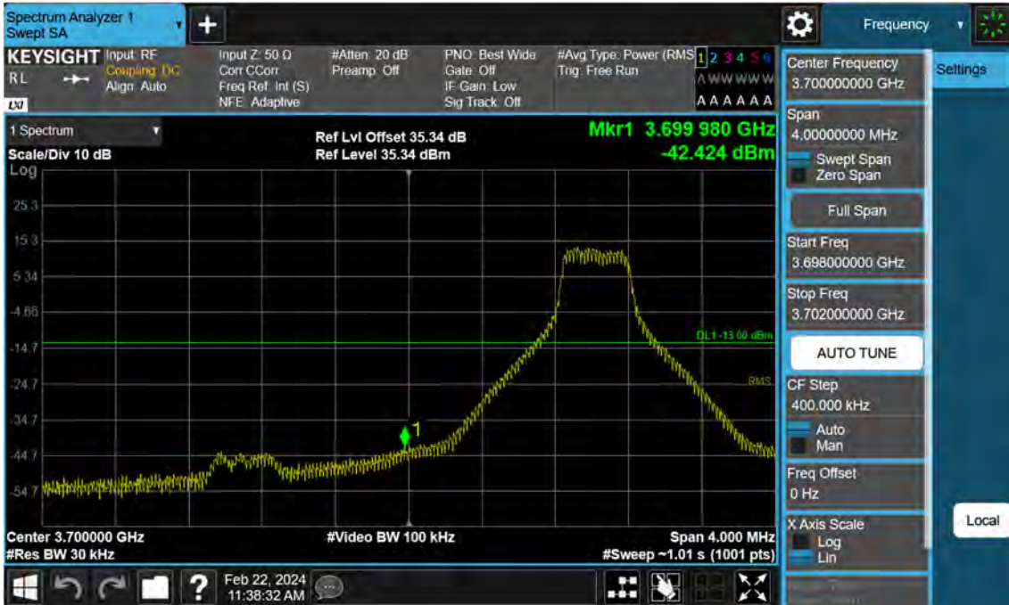
Sub6 n77. Low Band Edge Plot (60 M BW Ch.648668 BPSK 1RB)(1)
