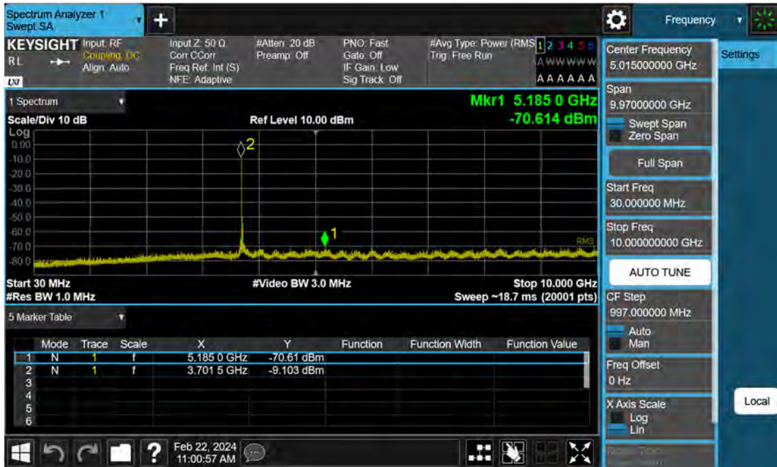
Sub6 n77. Conducted Spurious Plot_1 (647668ch_30 MHz_BPSK)
