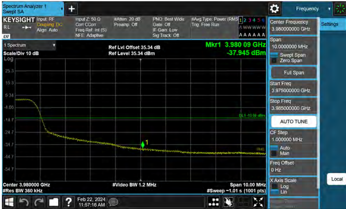
Sub6 n77. High Band Edge Plot (70 M BW Ch.663000 BPSK FullRB)(1)
