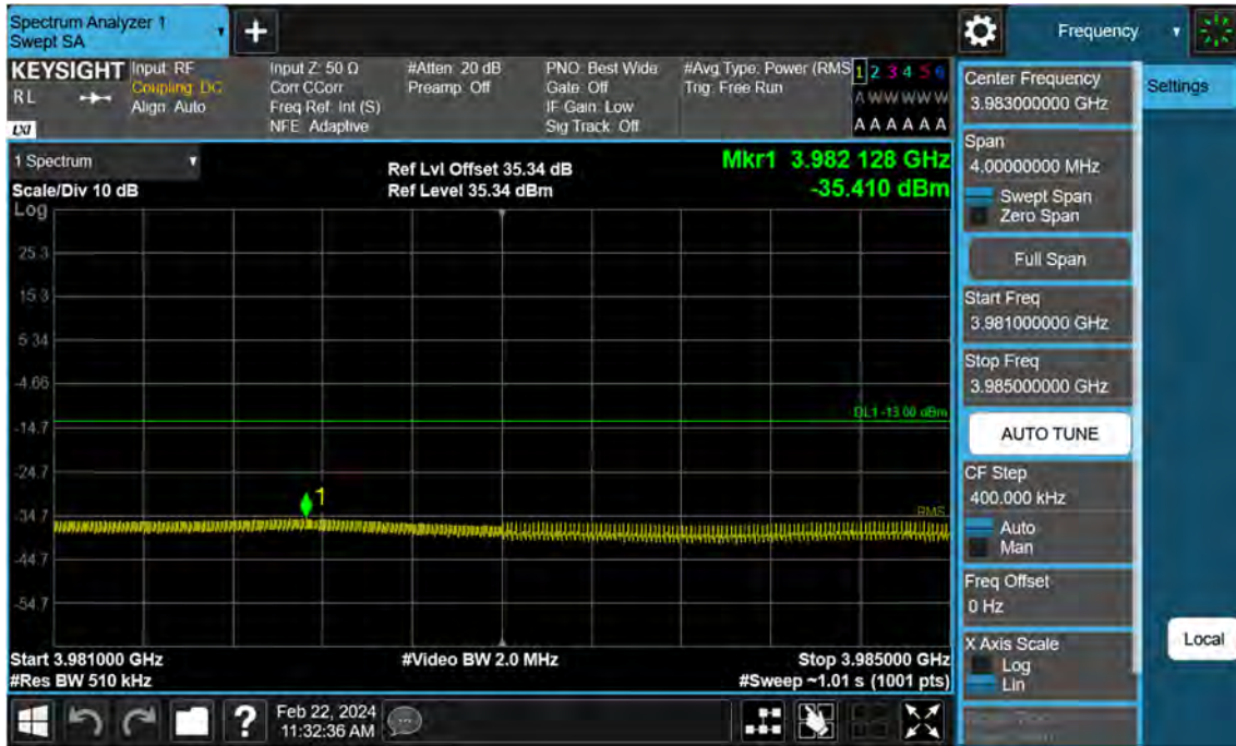
Sub6 n77. High Band Edge Plot (50 M BW Ch.663666 BPSK FullRB)(2)
