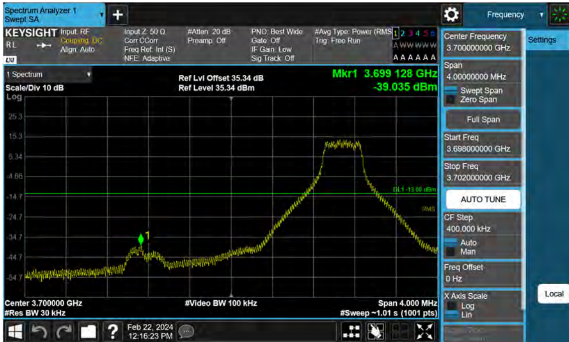
Sub6 n77. Low Band Edge Plot (90 M BW Ch.649668 BPSK 1RB)(1)
