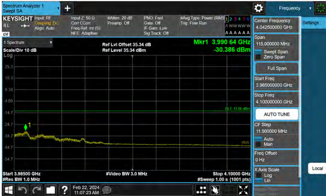
Sub6 n77. High Band Edge Plot (30 M BW Ch.664332 BPSK FullRB)(3)
