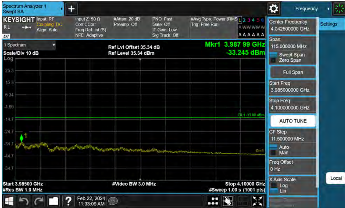
Sub6 n77. High Band Edge Plot (50 M BW Ch.663666 BPSK FullRB)(3)
