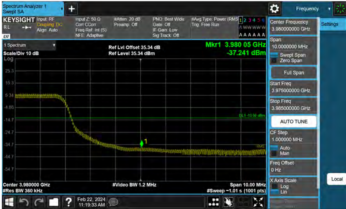
Sub6 n77. High Band Edge Plot (40 M BW Ch.664000 BPSK FullRB)(1)
