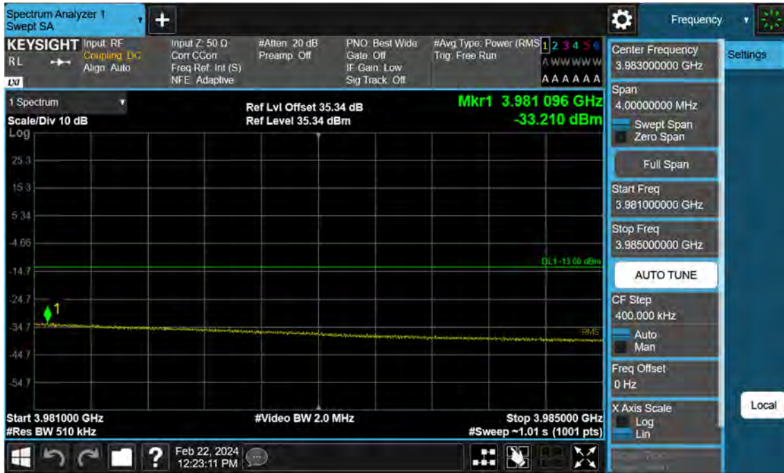
Sub6 n77. High Band Edge Plot (90 M BW Ch.662332 BPSK FullRB)(2)
