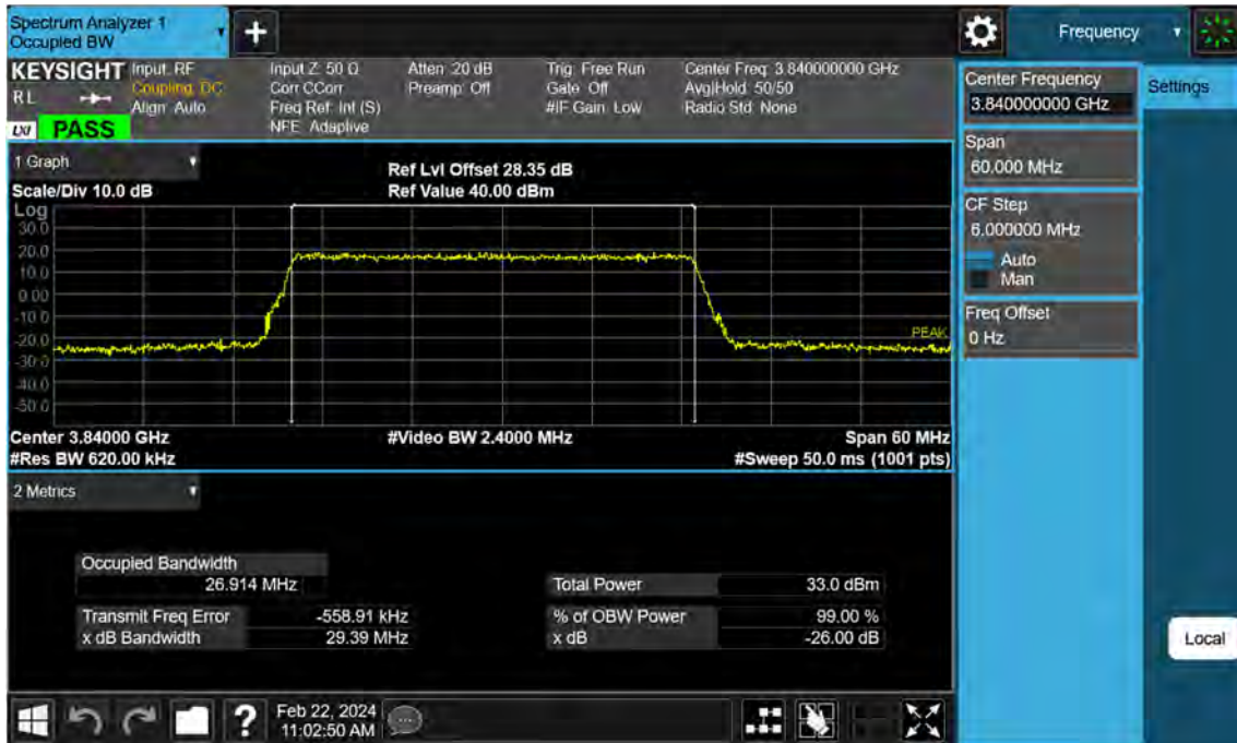
Sub6 n77. Occupied Bandwidth Plot (30 M BW Ch.656000 QPSK )
