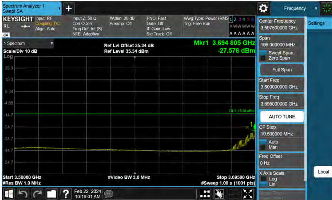
Sub6 n77. Low Band Edge Plot (15 M BW Ch.647168 BPSK FullRB)(3)
