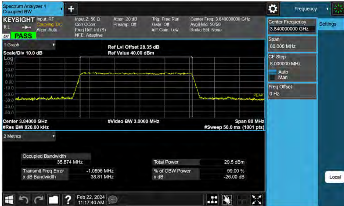
Sub6 n77. Occupied Bandwidth Plot (40 M BW Ch.656000 256QAM )
