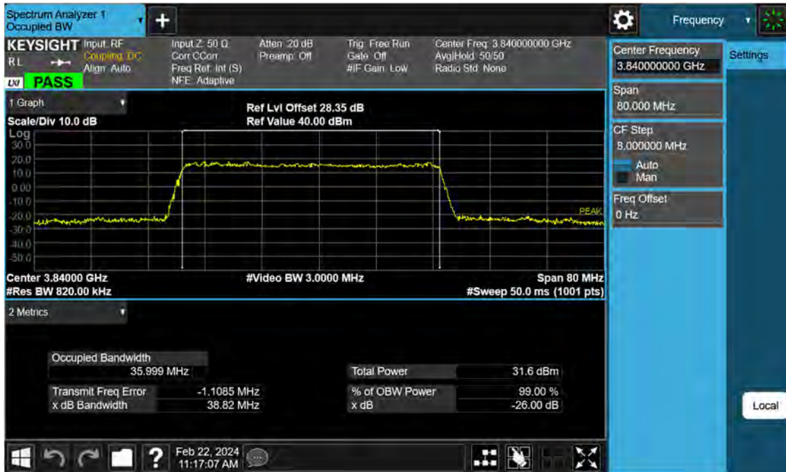
Sub6 n77. Occupied Bandwidth Plot (40 M BW Ch.656000 64QAM)
