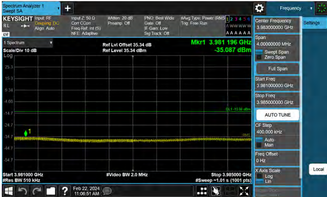
Sub6 n77. High Band Edge Plot (30 M BW Ch.664332 BPSK FullRB)(2)
