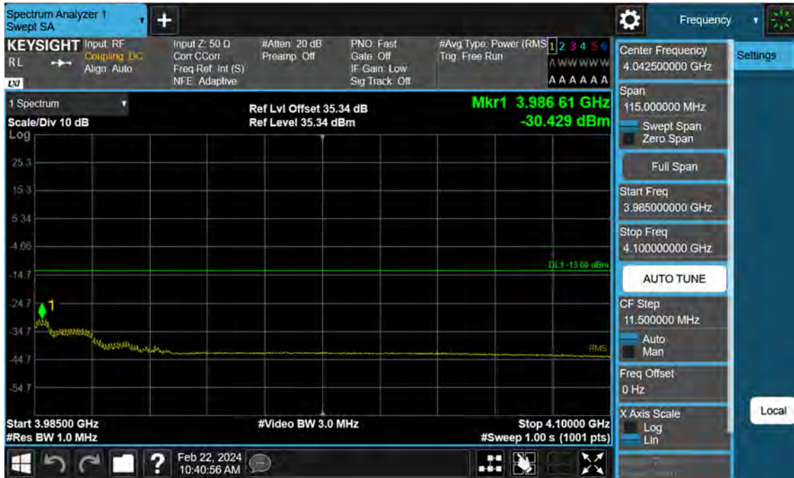
Sub6 n77. High Band Edge Plot (20 M BW Ch.664666 BPSK FullRB)(3)
