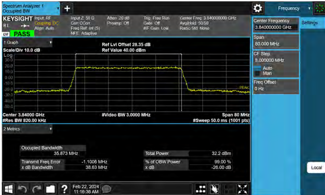
Sub6 n77. Occupied Bandwidth Plot (40 M BW Ch.656000 16QAM)
