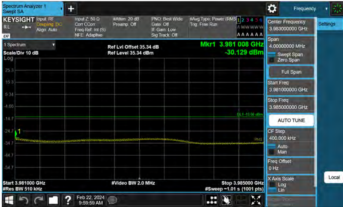
Sub6 n77. High Band Edge Plot (10 M BW Ch.665000 BPSK FullRB)(2)
