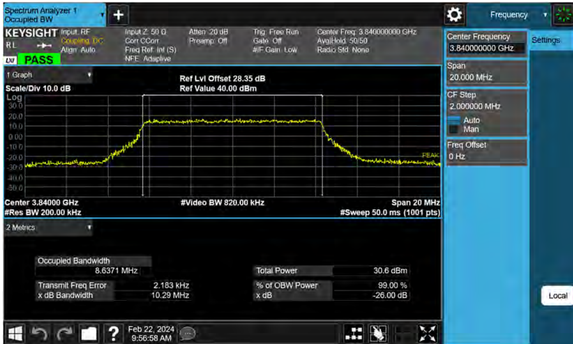
Sub6 n77. Occupied Bandwidth Plot (10 M BW Ch.656000 64QAM)
