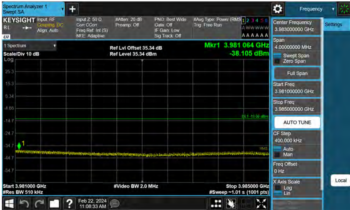
Sub6 n77. High Band Edge Plot (30 M BW Ch.664332 BPSK 1RB)(2)
