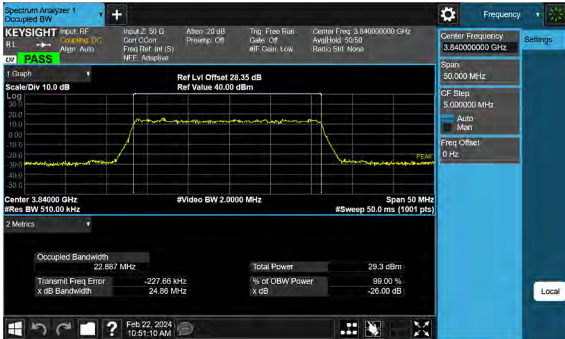
Sub6 n77. Occupied Bandwidth Plot (25 M BW Ch.656000 256QAM)
