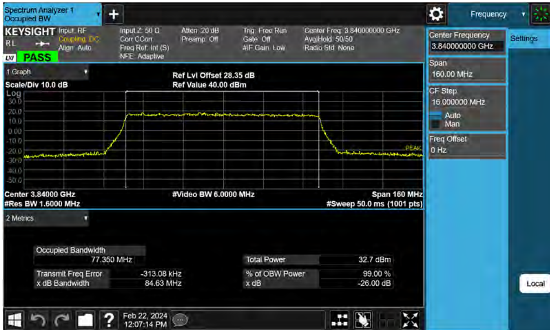
Sub6 n77. Occupied Bandwidth Plot (80 M BW Ch.656000 16QAM)
