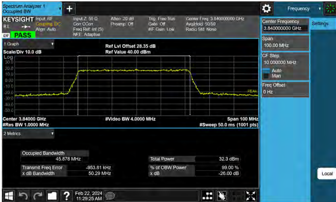
Sub6 n77. Occupied Bandwidth Plot (50 M BW Ch.656000 16QAM)
