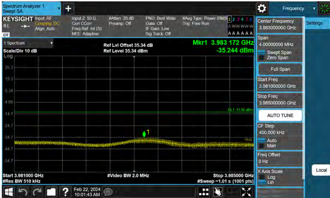
Sub6 n77. High Band Edge Plot (10 M BW Ch.665000 BPSK 1RB)(2)
