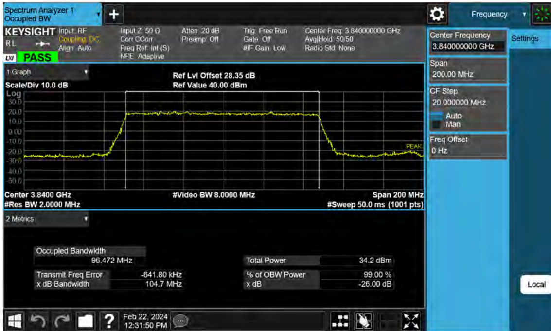
Sub6 n77. Occupied Bandwidth Plot (100 M BW Ch.656000 BPSK)
