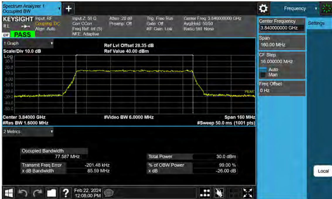
Sub6 n77. Occupied Bandwidth Plot (80 M BW Ch.656000 256QAM )
