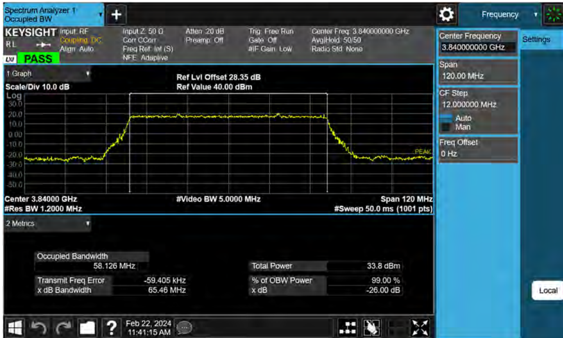
Sub6 n77. Occupied Bandwidth Plot (60 M BW Ch.656000 BPSK )
