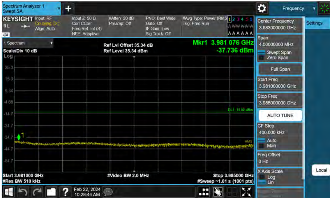
Sub6 n77. High Band Edge Plot (15 M BW Ch.664832 BPSK 1RB)(2)
