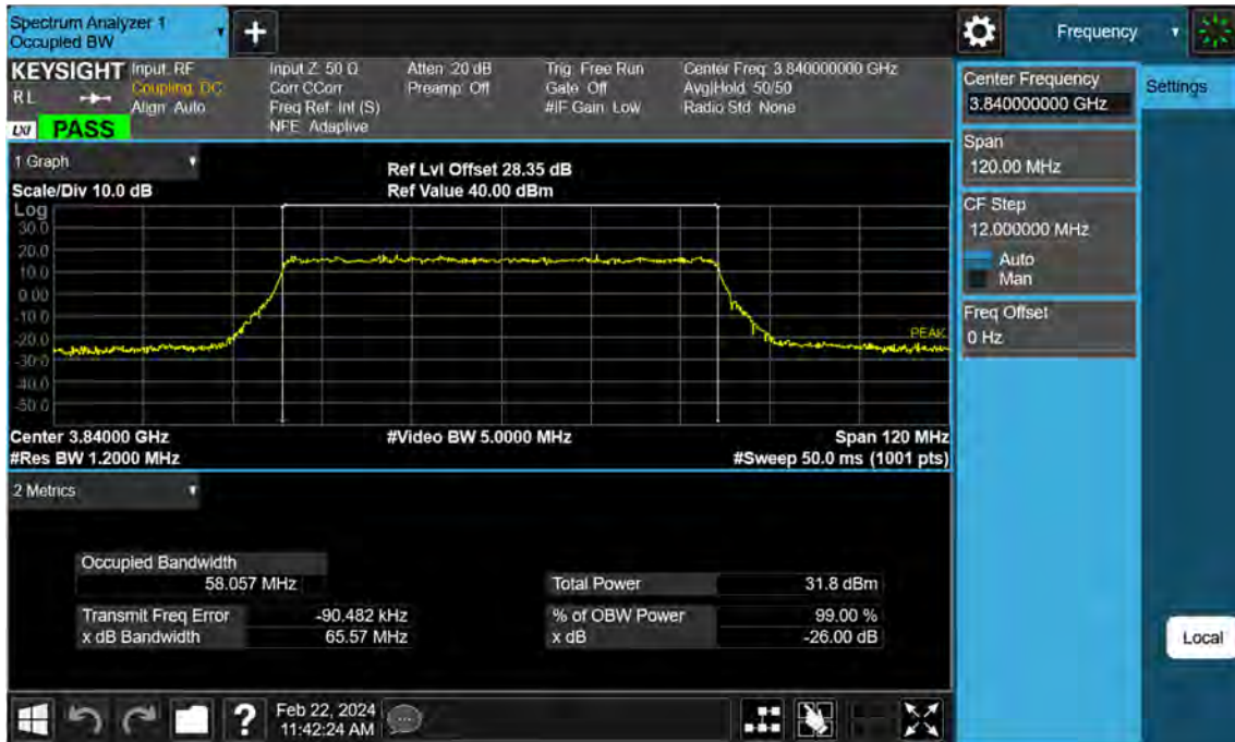
Sub6 n77. Occupied Bandwidth Plot (60 M BW Ch.656000 64QAM)
