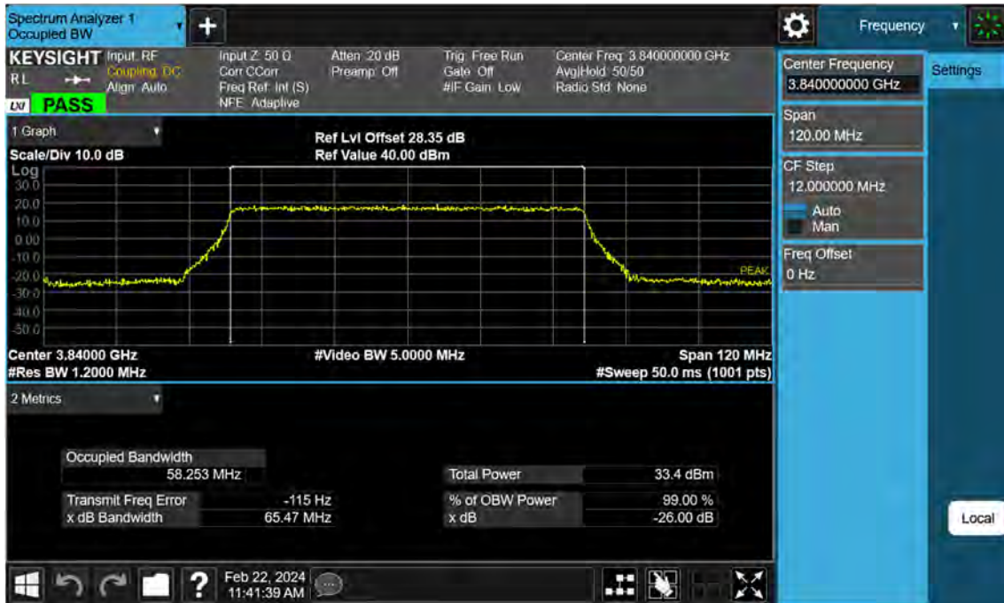
Sub6 n77. Occupied Bandwidth Plot (60 M BW Ch.656000 QPSK )
