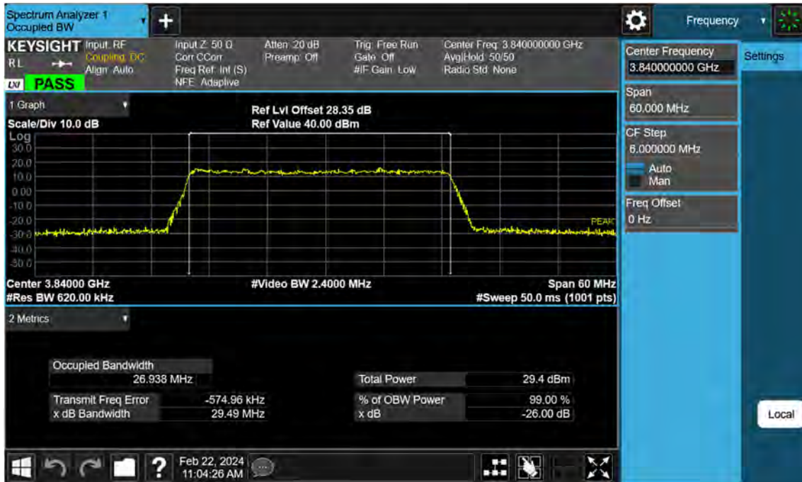
Sub6 n77. Occupied Bandwidth Plot (30 M BW Ch.656000 256QAM)
