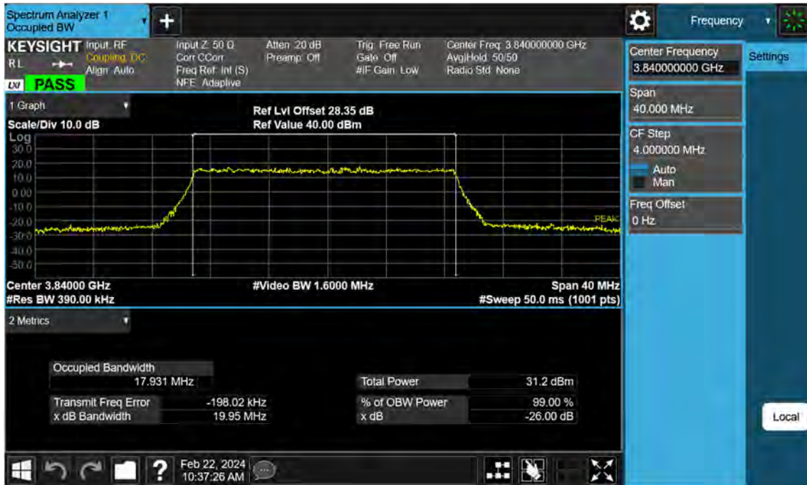
Sub6 n77. Occupied Bandwidth Plot (20 M BW Ch.656000 64QAM)
