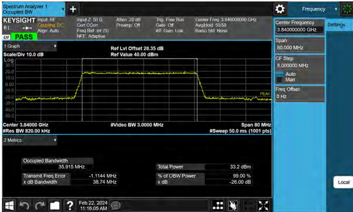
Sub6 n77. Occupied Bandwidth Plot (40 M BW Ch.656000 QPSK )
