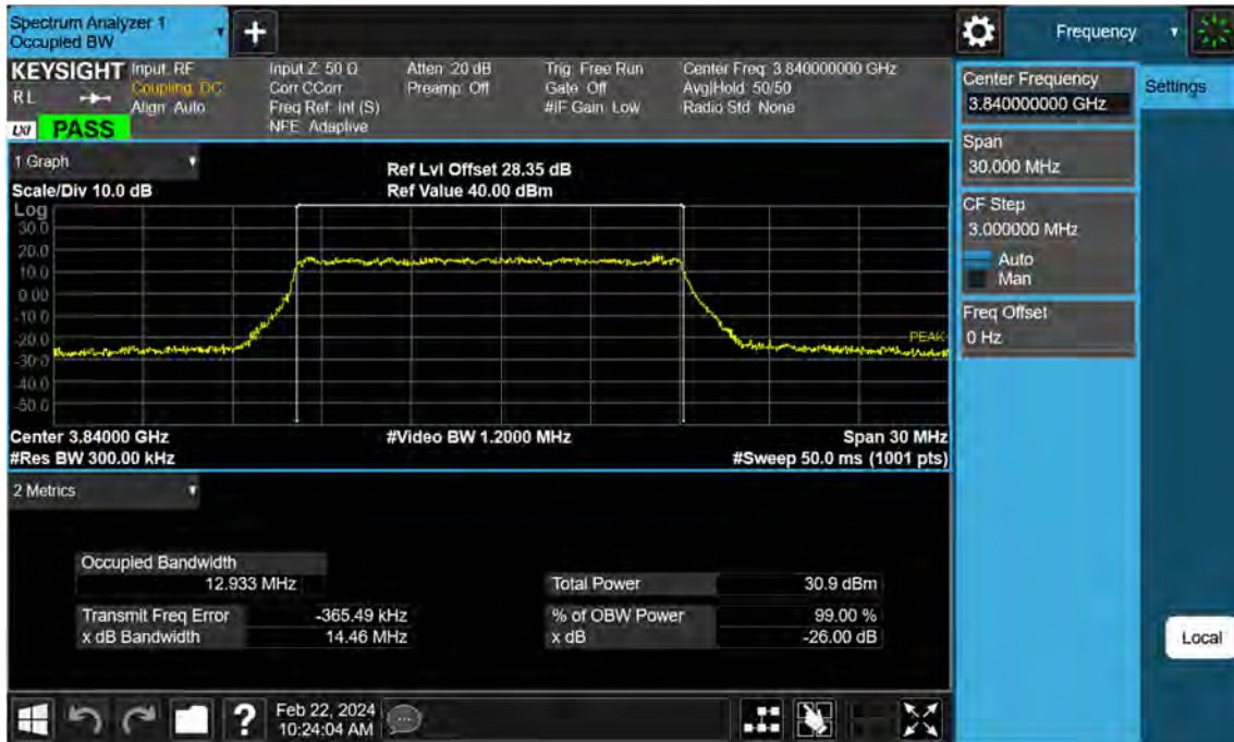
Sub6 n77. Occupied Bandwidth Plot (15 M BW Ch.656000 64QAM)
