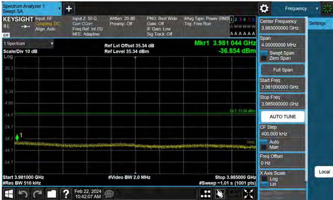
Sub6 n77. High Band Edge Plot (20 M BW Ch.664666 BPSK 1RB)(2)
