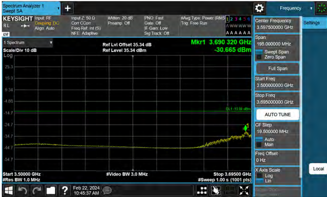
Sub6 n77. Low Band Edge Plot (25 M BW Ch.647500 BPSK FullRB)(3)
