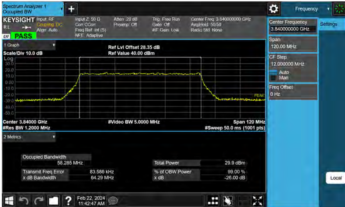
Sub6 n77. Occupied Bandwidth Plot (60 M BW Ch.656000 256QAM )
