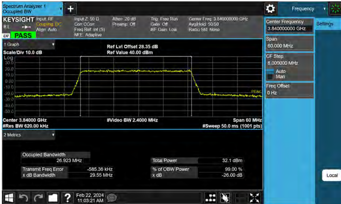
Sub6 n77. Occupied Bandwidth Plot (30 M BW Ch.656000 16QAM)
