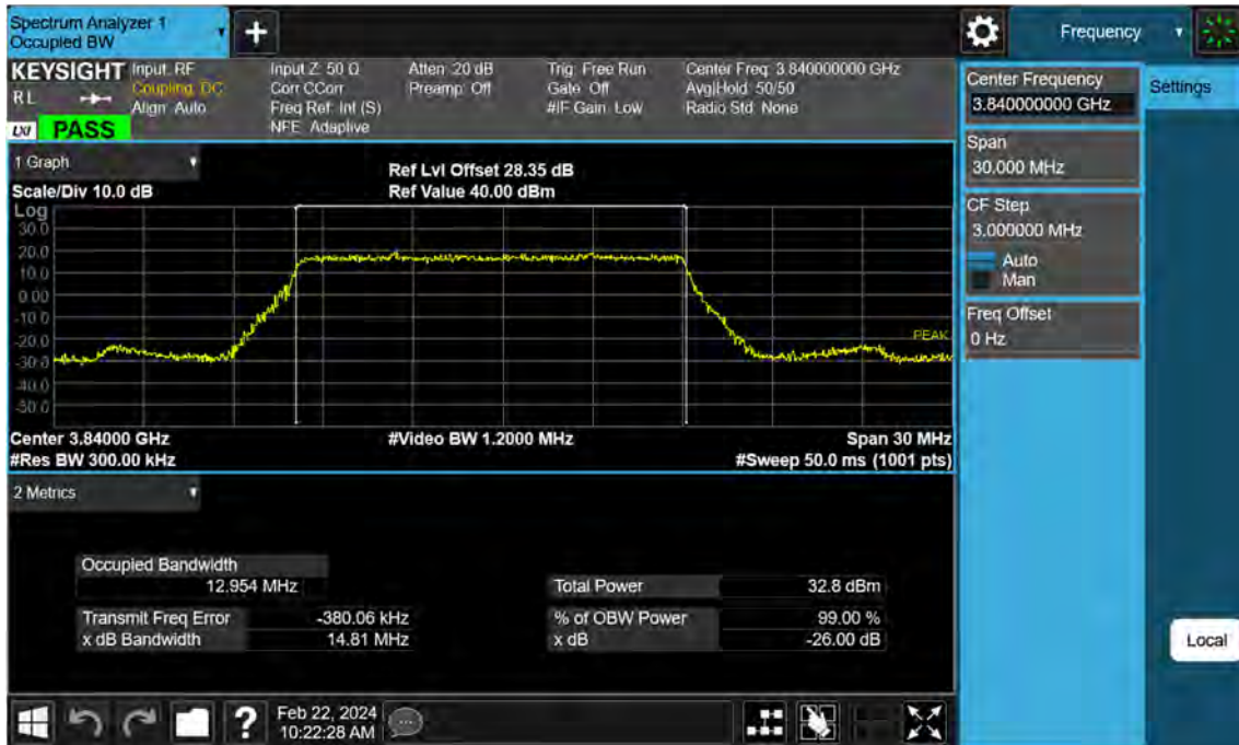
Sub6 n77. Occupied Bandwidth Plot (15 M BW Ch.656000 BPSK )
