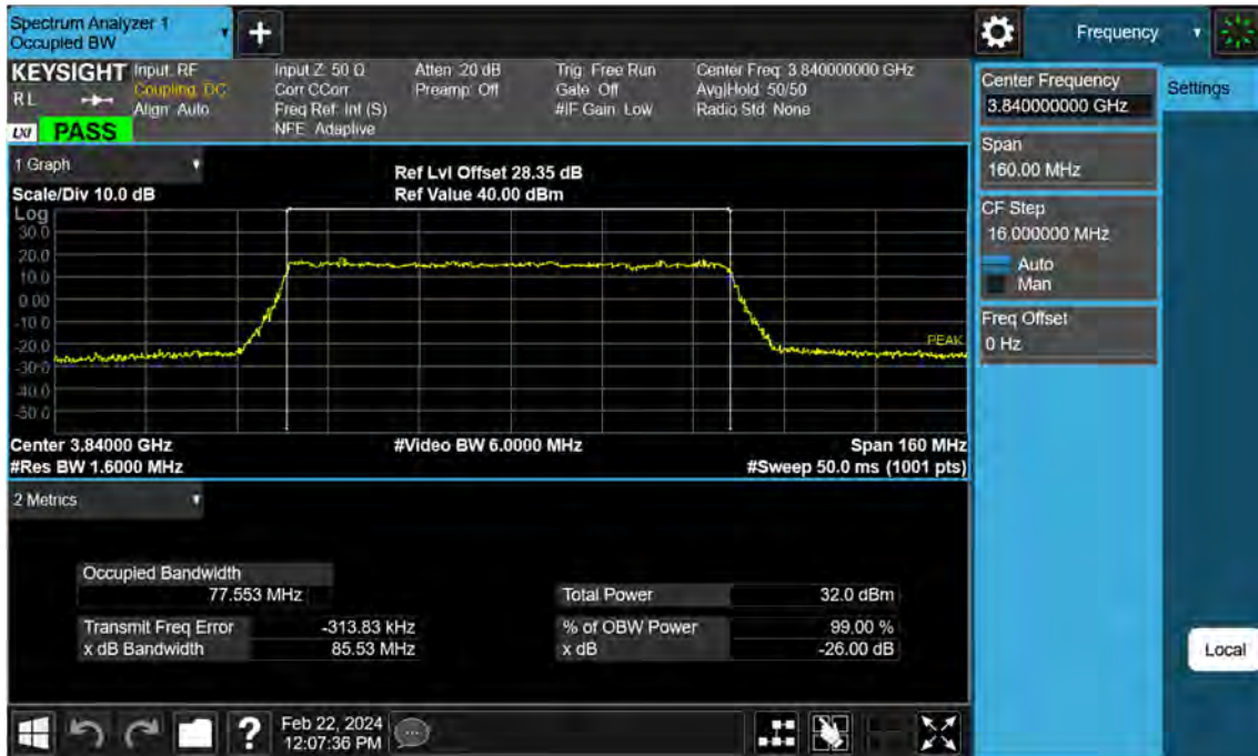
Sub6 n77. Occupied Bandwidth Plot (80 M BW Ch.656000 64QAM)
