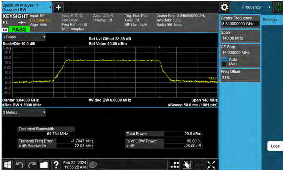
Sub6 n77. Occupied Bandwidth Plot (70 M BW Ch.656000 256QAM )
