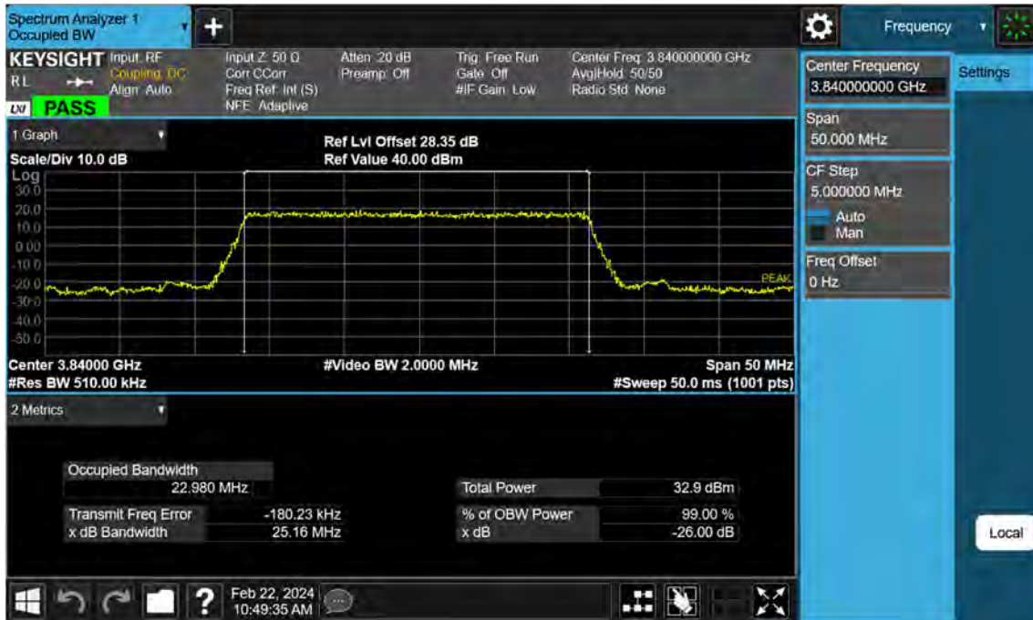
Sub6 n77. Occupied Bandwidth Plot (25 M BW Ch.656000 QPSK )
