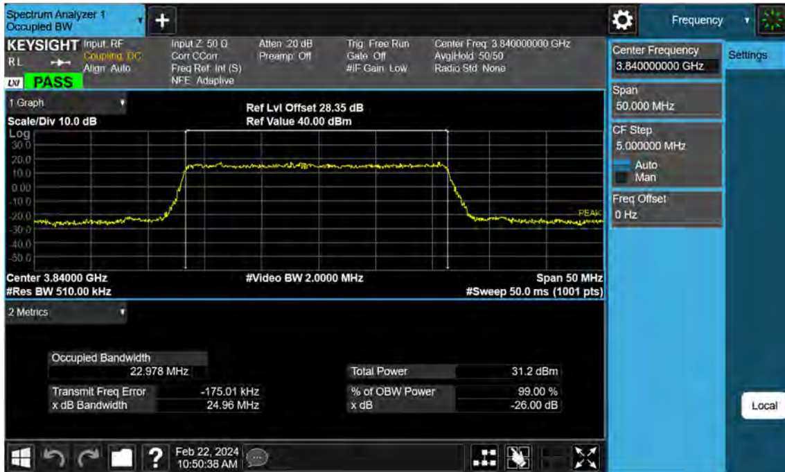
Sub6 n77. Occupied Bandwidth Plot (25 M BW Ch.656000 64QAM)
