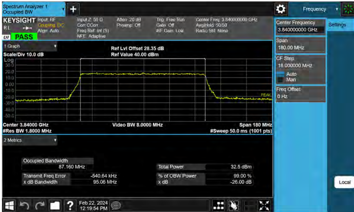
Sub6 n77. Occupied Bandwidth Plot (90 M BW Ch.656000 16QAM)
