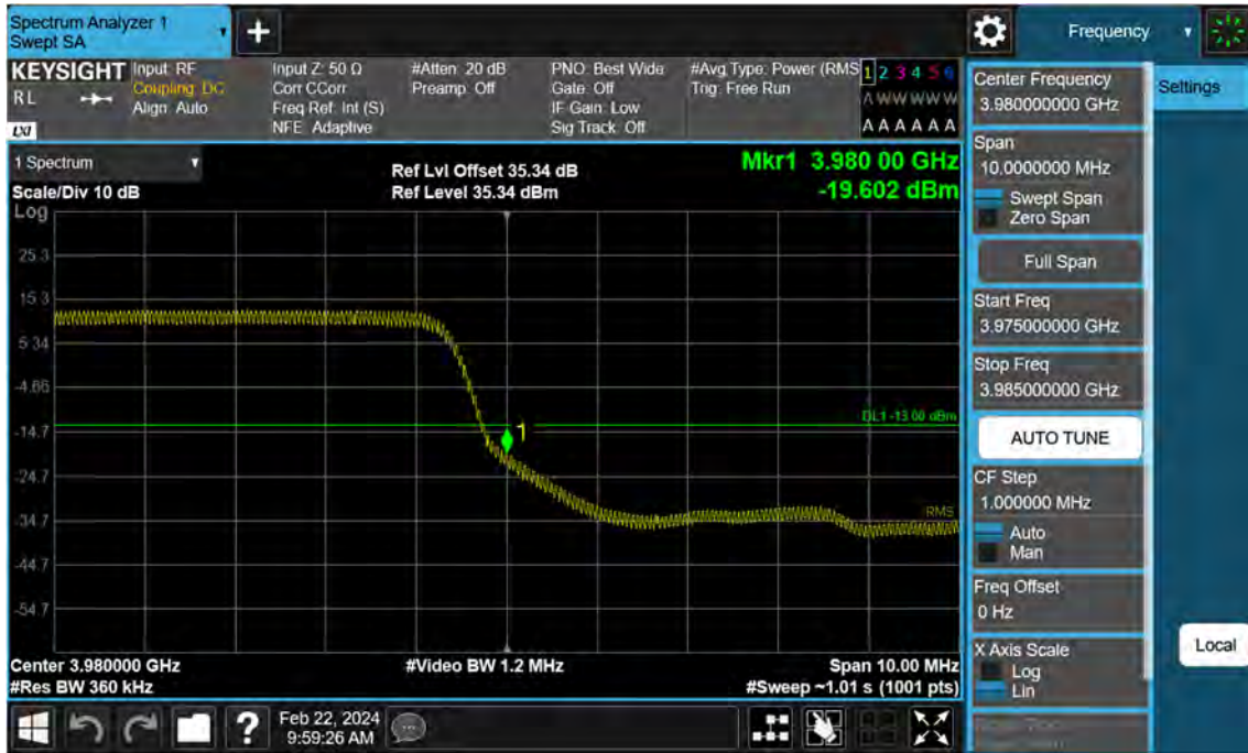
Sub6 n77. High Band Edge Plot (10 M BW Ch.665000 BPSK FullRB)(1)
