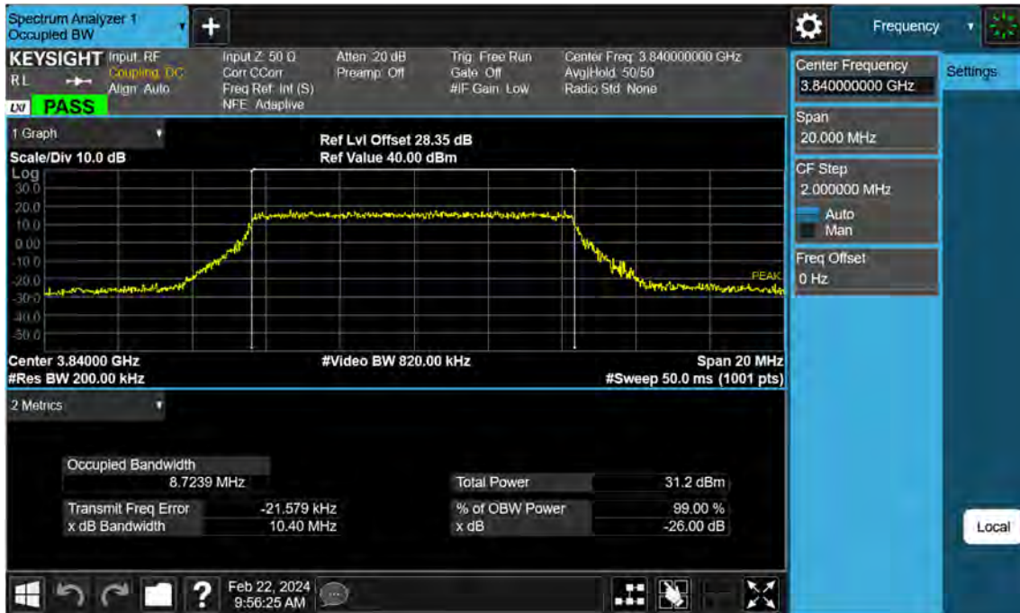
Sub6 n77. Occupied Bandwidth Plot (10 M BW Ch.656000 16QAM)
