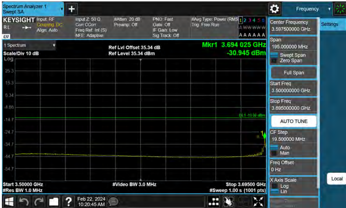
Sub6 n77. Low Band Edge Plot (15 M BW Ch.647168 BPSK 1RB)(3)
