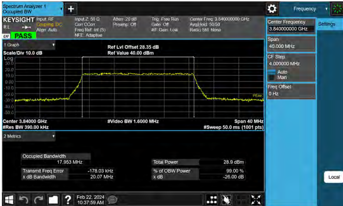
Sub6 n77. Occupied Bandwidth Plot (20 M BW Ch.656000 256QAM)
