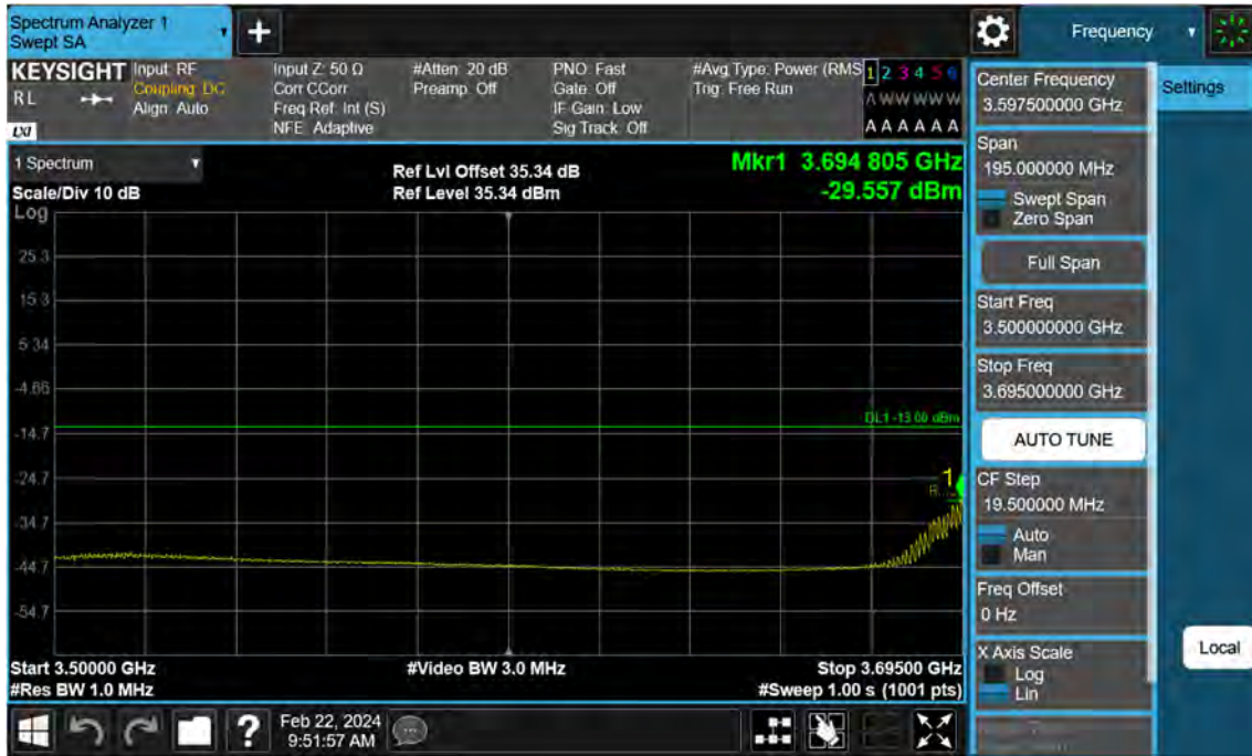
Sub6 n77. Low Band Edge Plot (10 M BW Ch.647000 BPSK FullRB)(3)
