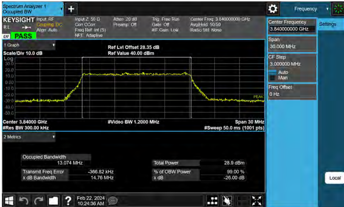
Sub6 n77. Occupied Bandwidth Plot (15 M BW Ch.656000 256QAM)
