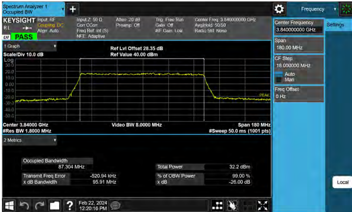
Sub6 n77. Occupied Bandwidth Plot (90 M BW Ch.656000 64QAM)
