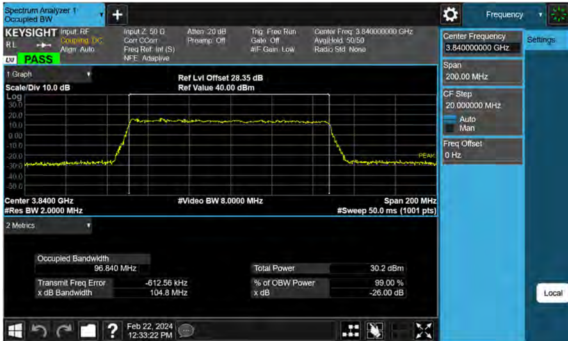
Sub6 n77. Occupied Bandwidth Plot (100 M BW Ch.656000 256QAM)
