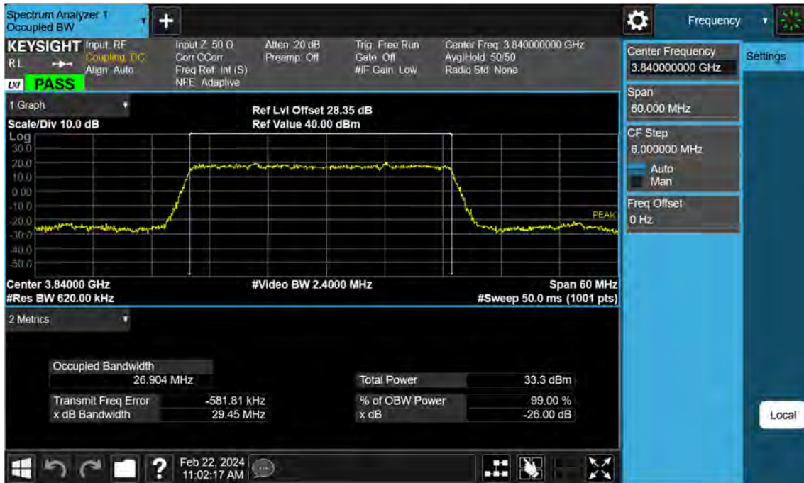
Sub6 n77. Occupied Bandwidth Plot (30 M BW Ch.656000 BPSK )
