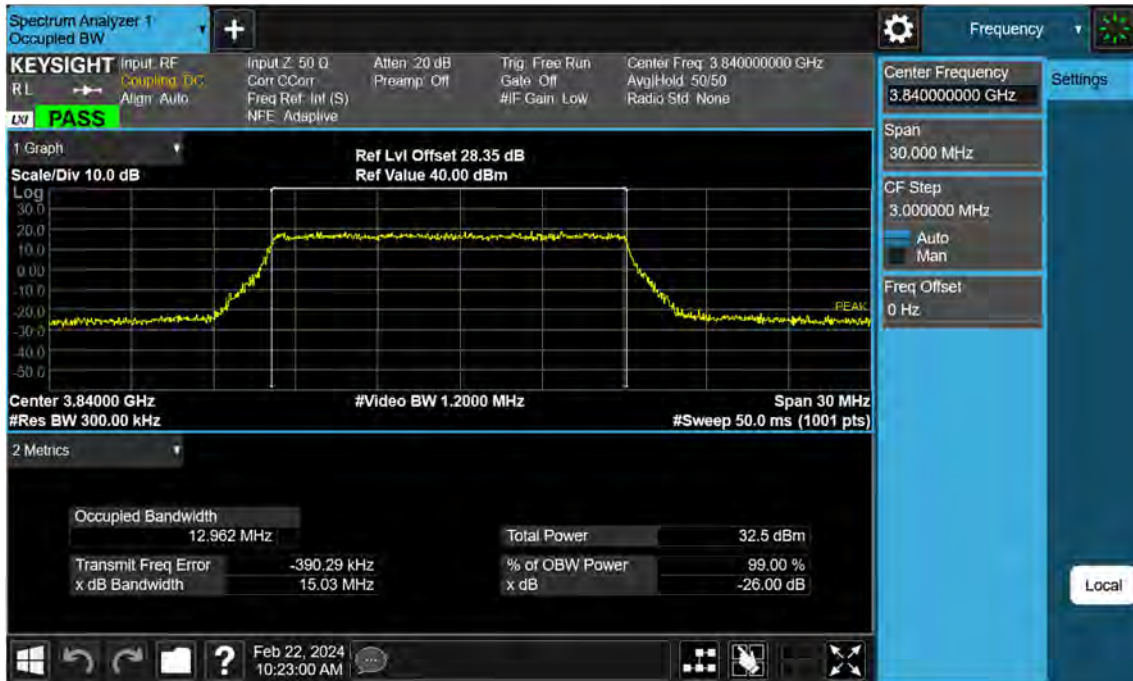
Sub6 n77. Occupied Bandwidth Plot (15 M BW Ch.656000 QPSK )
