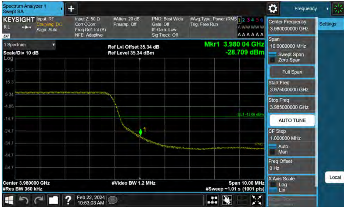
Sub6 n77. High Band Edge Plot (25 M BW Ch.664500 BPSK FullRB)(1)
