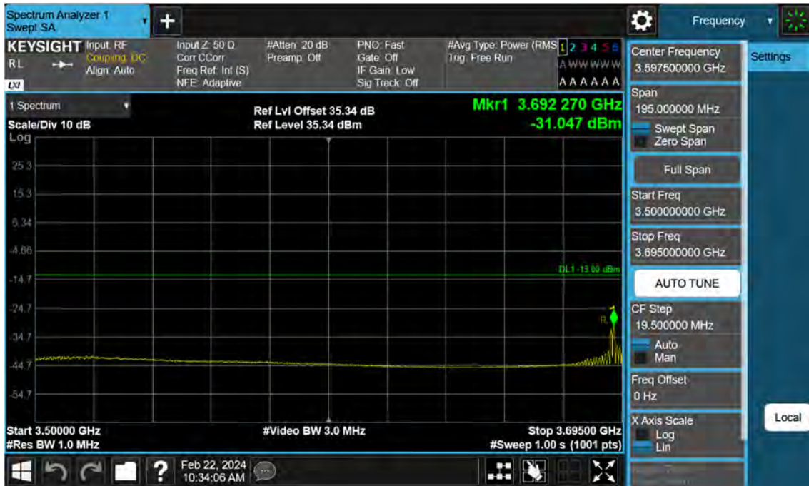
Sub6 n77. Low Band Edge Plot (20 M BW Ch.647334 BPSK 1RB)(3)
