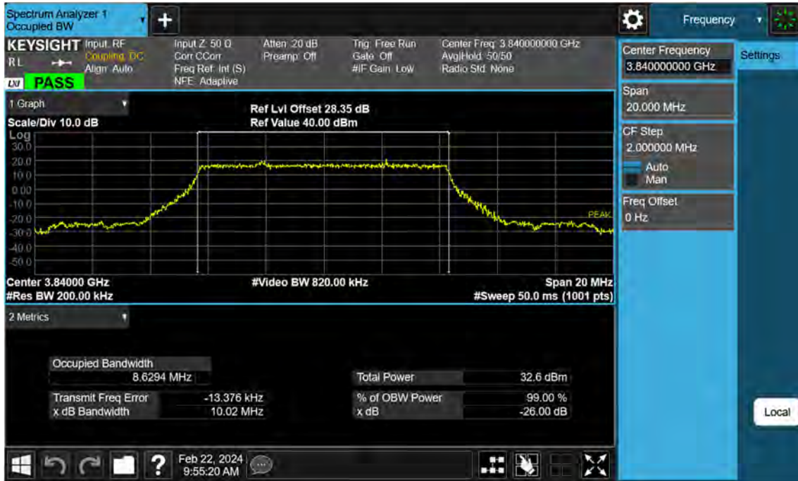
Sub6 n77. Occupied Bandwidth Plot (10 M BW Ch.656000 BPSK )
