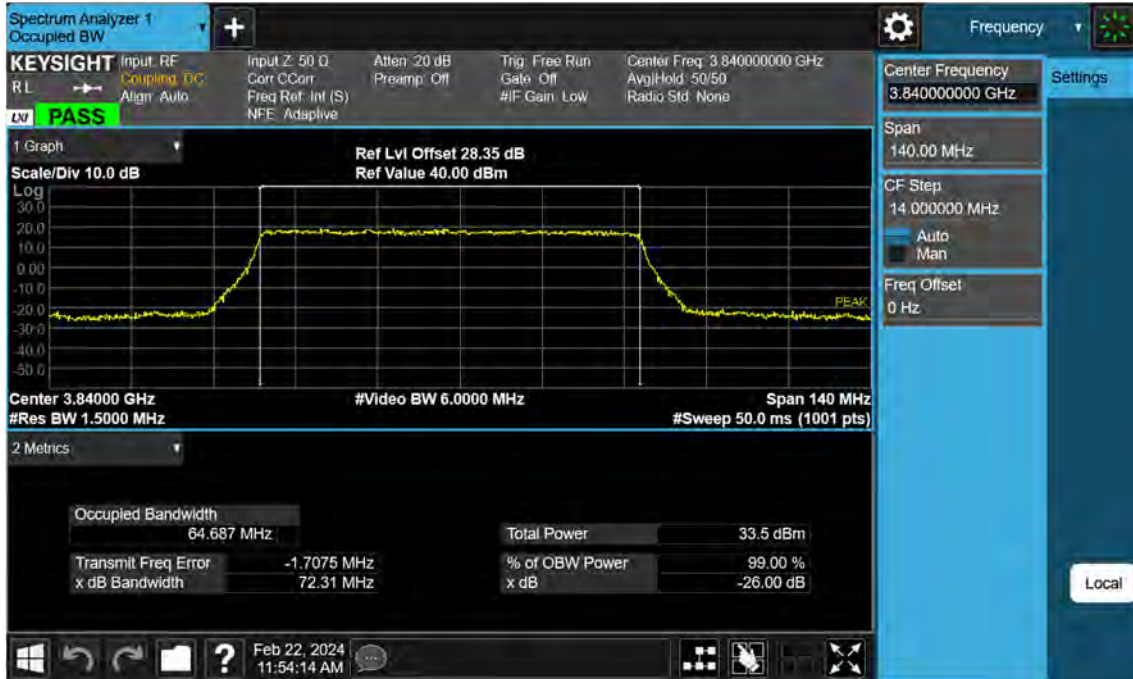
Sub6 n77. Occupied Bandwidth Plot (70 M BW Ch.656000 QPSK )
