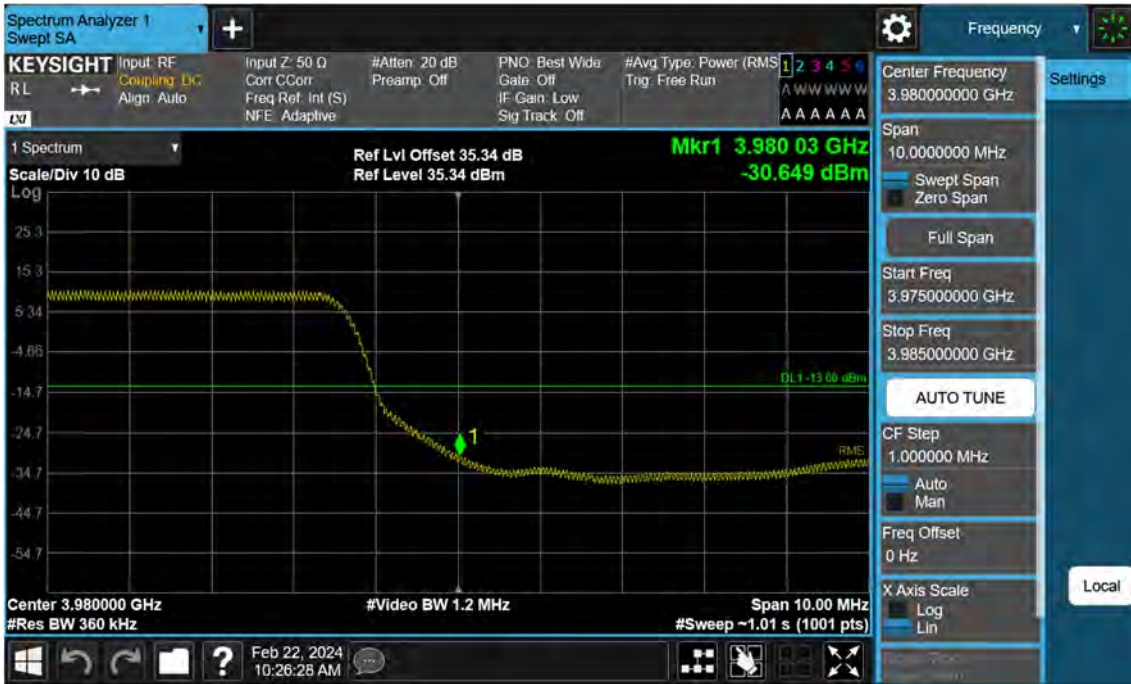
Sub6 n77. High Band Edge Plot (15 M BW Ch.664832 BPSK FullRB)(1)
