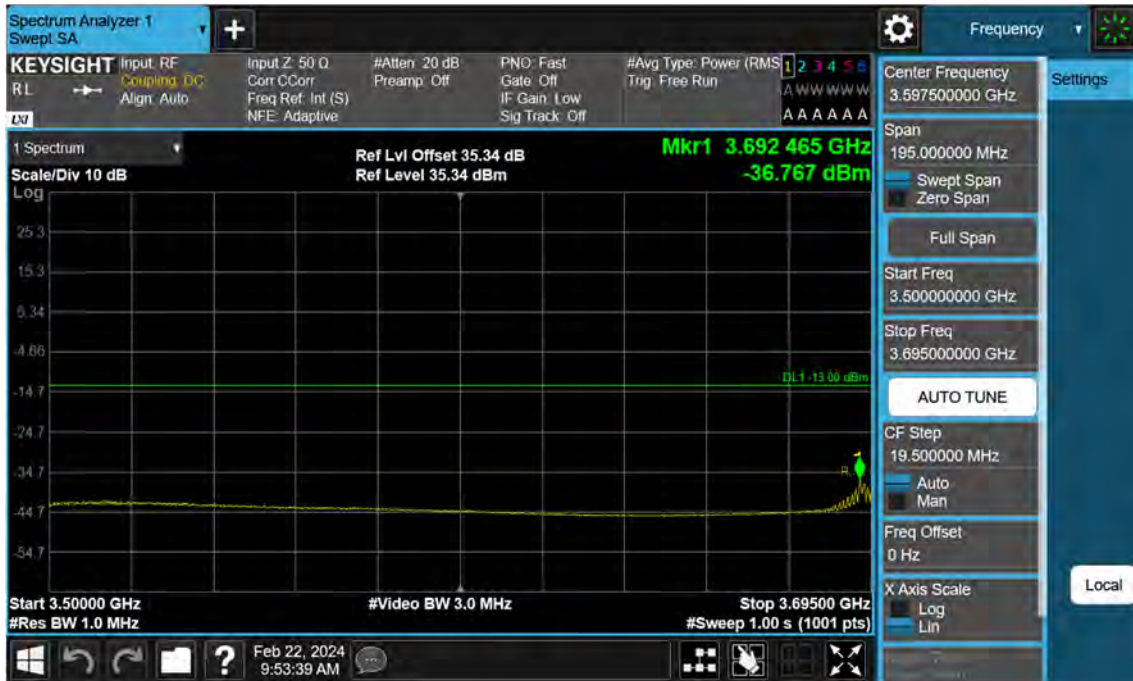
Sub6 n77. Low Band Edge Plot (10 M BW Ch.647000 BPSK 1RB)(3)
