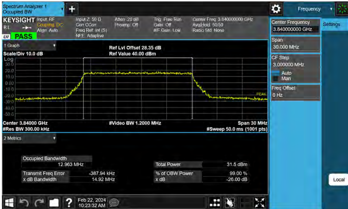
Sub6 n77. Occupied Bandwidth Plot (15 M BW Ch.656000 16QAM)
