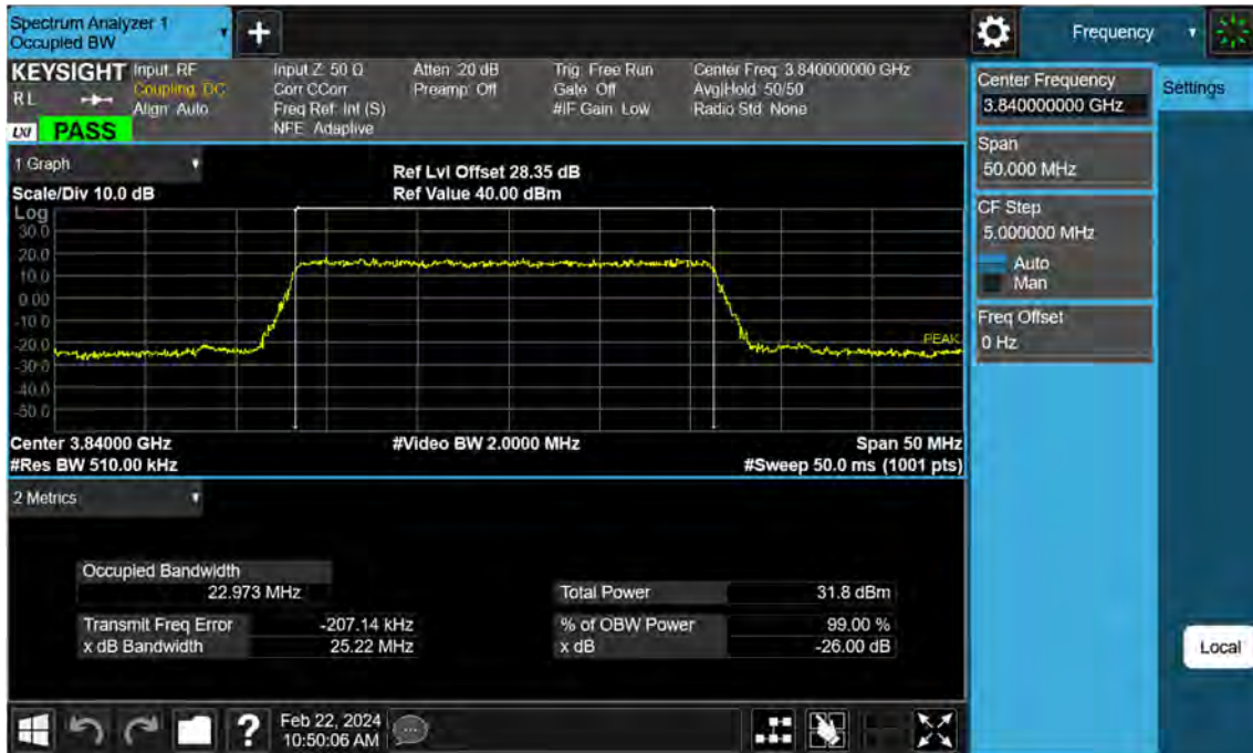
Sub6 n77. Occupied Bandwidth Plot (25 M BW Ch.656000 16QAM)
