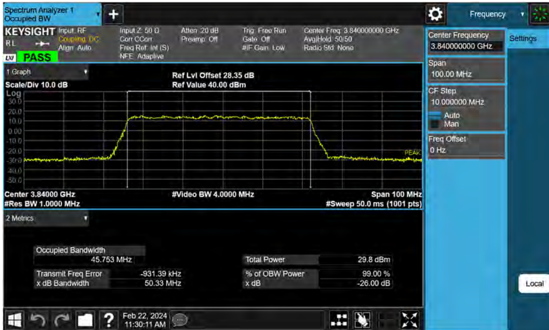
Sub6 n77. Occupied Bandwidth Plot (50 M BW Ch.656000 256QAM )
