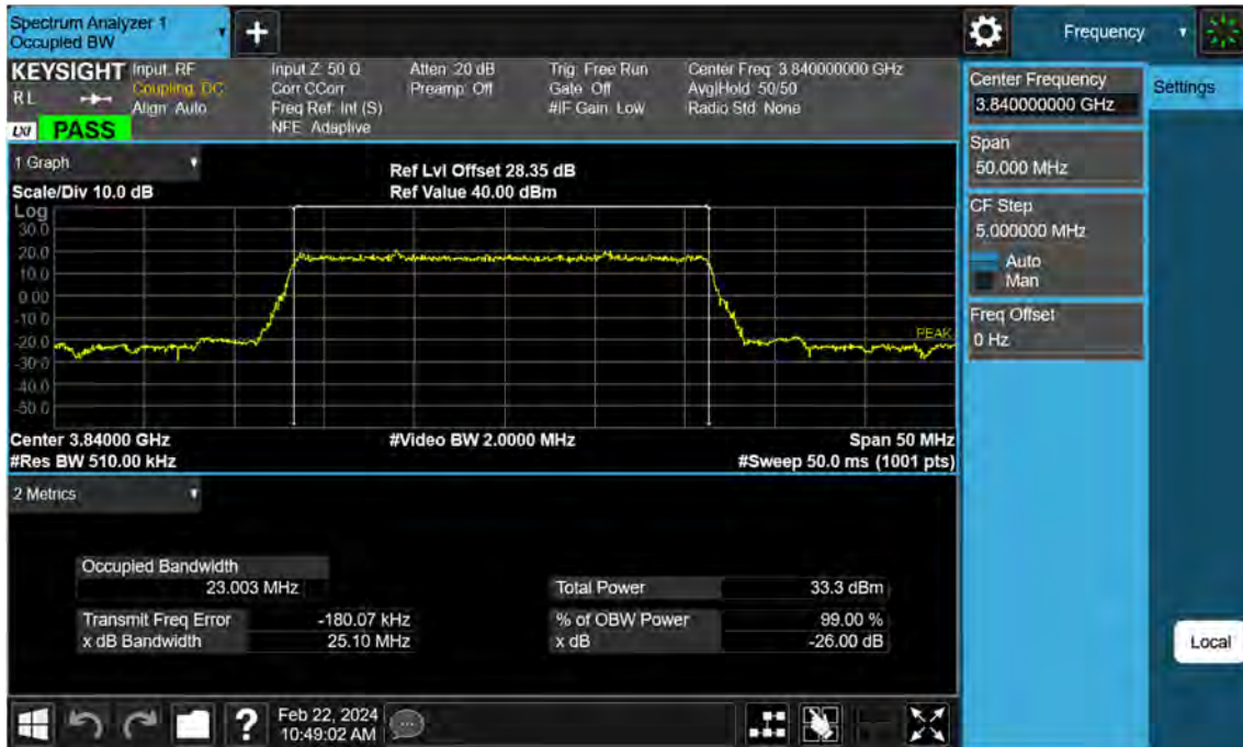
Sub6 n77. Occupied Bandwidth Plot (25 M BW Ch.656000 BPSK )
