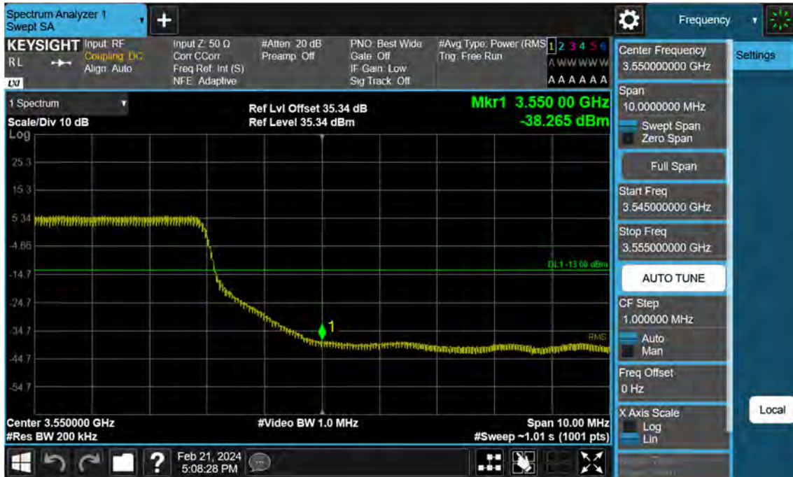
Sub6 n77. High Band Edge Plot (30 M BW Ch.635666 BPSK FullRB)(1)
