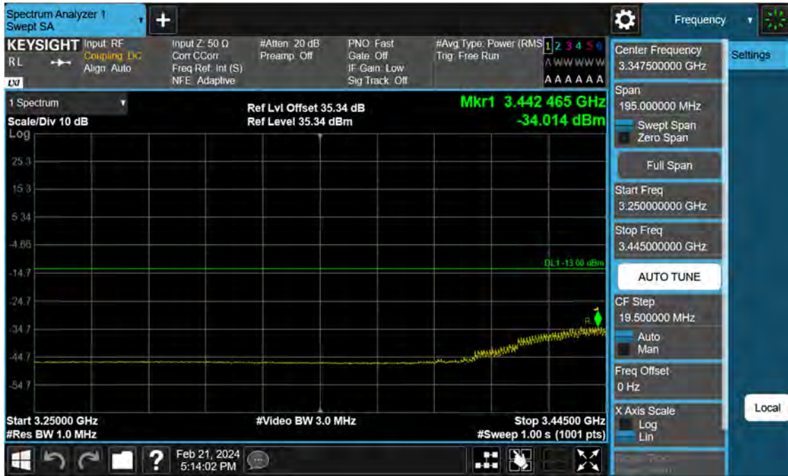
Sub6 n77. Low Band Edge Plot (40 M BW Ch.631334 BPSK FullRB)(3)
