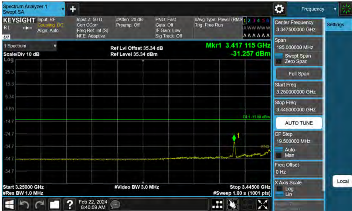
Sub6 n77. Low Band Edge Plot (70 M BW Ch.632334 BPSK 1RB)(3)
