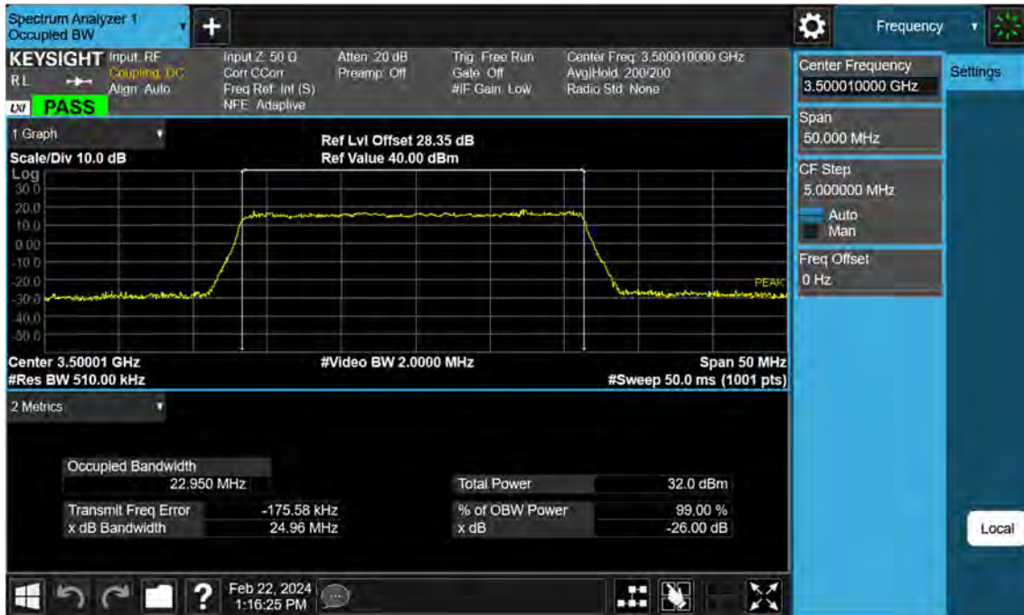
Sub6 n77. Occupied Bandwidth Plot (25 M BW Ch.633334 64QAM)
