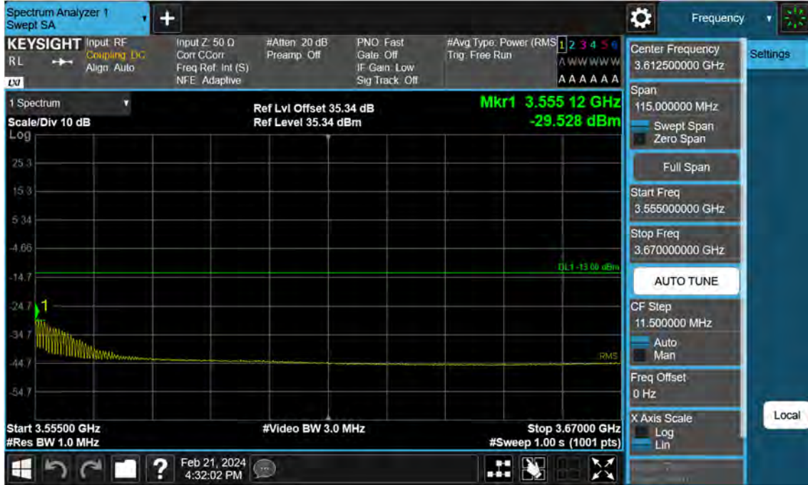
Sub6 n77. High Band Edge Plot (10 M BW Ch.636322 BPSK FullRB)(3)
