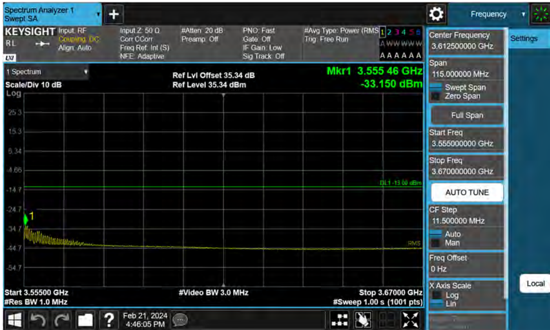
Sub6 n77. High Band Edge Plot (15 M BW Ch.636166 BPSK 1RB)(3)
