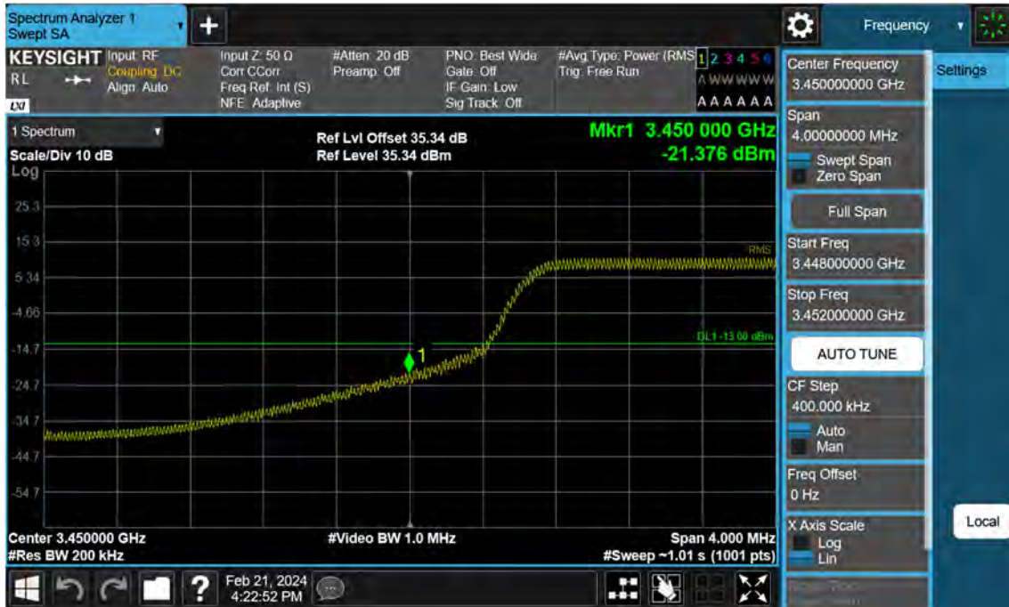
Sub6 n77. Low Band Edge Plot (10 M BW Ch.630334 BPSK FullRB)(1)
