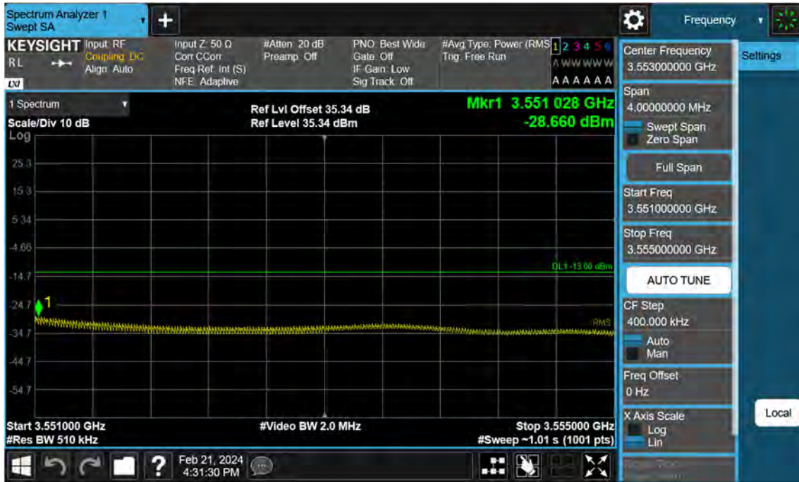
Sub6 n77. High Band Edge Plot (10 M BW Ch.636322 BPSK FullRB)(2)
