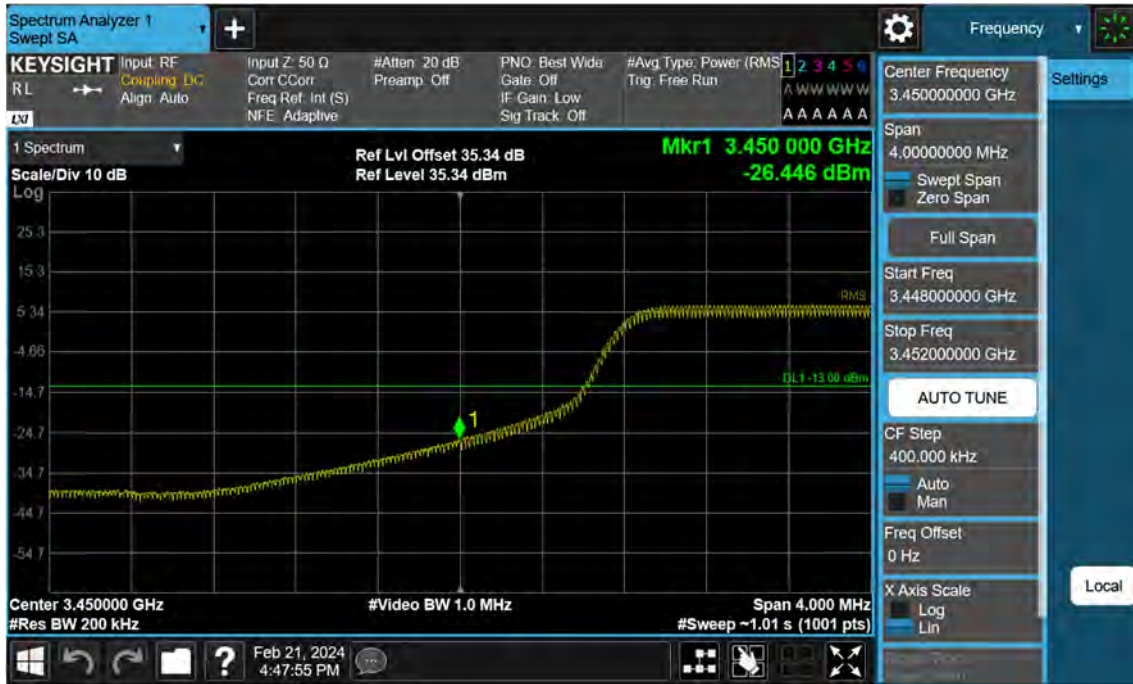
Sub6 n77. Low Band Edge Plot (20 M BW Ch.630668 BPSK FullRB)(1)
