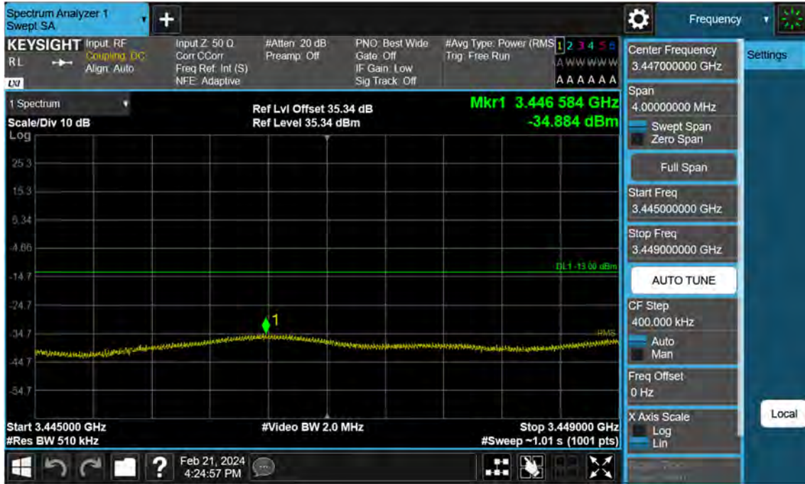
Sub6 n77. Low Band Edge Plot (10 M BW Ch.630334 BPSK 1RB)(2)
