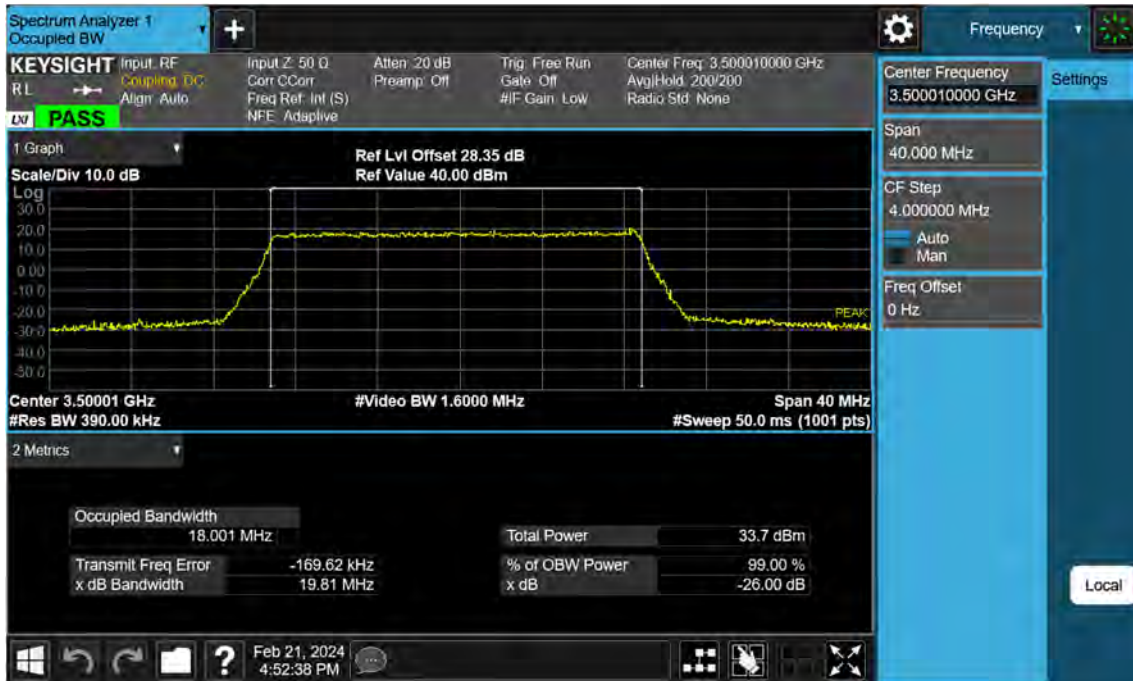
Sub6 n77. Occupied Bandwidth Plot (20 M BW Ch.633334 QPSK )
