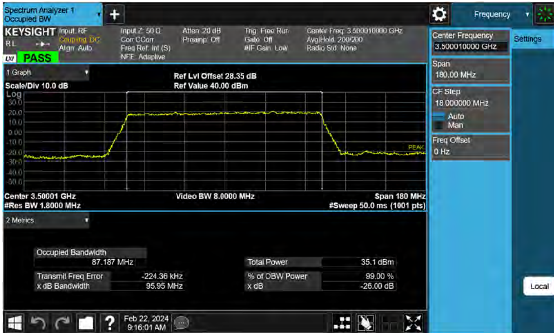
Sub6 n77. Occupied Bandwidth Plot (90 M BW Ch.633334 QPSK )
