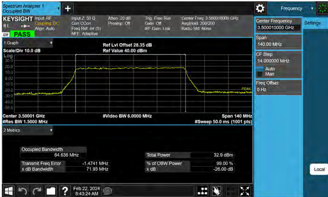
Sub6 n77. Occupied Bandwidth Plot (70 M BW Ch.633334 64QAM)
