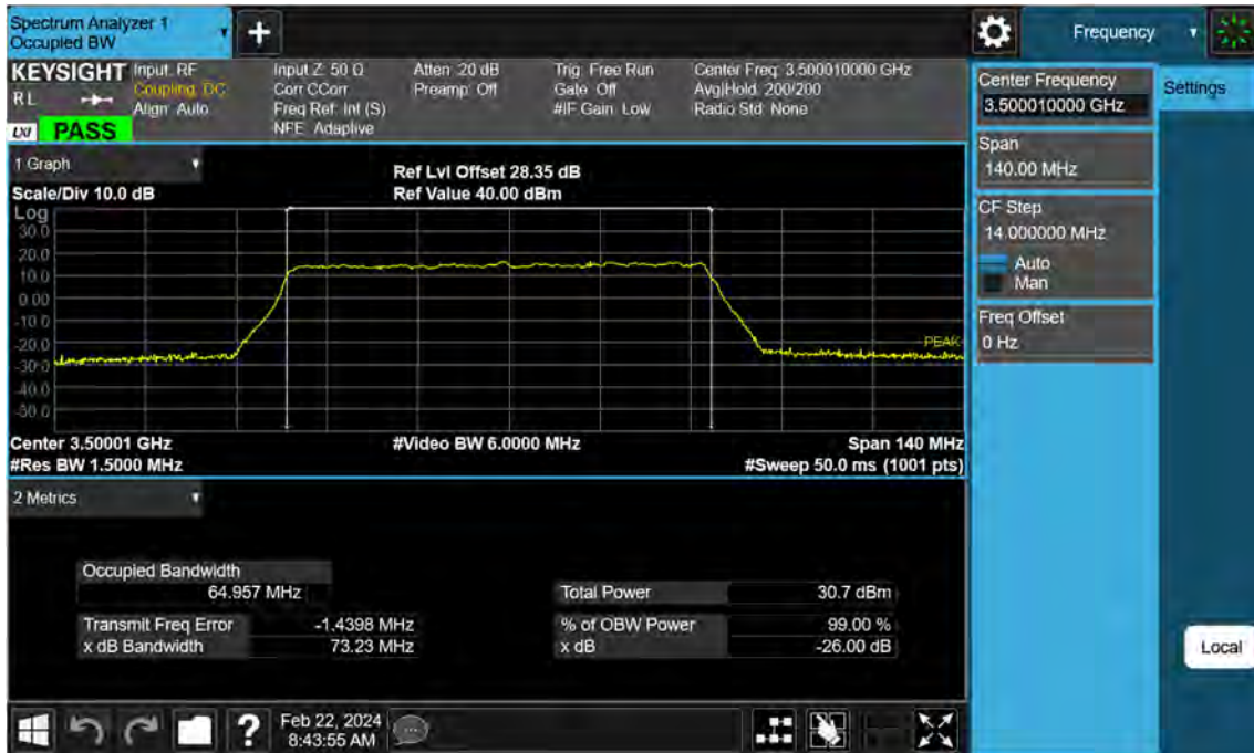
Sub6 n77. Occupied Bandwidth Plot (70 M BW Ch.633334 256QAM)
