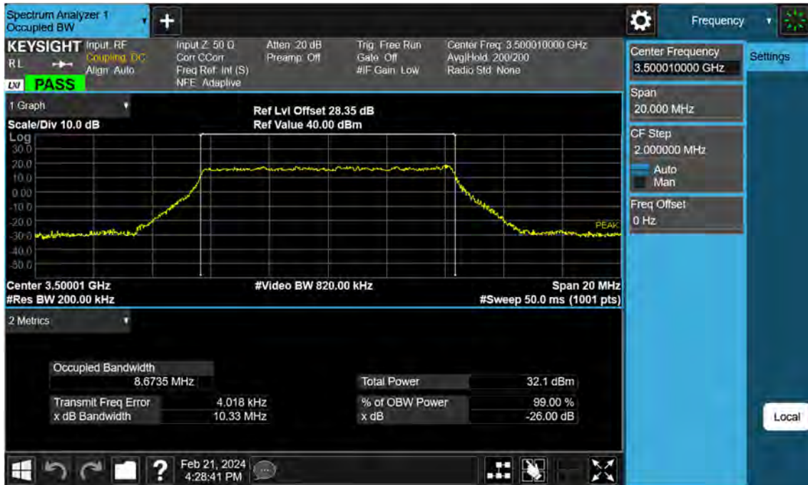
Sub6 n77. Occupied Bandwidth Plot (10 M BW Ch.633334 64QAM)
