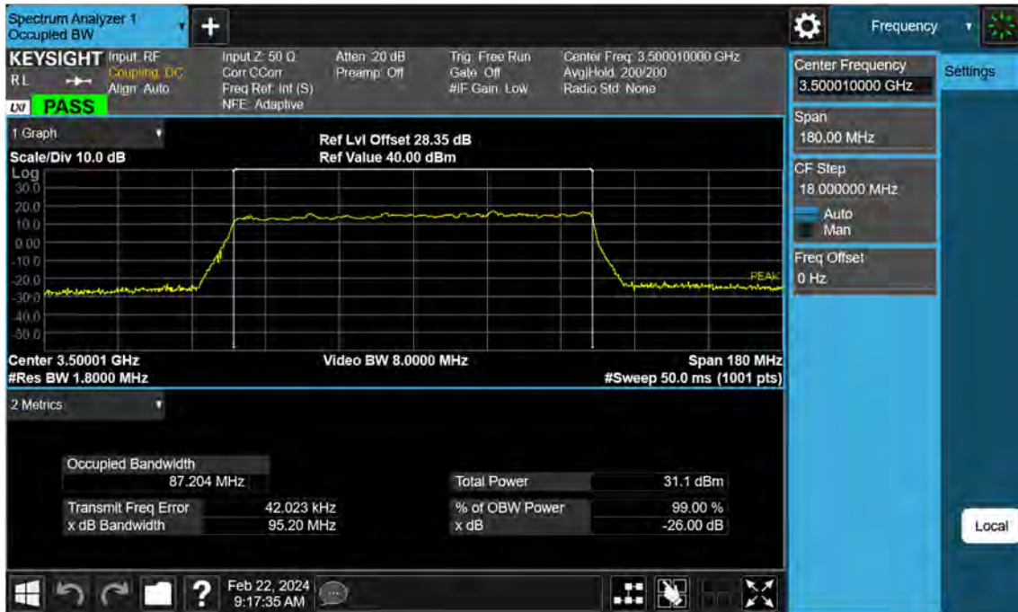
Sub6 n77. Occupied Bandwidth Plot (90 M BW Ch.633334 256QAM )
