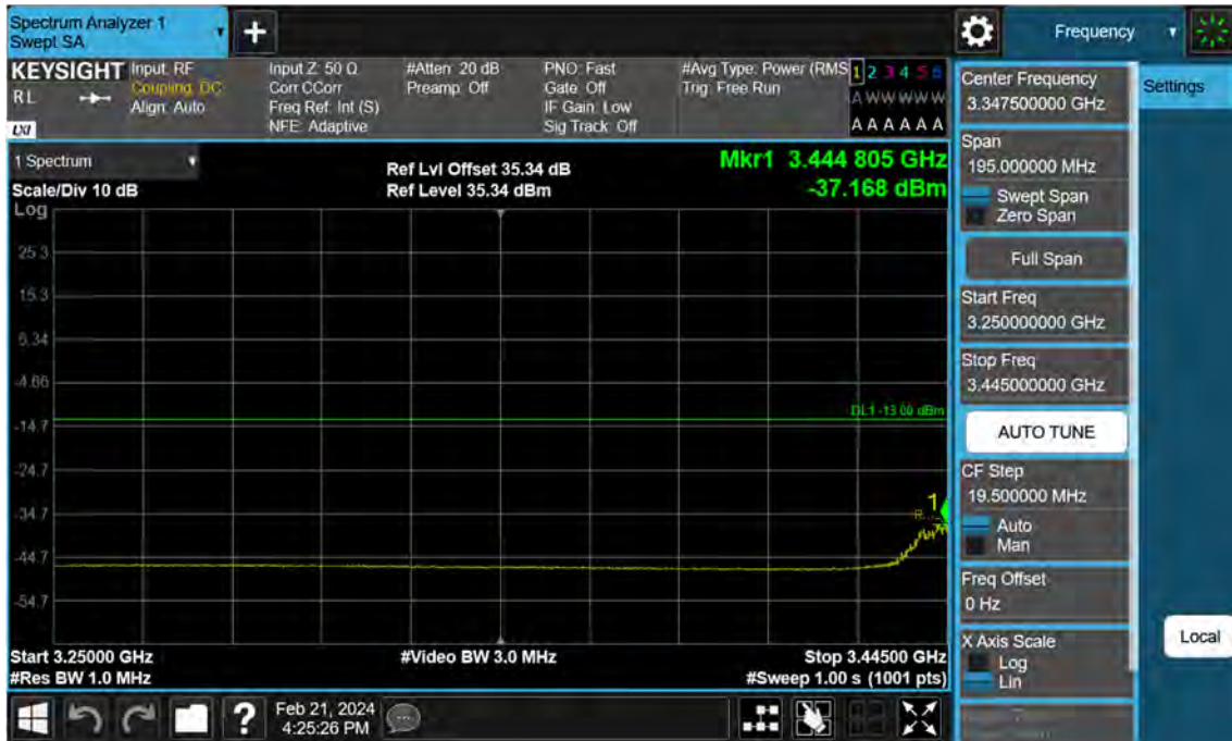
Sub6 n77. Low Band Edge Plot (10 M BW Ch.630334 BPSK 1RB)(3)
