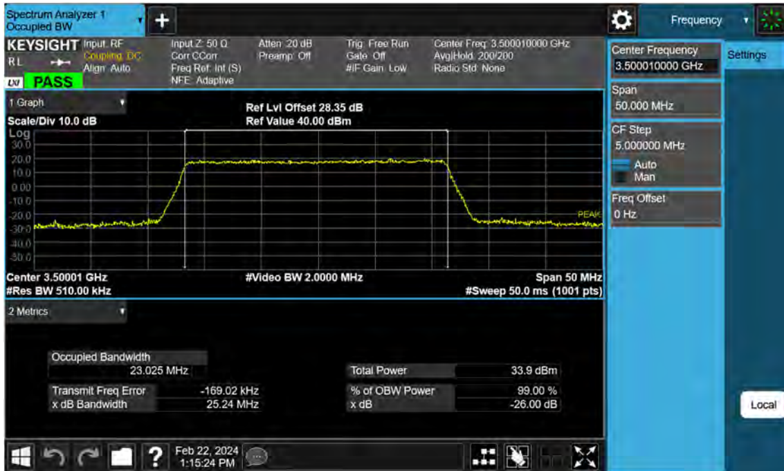
Sub6 n77. Occupied Bandwidth Plot (25 M BW Ch.633334 QPSK )
