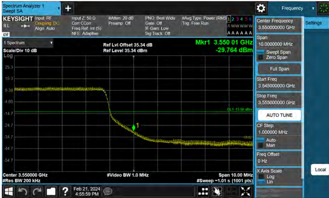
Sub6 n77. High Band Edge Plot (20 M BW Ch.636000 BPSK FullRB)(1)
