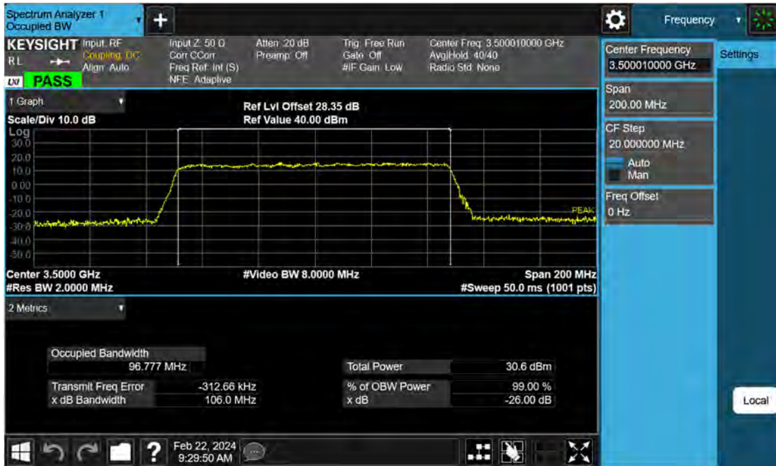
Sub6 n77. Occupied Bandwidth Plot (100 M BW Ch.633334 256QAM)
