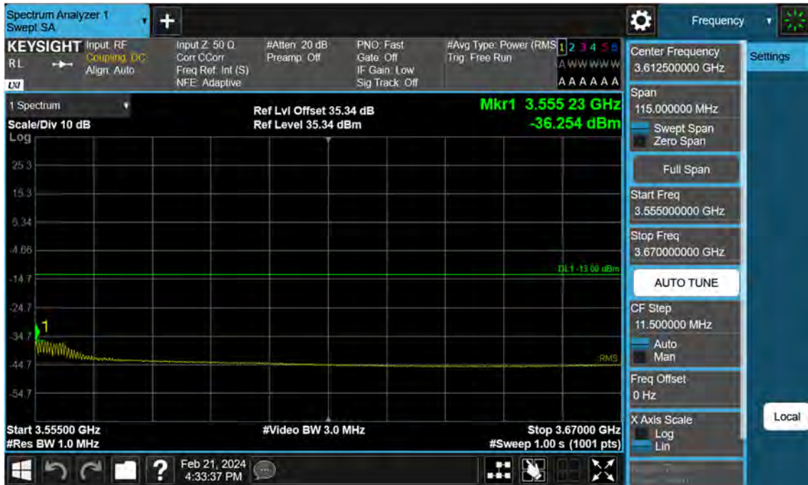
Sub6 n77. High Band Edge Plot (10 M BW Ch.636322 BPSK 1RB)(3)
