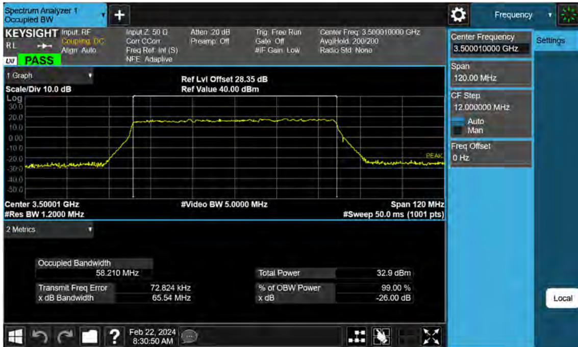
Sub6 n77. Occupied Bandwidth Plot (60 M BW Ch.633334 64QAM)
