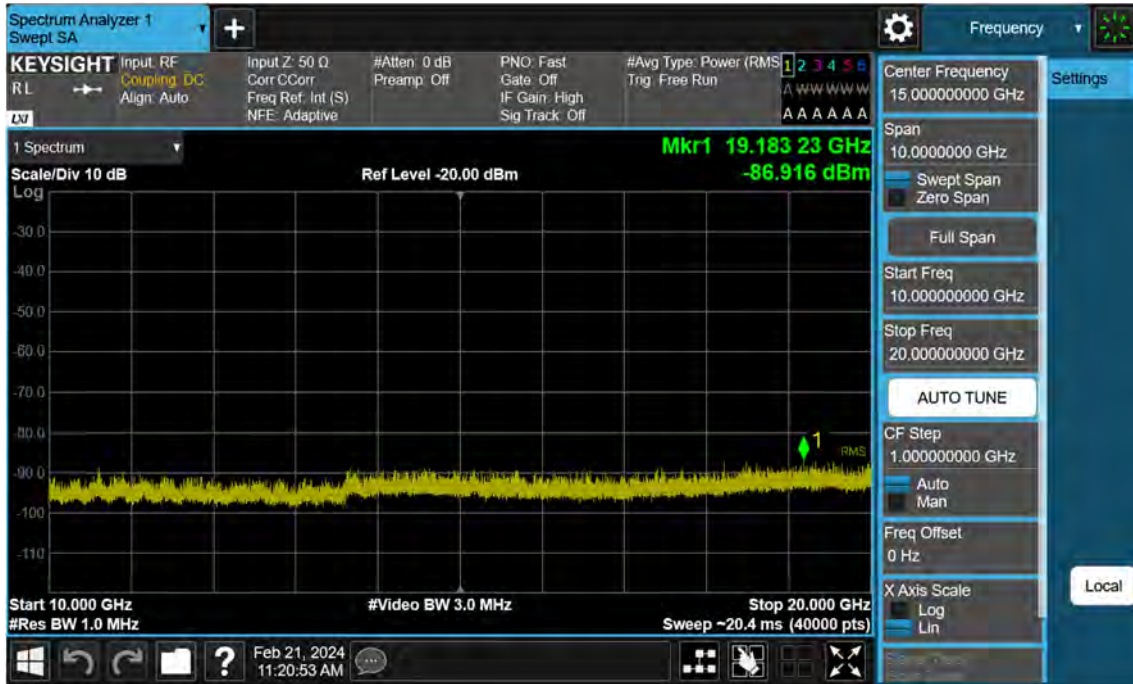
Sub6 n66. Conducted Spurious Plot_2 (349000ch_15 MHz_BPSK_RB 1_1)
