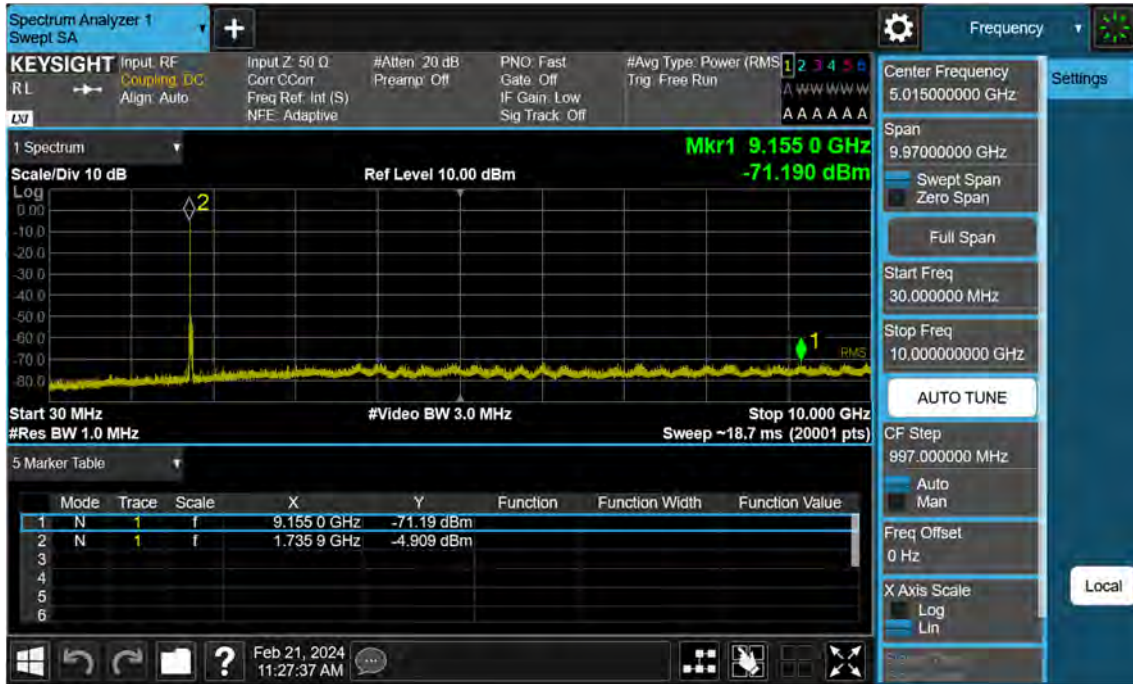
Sub6 n66. Conducted Spurious Plot_1 (349000ch_20 MHz_BPSK_RB 1_1)
