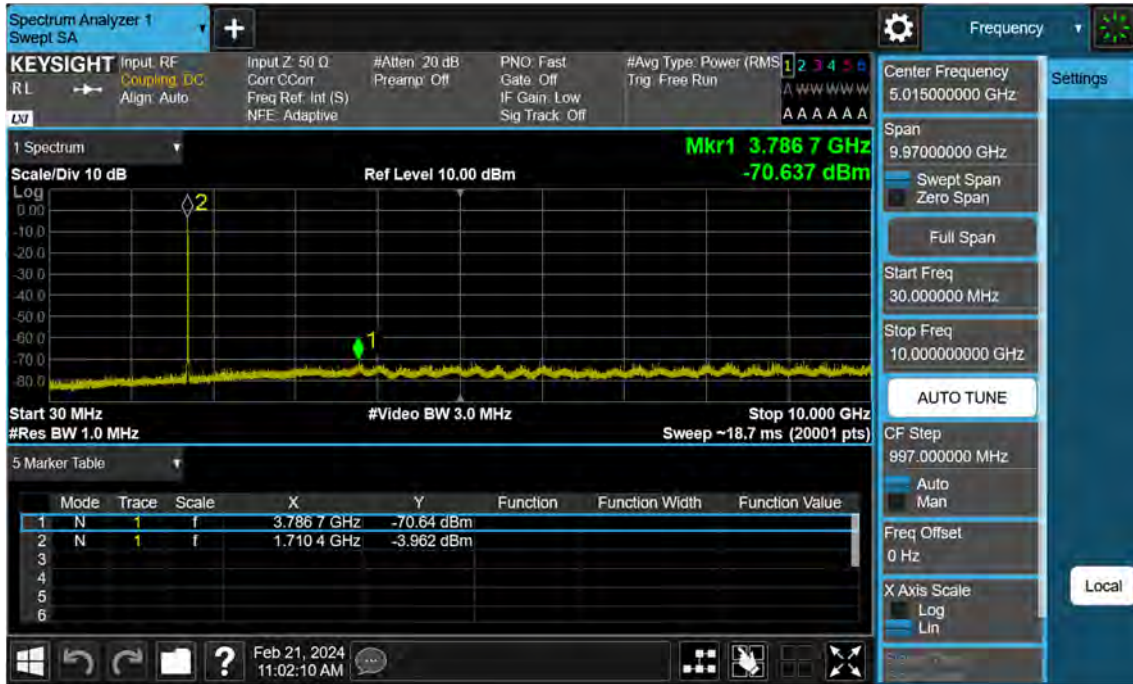
Sub6 n66. Conducted Spurious Plot_1 (342500ch_5 MHz_BPSK_RB 1_1)
