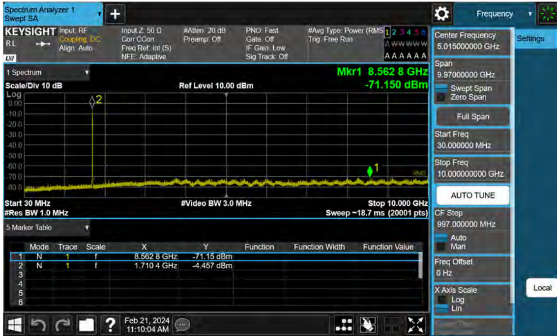
Sub6 n66. Conducted Spurious Plot_1 (343000ch_10 MHz_BPSK_RB 1_1)
