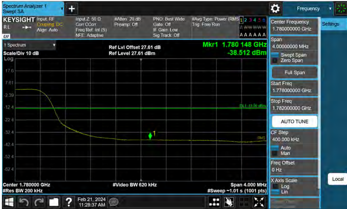
Sub6 n66. Upper Band Edge Plot (20 M BW Ch.354000 BPSK_ Full RB) -2
