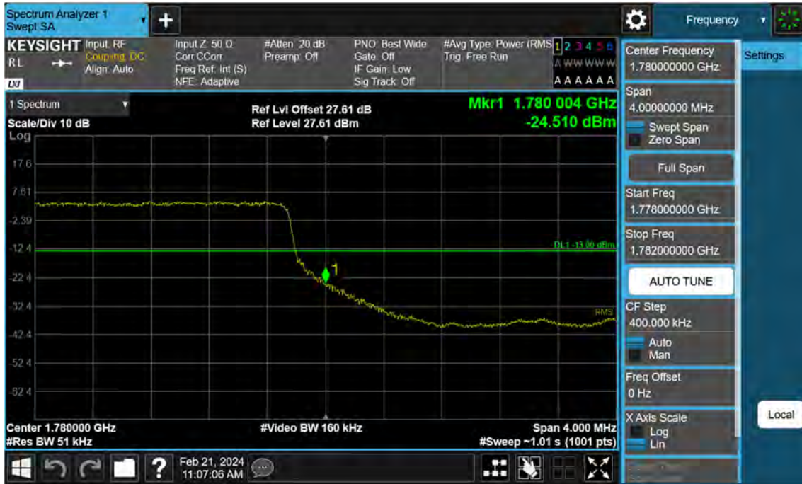
Sub6 n66. Upper Band Edge Plot (5 M BW Ch.355500 BPSK_ Full RB) -2
