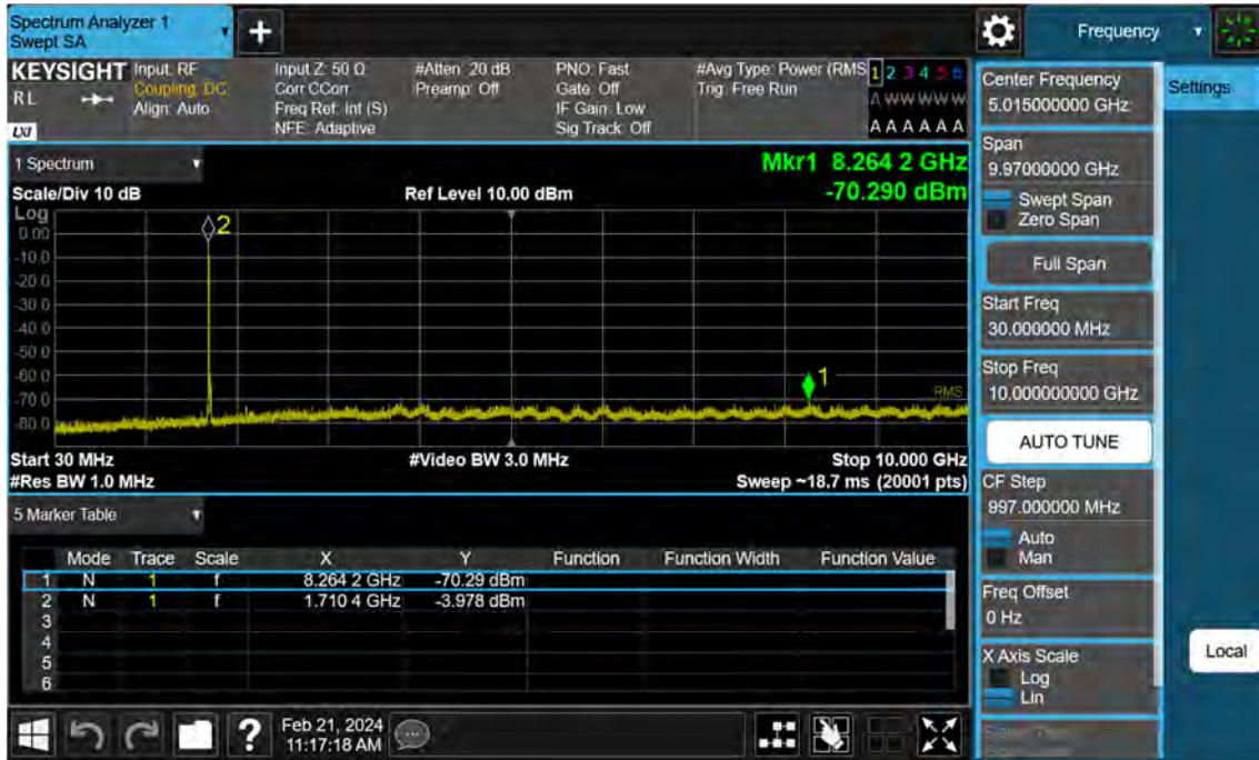
Sub6 n66. Conducted Spurious Plot_1 (343500ch_15 MHz_BPSK_RB 1_1)
