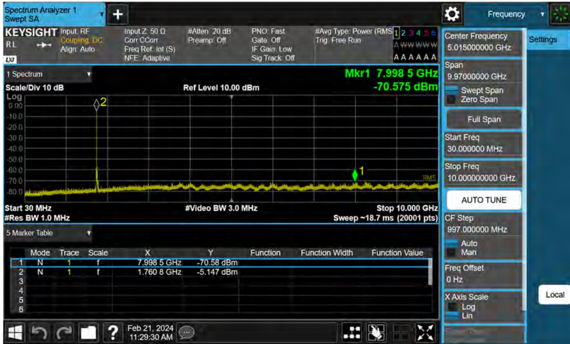
Sub6 n66. Conducted Spurious Plot_1 (354000ch_20 MHz_BPSK_RB 1_1)
