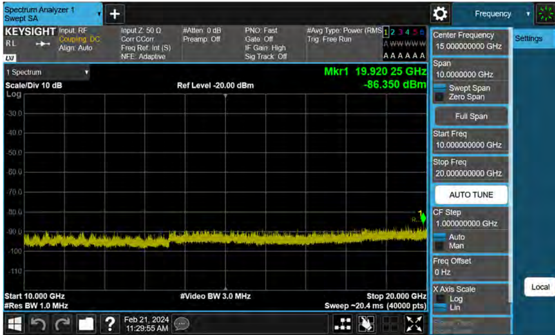
Sub6 n66. Conducted Spurious Plot_2 (354000ch_20 MHz_BPSK_RB 1_1)
