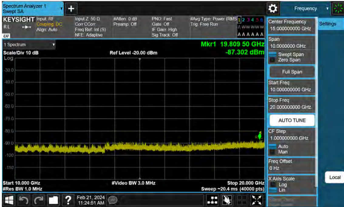
Sub6 n66. Conducted Spurious Plot_2 (344000ch_20 MHz_BPSK_RB 1_1)
