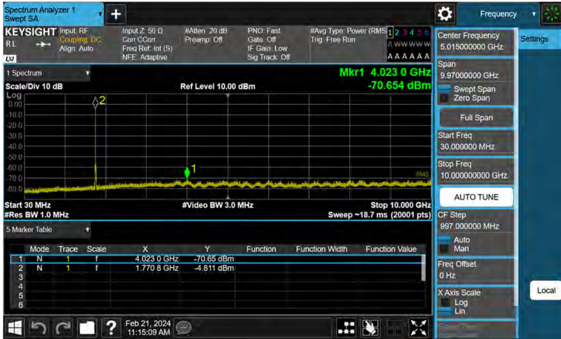
Sub6 n66. Conducted Spurious Plot_1 (355000ch_10 MHz_BPSK_RB 1_1)
