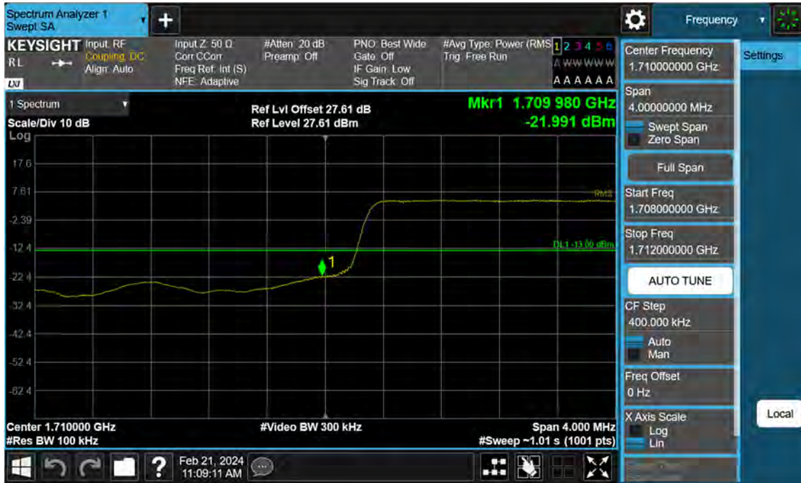
Sub6 n66. Lower Band Edge Plot (10 M BW Ch.343000 BPSK Full RB) -2
