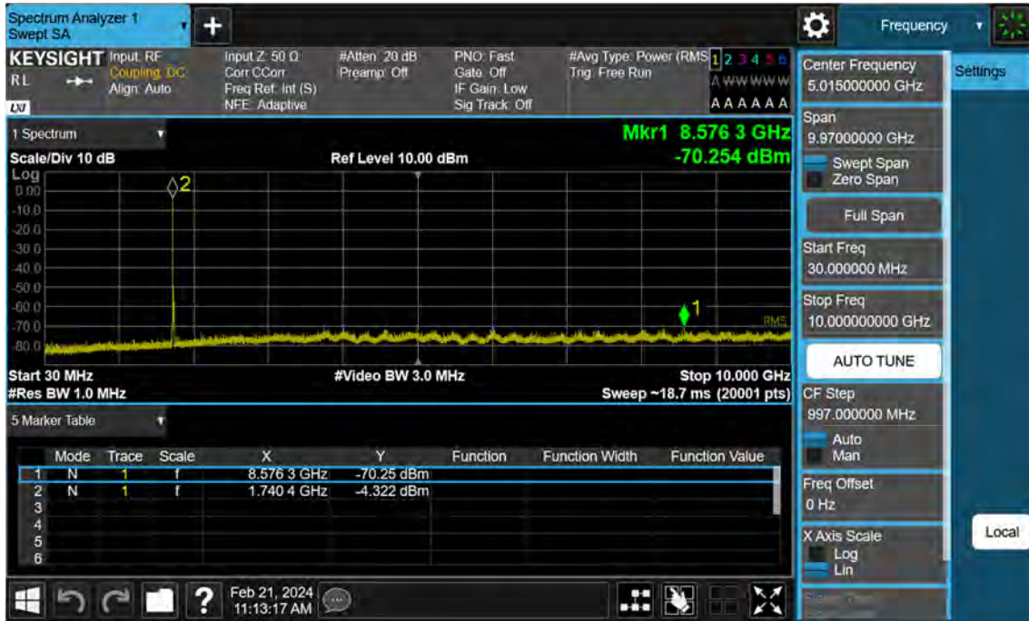
Sub6 n66. Conducted Spurious Plot_1 (349000ch_10 MHz_BPSK_RB 1_1)
