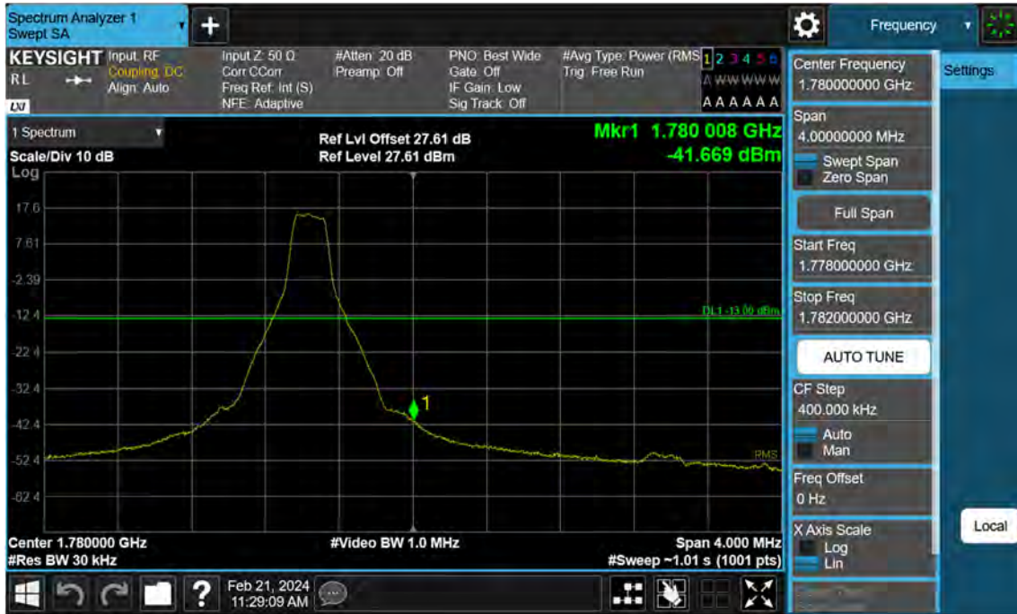
Sub6 n66. Upper Band Edge Plot (20 M BW Ch.354000 BPSK_RB1_Offset 105) -1
