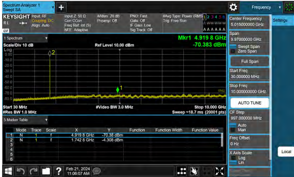
Sub6 n66. Conducted Spurious Plot_1 (349000ch_5 MHz_BPSK_RB 1_1)
