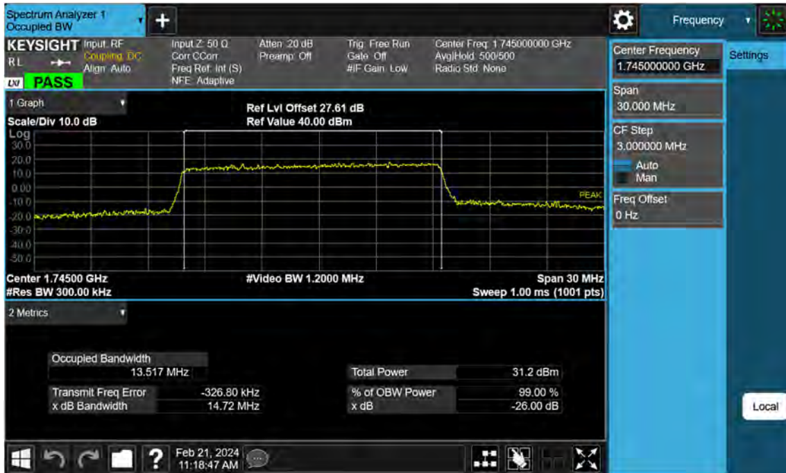
Sub6 n66. Occupied Bandwidth Plot (15 M BW Ch.349000 QPSK Full RB)
