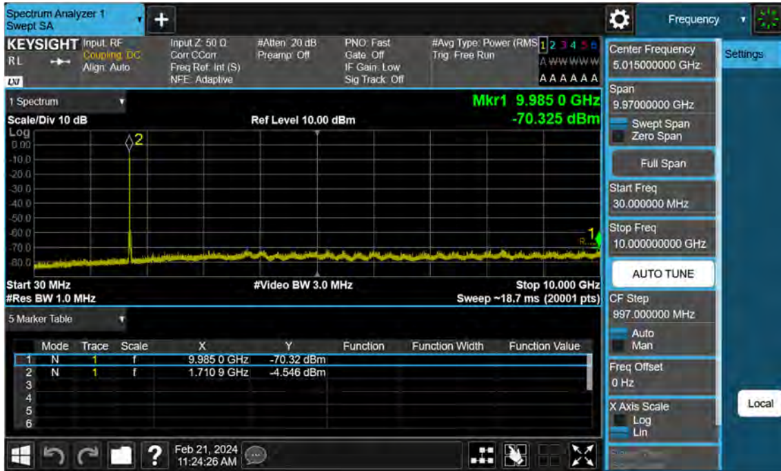
Sub6 n66. Conducted Spurious Plot_1 (344000ch_20 MHz_BPSK_ RB 1_1)
