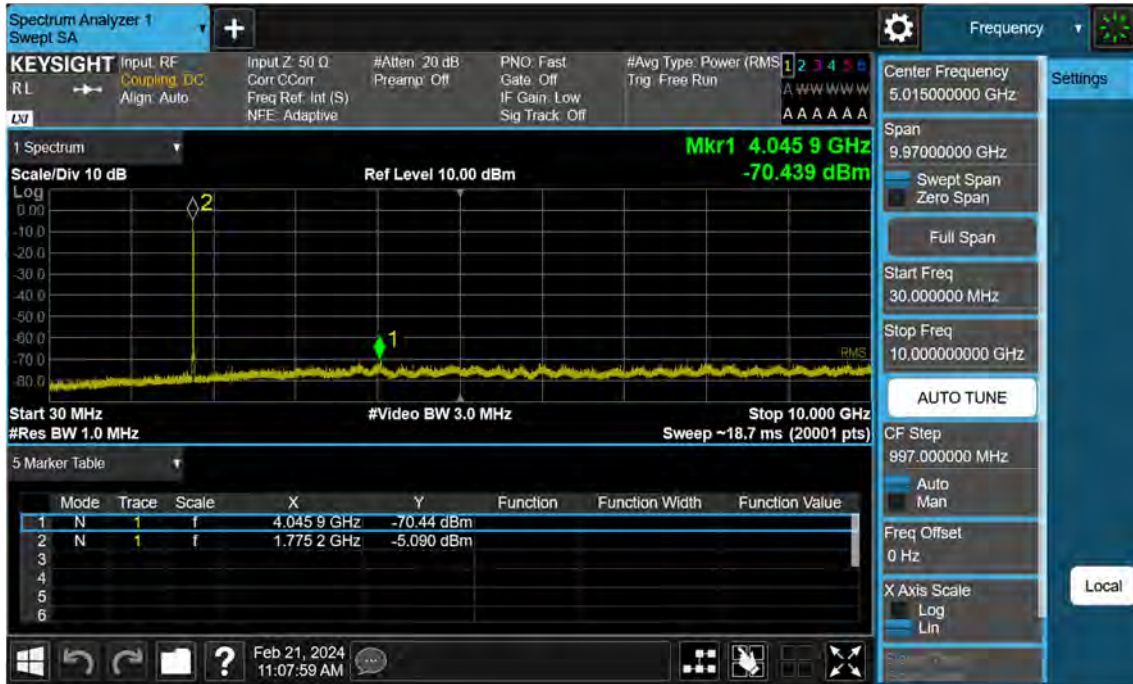
Sub6 n66. Conducted Spurious Plot_1 (355500ch_5 MHz_BPSK_RB 1_1)
