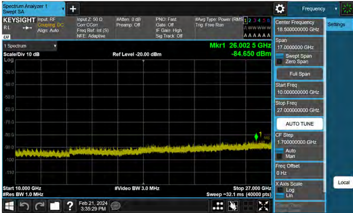
Sub6 n41. Conducted Spurious Plot 2 (80 MHz Ch.529998 BPSK RB 1)
