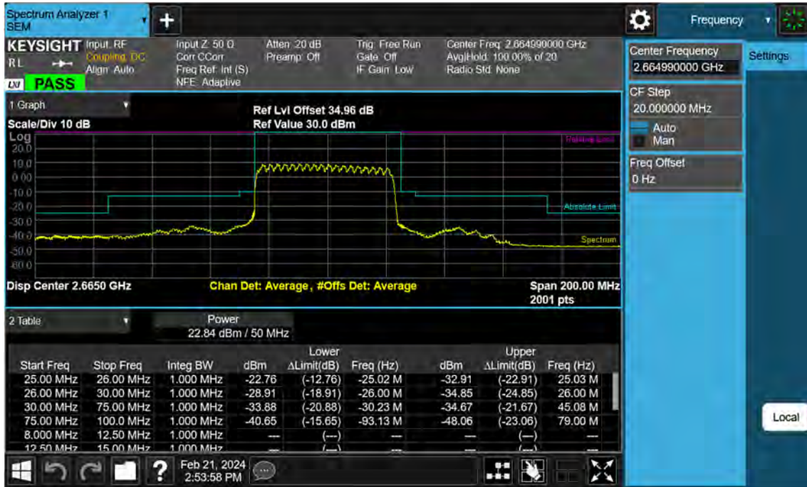
Sub6 n41. High Channel Edge Plot (50 MHz Ch.532998 BPSK)
