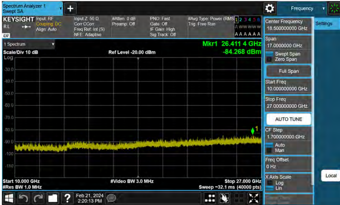
Sub6 n41. Conducted Spurious Plot 2 (30 MHz Ch.502200 BPSK RB 1)
