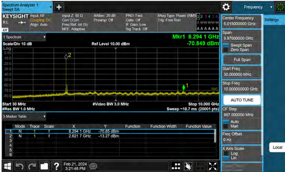
Sub6 n41. Conducted Spurious Plot 1 (70 MHz Ch.531000 BPSK RB 1)
