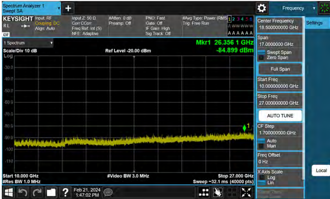
Sub6 n41. Conducted Spurious Plot 2 (10 MHz Ch. 518598 BPSK RB 1)
