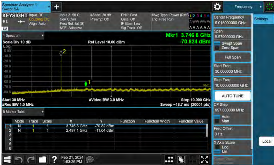
Sub6 n41. Conducted Spurious Plot 1 (15 MHz Ch.500700 BPSK RB 1)
