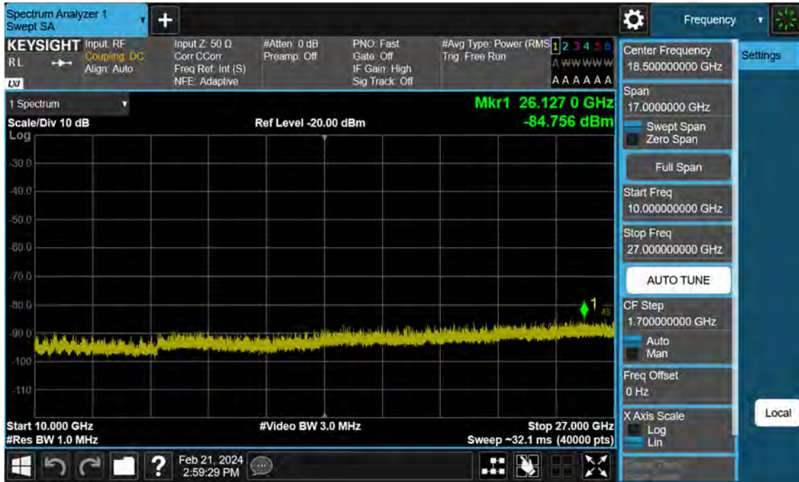
Sub6 n41. Conducted Spurious Plot 2 (60 MHz Ch.505200 BPSK RB 1)
