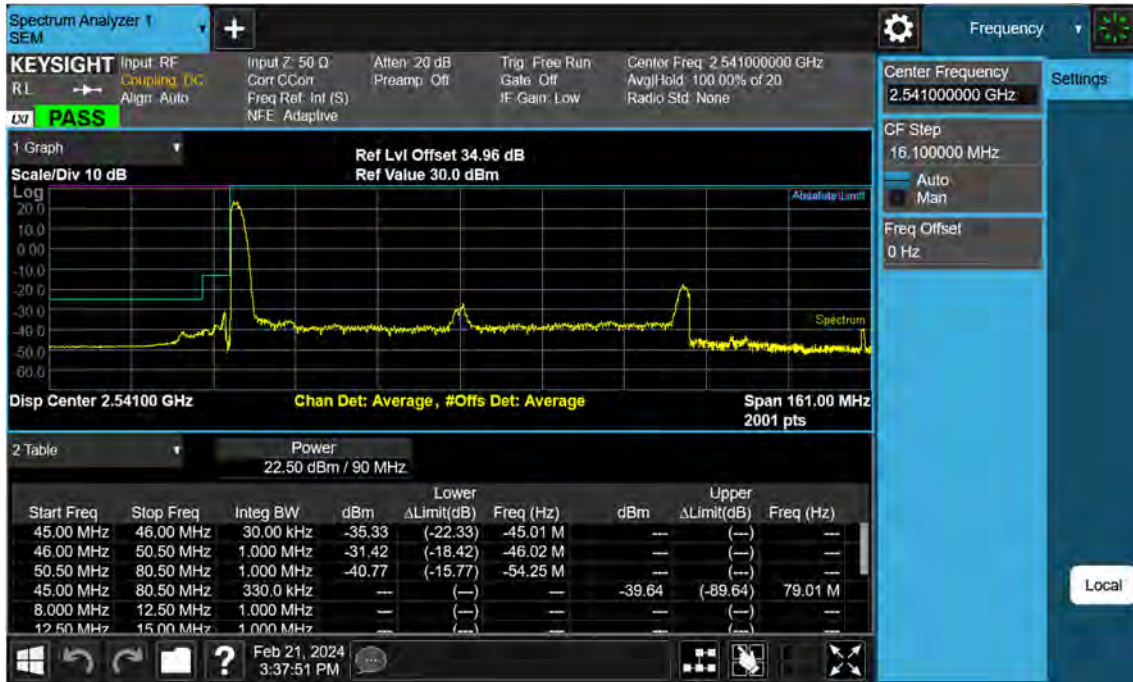
Sub6 n41. Low Channel Edge Plot (90 MHz Ch.508200 BPSK RB 1)-1
