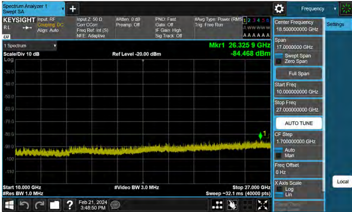
Sub6 n41. Conducted Spurious Plot 2 (90 MHz Ch.528996 BPSK RB 1)
