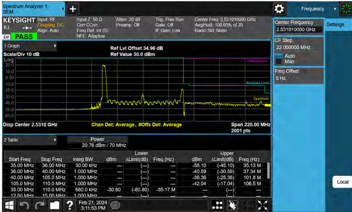
Sub6 n41. Low Channel Edge Plot (70 MHz Ch.506202 BPSK_RB1)-2
