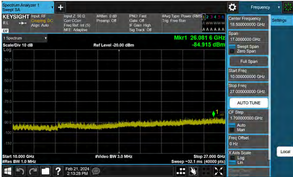
Sub6 n41. Conducted Spurious Plot 2 (20 MHz Ch. 518598 BPSK RB 1)
