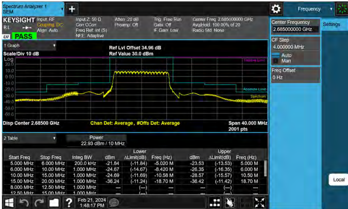
Sub6 n41. High Channel Edge Plot (10 MHz Ch.537000 BPSK)
