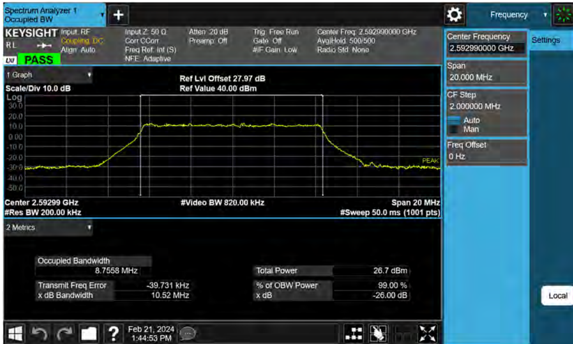
Sub6 n41. Occupied Bandwidth Plot (10 MHz Ch.518598 256-QAM)
