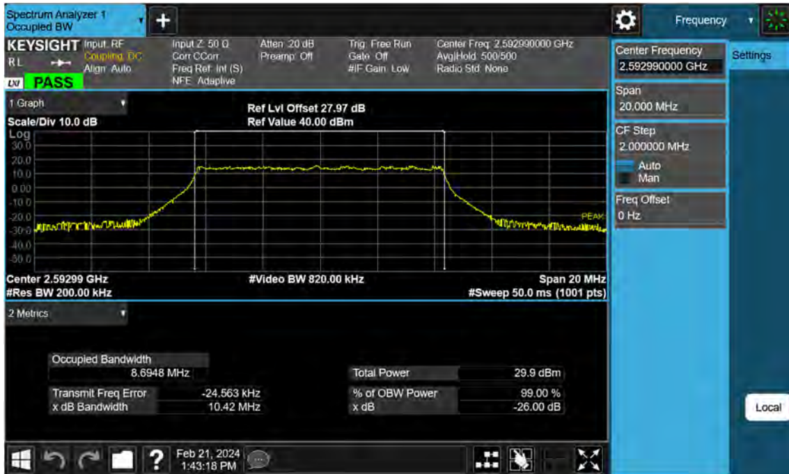
Sub6 n41. Occupied Bandwidth Plot (10 MHz Ch.518598 16-QAM )
