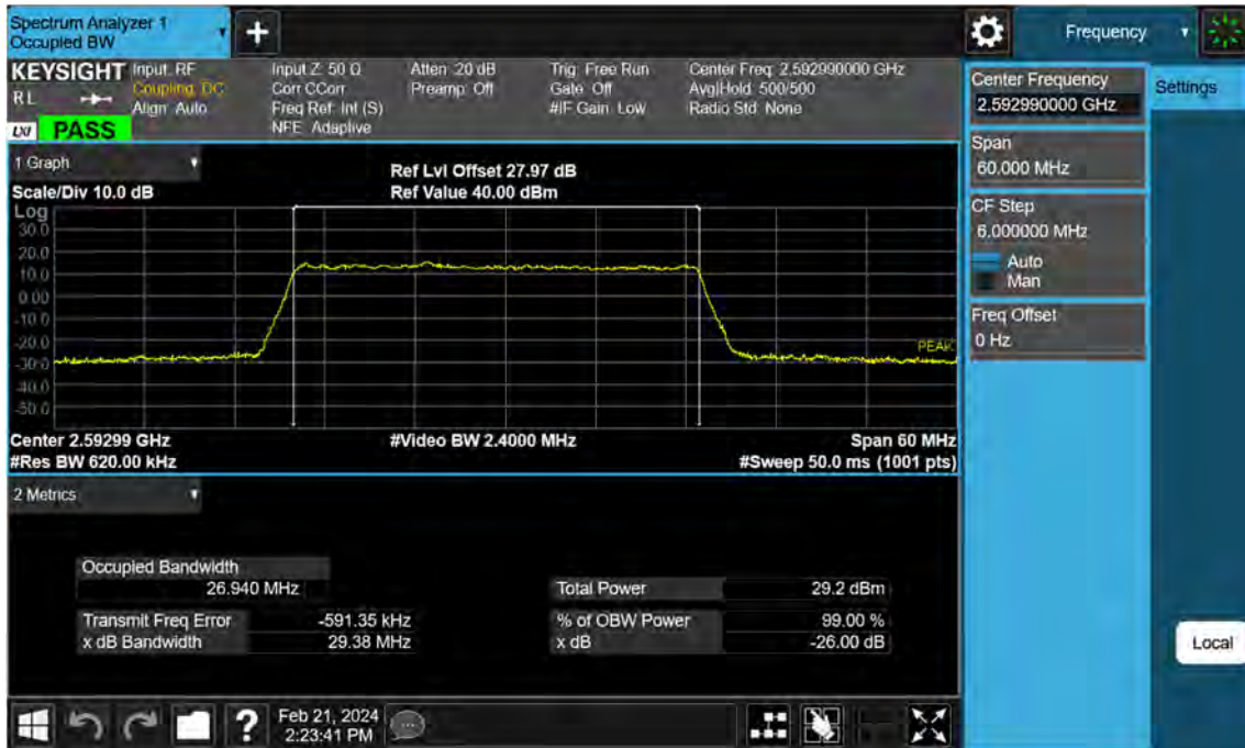
Sub6 n41. Occupied Bandwidth Plot (30 MHz Ch.518598 64-QAM )
