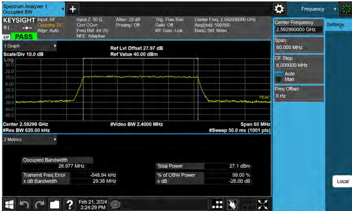
Sub6 n41. Occupied Bandwidth Plot (30 MHz Ch.518598 256-QAM)
