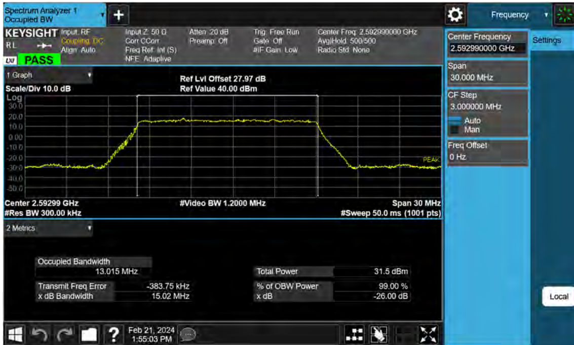
Sub6 n41. Occupied Bandwidth Plot (15 MHz Ch.518598 BPSK )
