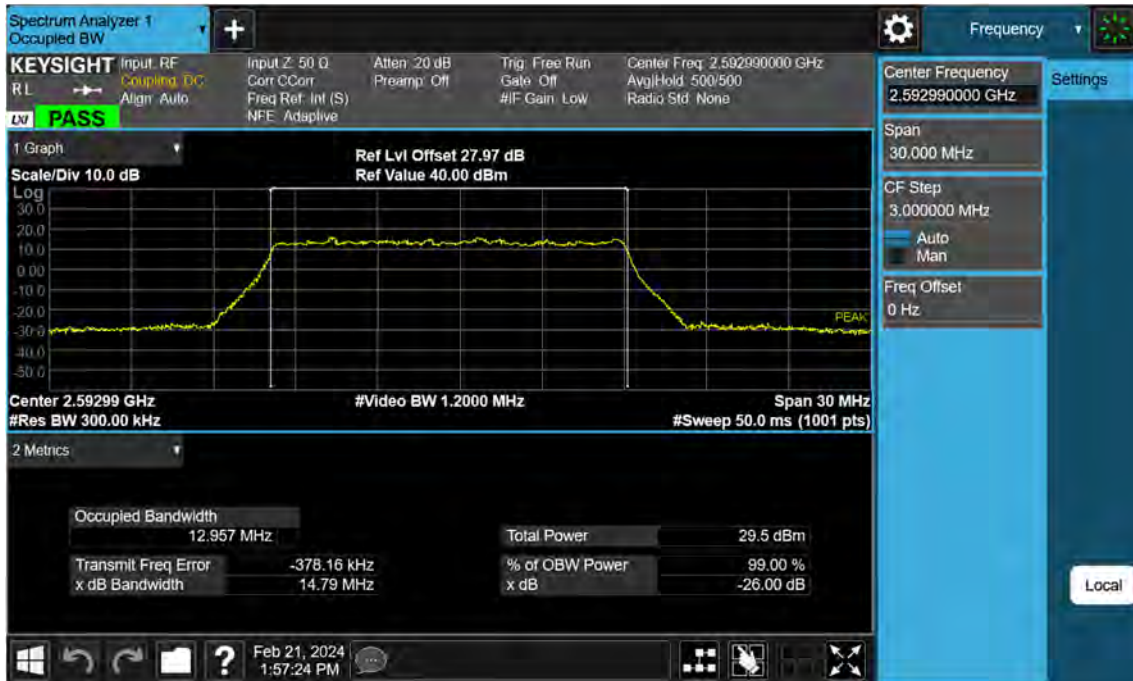
Sub6 n41. Occupied Bandwidth Plot (15 MHz Ch.518598 64-QAM )
