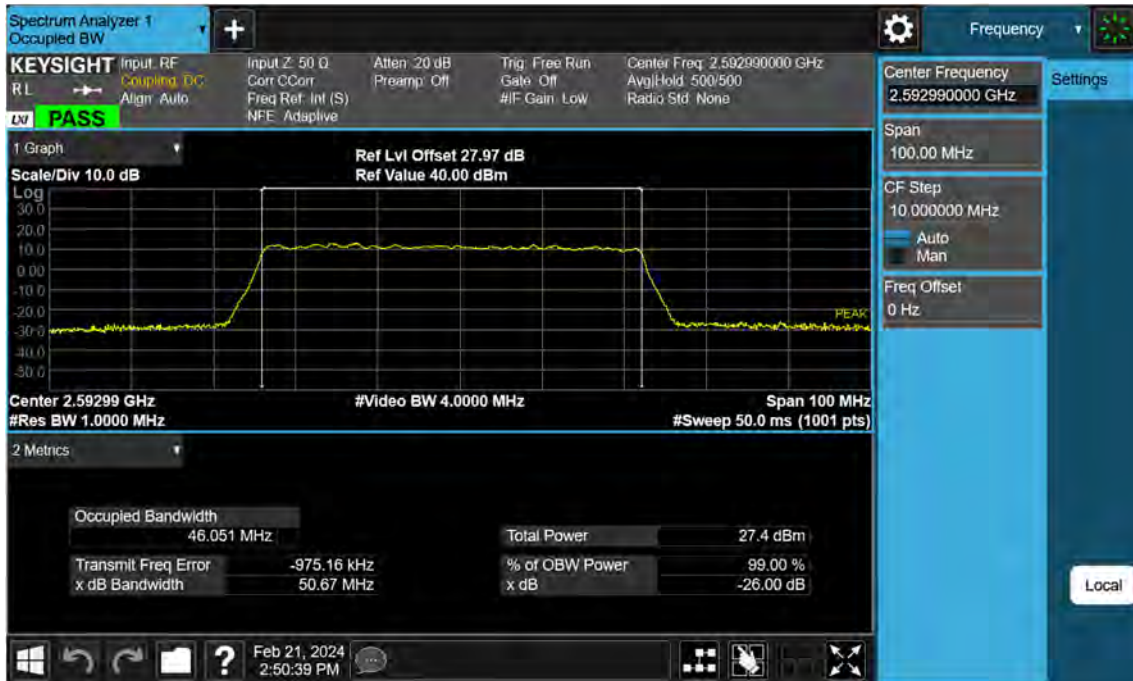
Sub6 n41. Occupied Bandwidth Plot (50 MHz Ch.518598 256-QAM)
