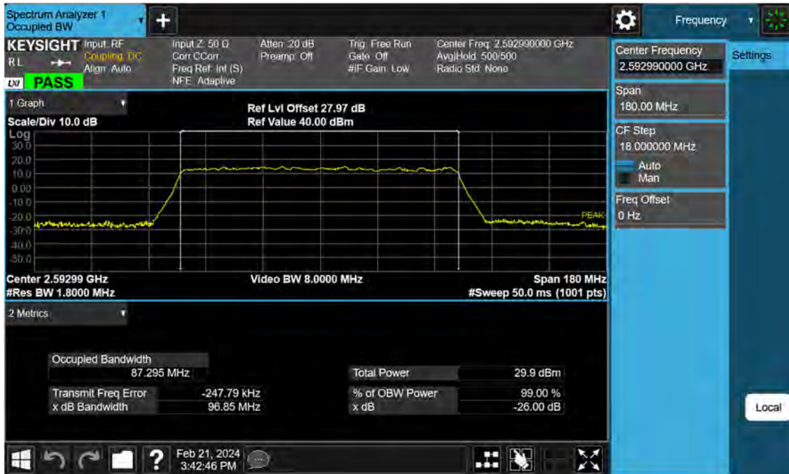
Sub6 n41. Occupied Bandwidth Plot (90 MHz Ch.518598 64-QAM )
