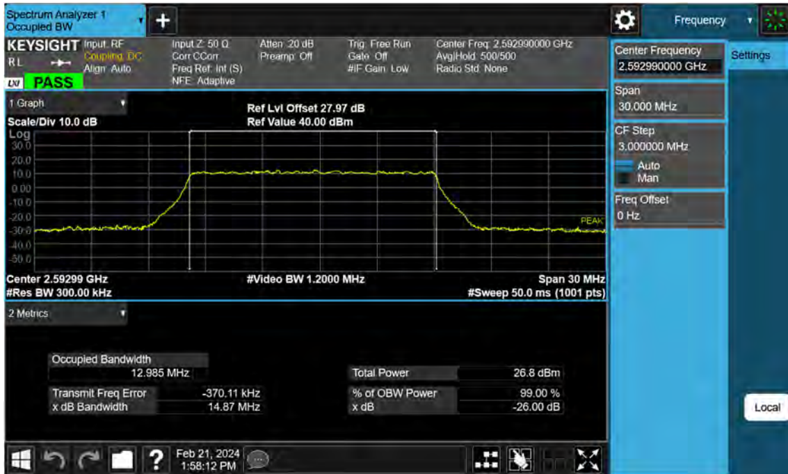
Sub6 n41. Occupied Bandwidth Plot (15 MHz Ch.518598 256-QAM)
