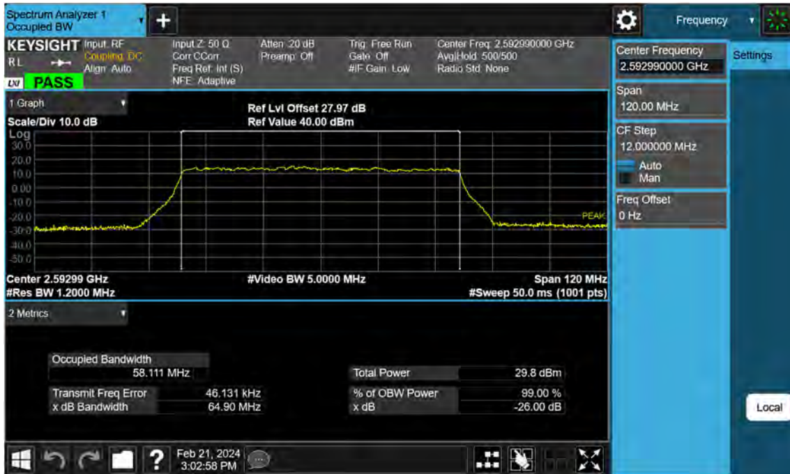
Sub6 n41. Occupied Bandwidth Plot (60 MHz Ch.518598 64-QAM )
