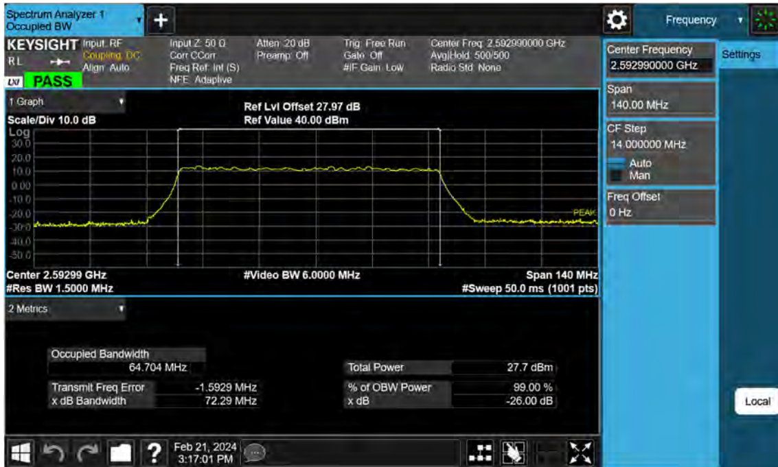
Sub6 n41. Occupied Bandwidth Plot (70 MHz Ch.518598 256-QAM)
