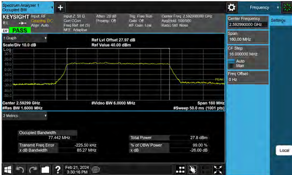
Sub6 n41. Occupied Bandwidth Plot (80 MHz Ch.518598 256-QAM )
