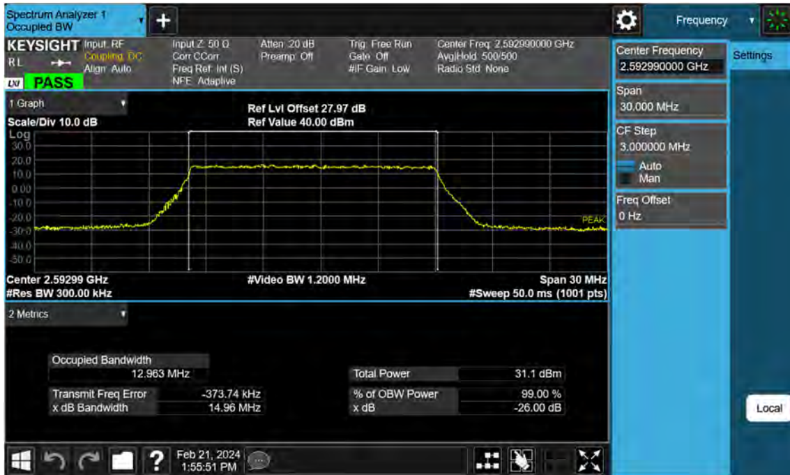
Sub6 n41. Occupied Bandwidth Plot (15 MHz Ch.518598 QPSK)
