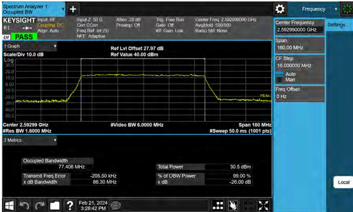
Sub6 n41. Occupied Bandwidth Plot (80 MHz Ch.518598 16-QAM )
