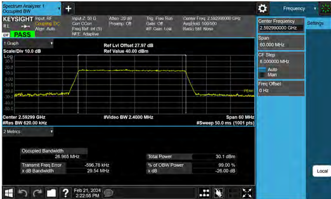
Sub6 n41. Occupied Bandwidth Plot (30 MHz Ch.518598 16-QAM )
