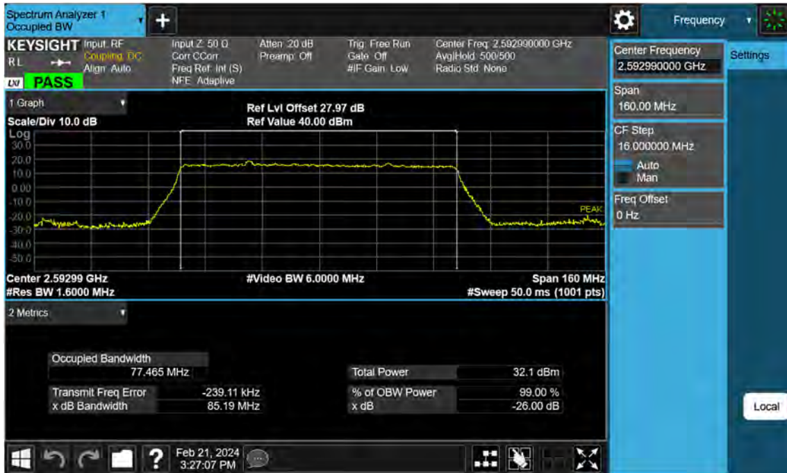
Sub6 n41. Occupied Bandwidth Plot (80 MHz Ch.518598 BPSK)
