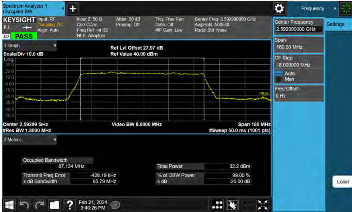
Sub6 n41. Occupied Bandwidth Plot (90 MHz Ch.518598 BPSK )
