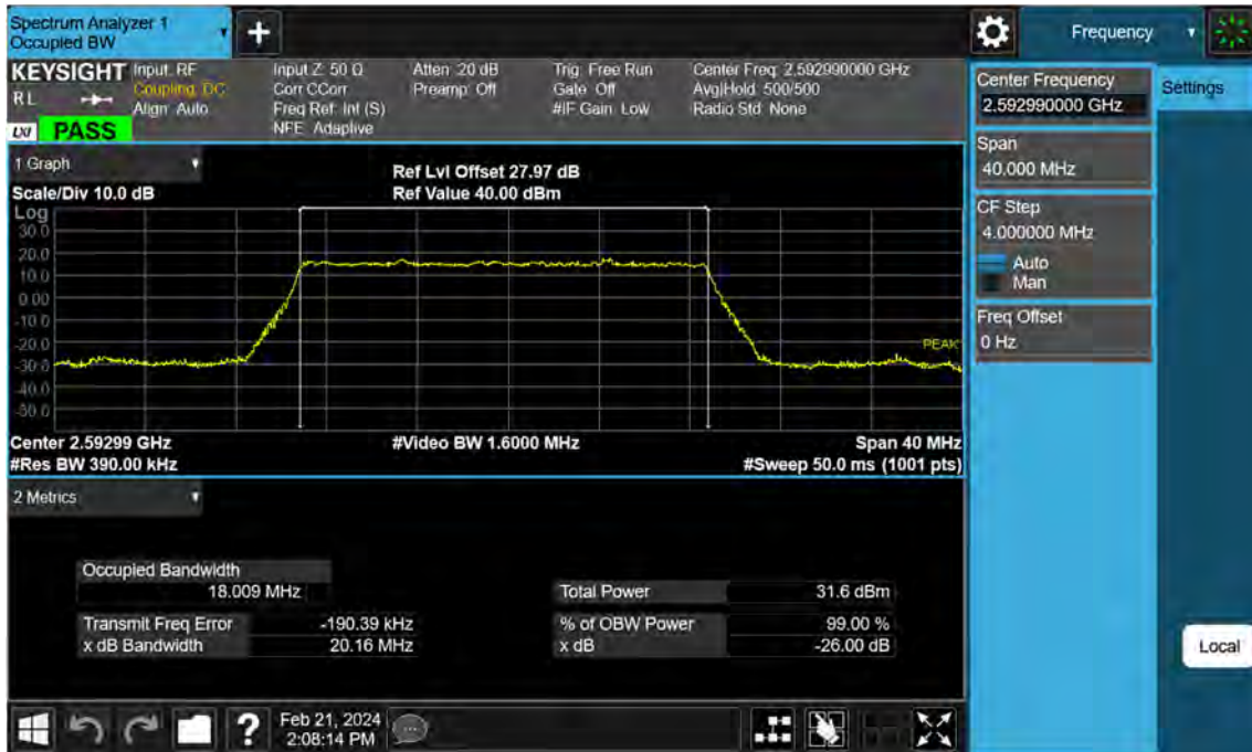
Sub6 n41. Occupied Bandwidth Plot (20 MHz Ch.518598 BPSK)
