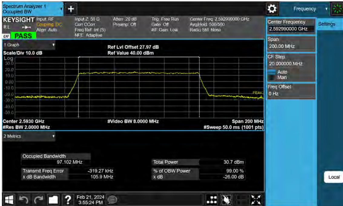
Sub6 n41. Occupied Bandwidth Plot (100 MHz Ch.518598 16-QAM)
