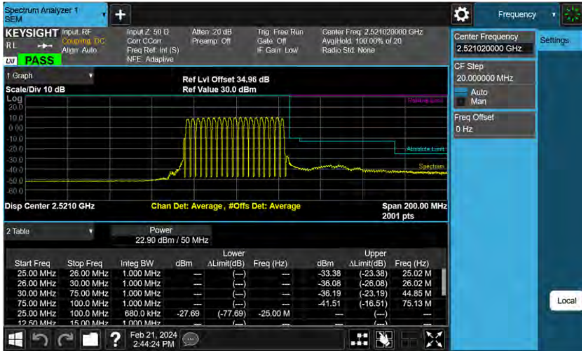
Sub6 n41. Low Channel Edge Plot (50 MHz Ch.504204 BPSK)-2
