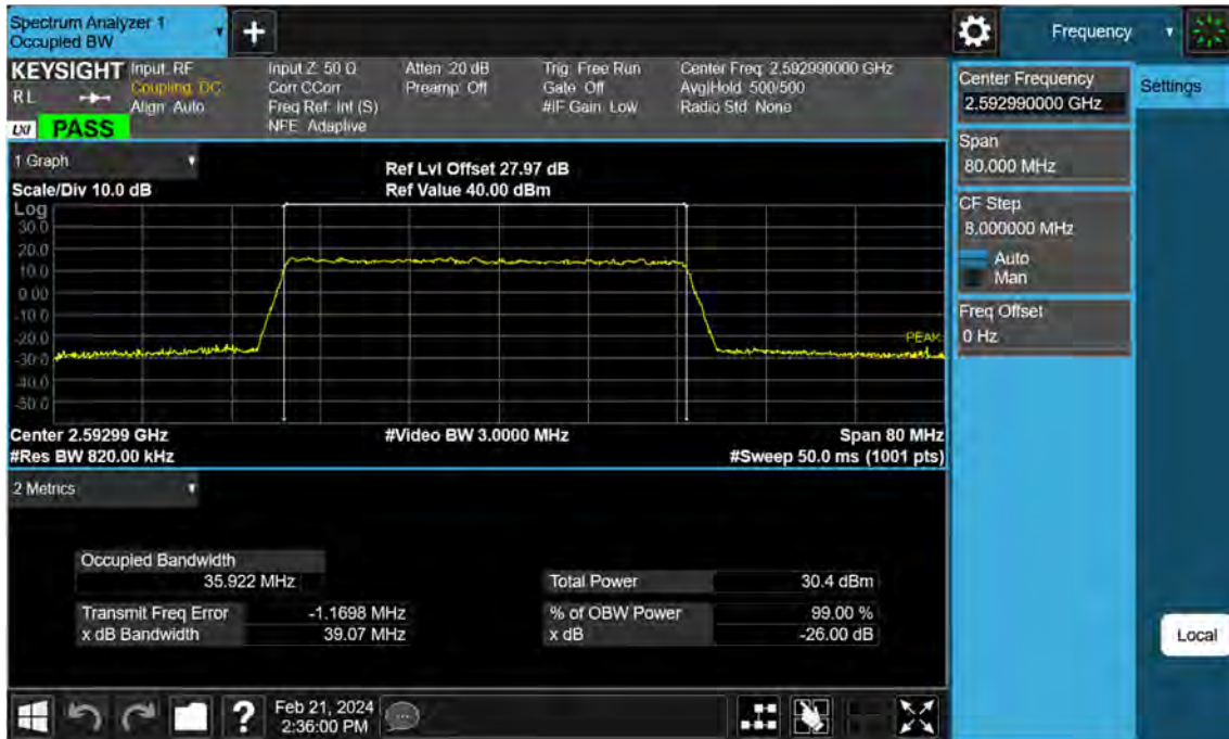
Sub6 n41. Occupied Bandwidth Plot (40 MHz Ch.518598 16-QAM )
