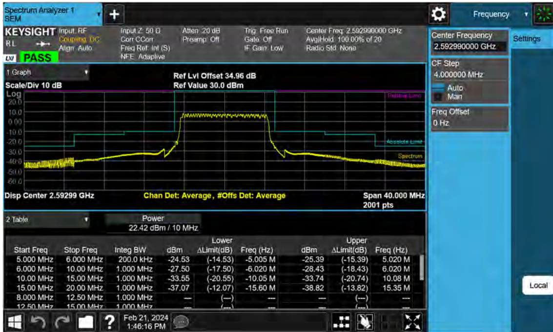
Sub6 n41. Mid Channel Edge Plot (10 MHz Ch.518598 BPSK)
