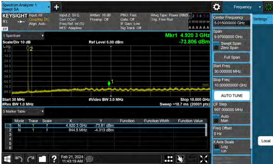
Sub6 n5. Conducted Spurious Plot (169300ch_5 MHz_BPSK_RB 1_1)
