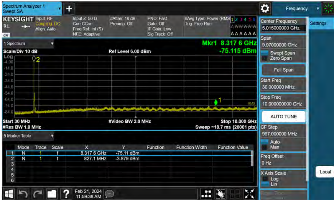
Sub6 n5. Conducted Spurious Plot (167300ch_20 MHz_BPSK_RB 1_1)
