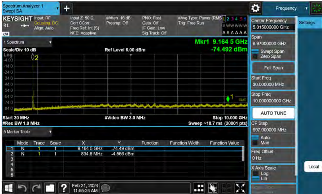
Sub6 n5. Conducted Spurious Plot (168300ch_15 MHz_BPSK_RB 1_1)
