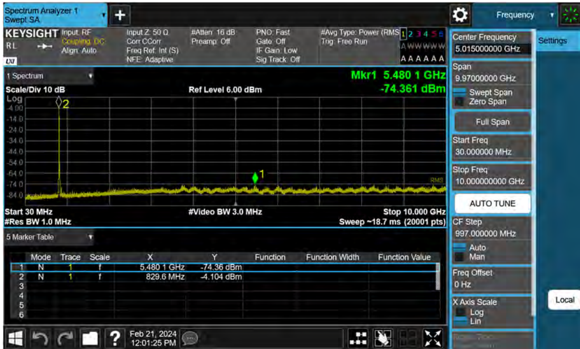
Sub6 n5. Conducted Spurious Plot (167800ch_20 MHz_BPSK_RB 1_1)
