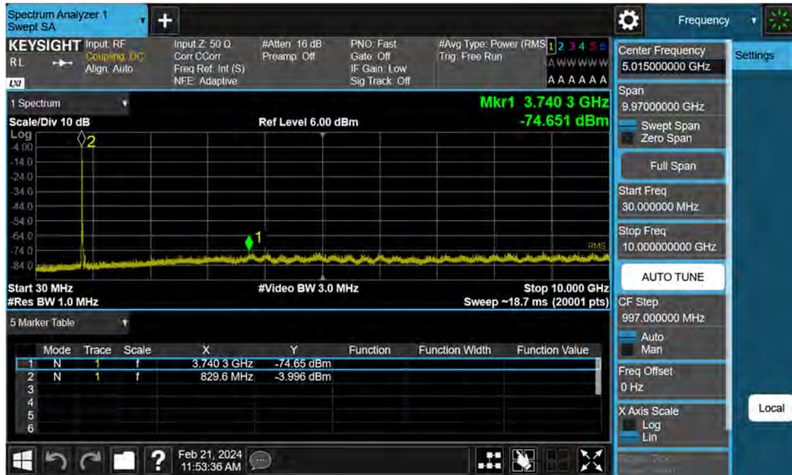
Sub6 n5. Conducted Spurious Plot (167300ch_15 MHz_BPSK_RB 1_1)
