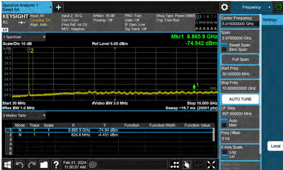
Sub6 n5. Conducted Spurious Plot (166300ch_15 MHz_BPSK_RB 1_1)
