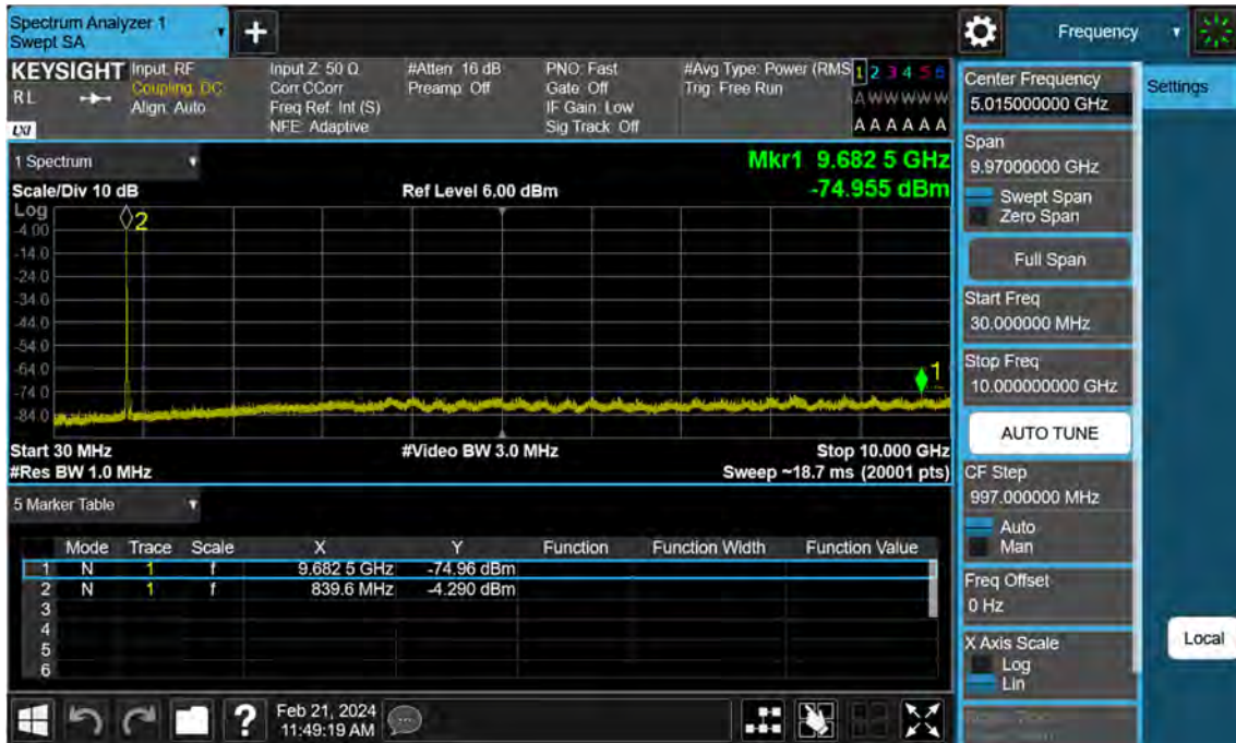
Sub6 n5. Conducted Spurious Plot (168800ch_10 MHz_BPSK_RB 1_1)
