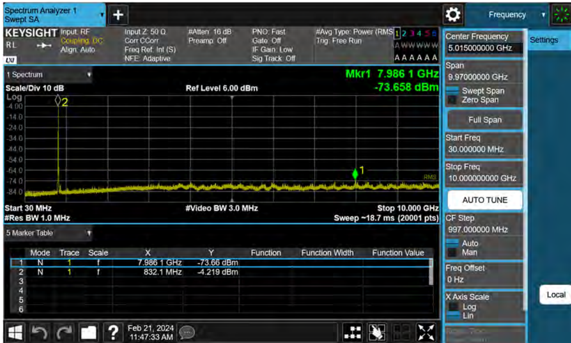
Sub6 n5. Conducted Spurious Plot (167300ch_10 MHz_BPSK_RB 1_1)
