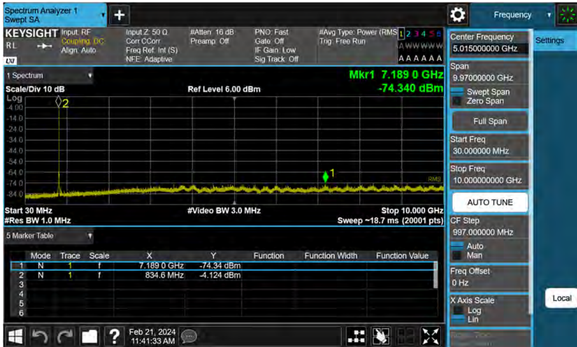
Sub6 n5. Conducted Spurious Plot (167300ch_5 MHz_BPSK_RB 1_1)
