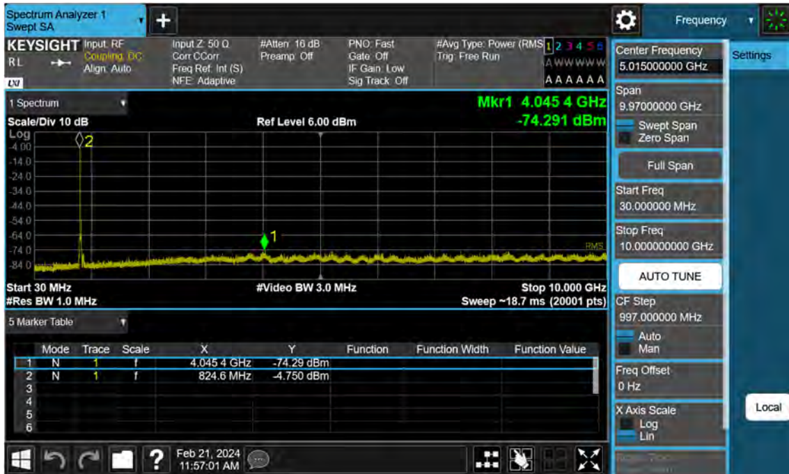
Sub6 n5. Conducted Spurious Plot (166800ch_20 MHz_BPSK_RB 1_1)
