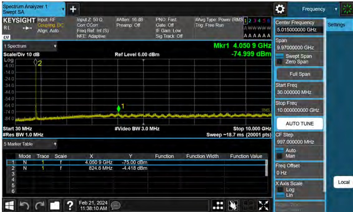
Sub6 n5. Conducted Spurious Plot (165300ch_5 MHz_BPSK_RB 1_1)
