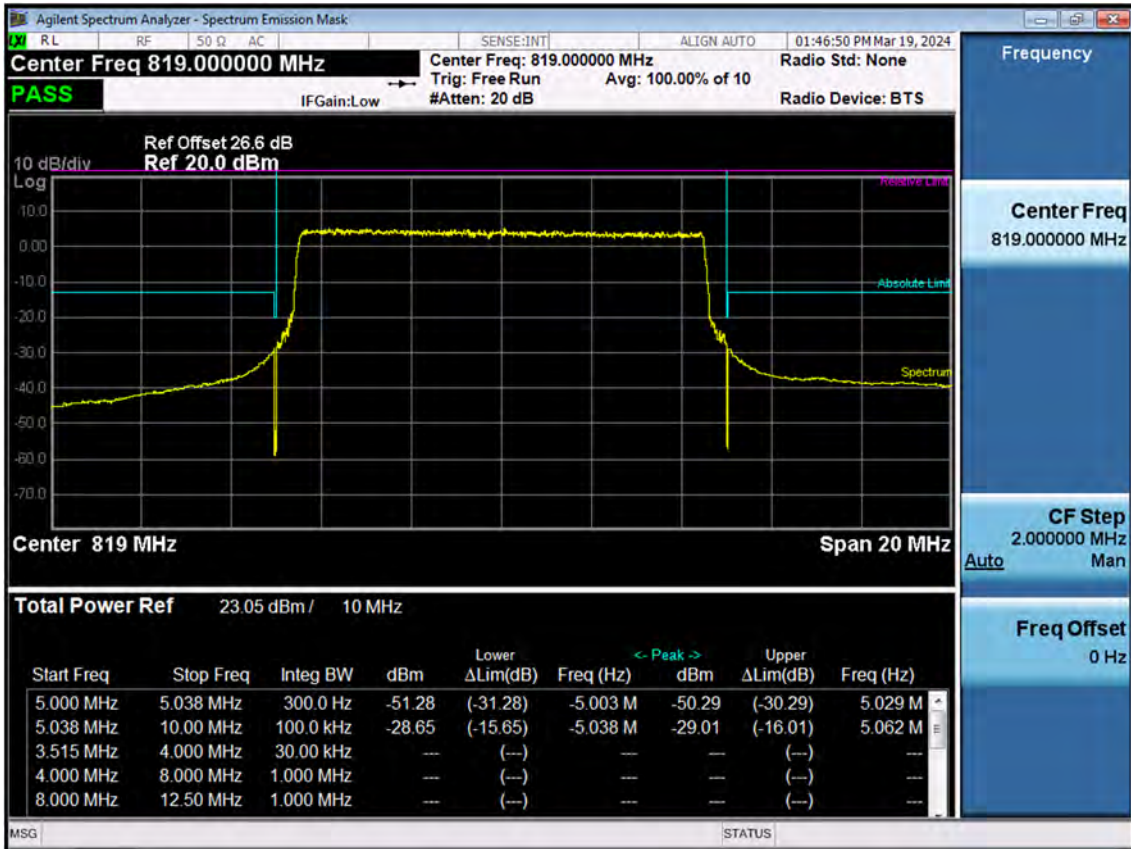
BAND 26. Low Channel Edge Plot (10 M BW Ch.26740 QPSK_RB50_Offset 0)
