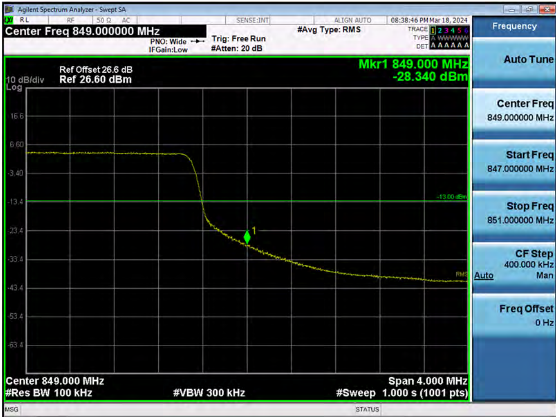
BAND5/26. Upper Band Edge Plot (10 M BW Ch.26990 QPSK_RB50_Offset 0)
