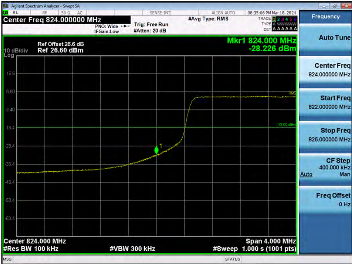
BAND5/26. Lower Band Edge Plot (10 M BW Ch.26840 QPSK_RB50_Offset 0)
