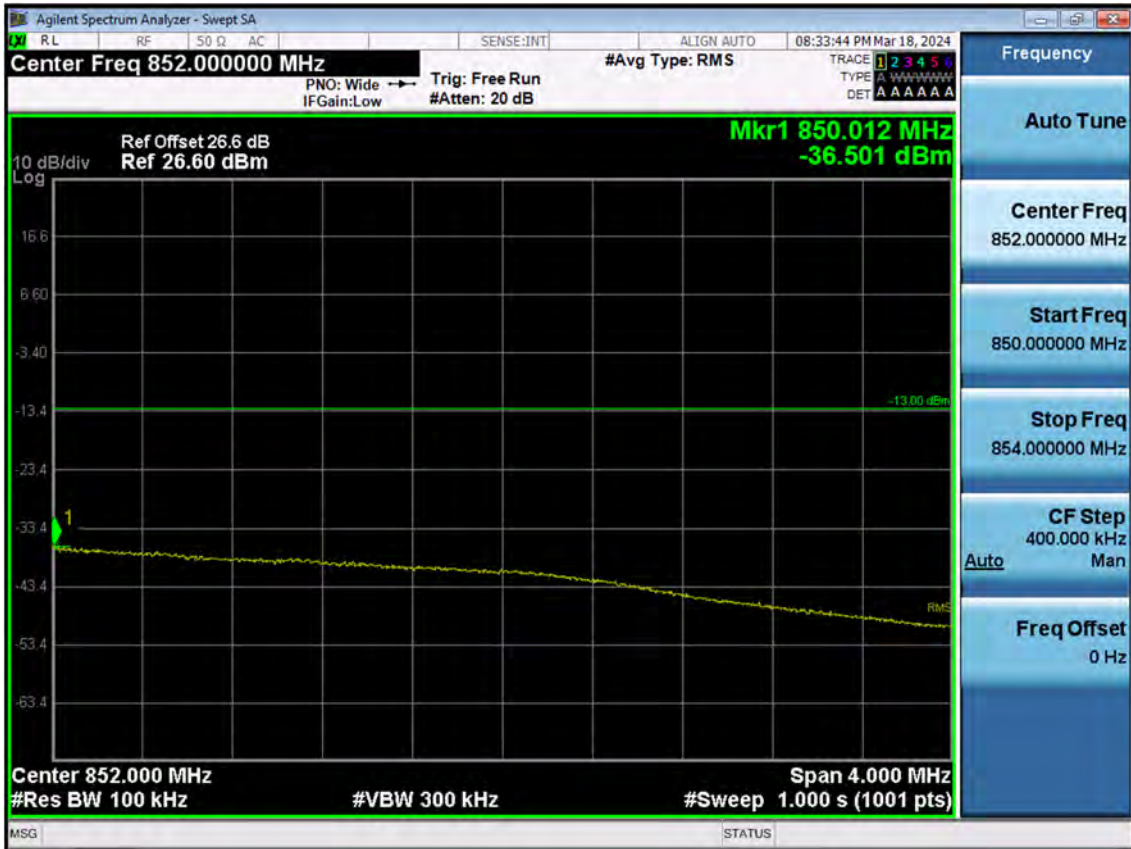
BAND5/26. Upper Extended Band Edge Plot (5 M BW Ch.27015 QPSK_RB25_0)
