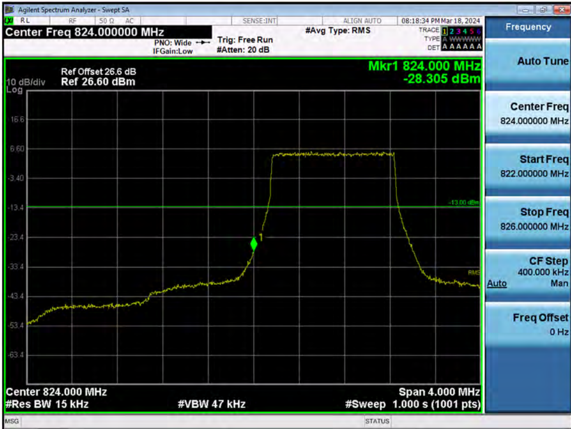
BAND5/26. Lower Band Edge Plot (1.4 M BW Ch.26797 QPSK_RB6_Offset 0)
