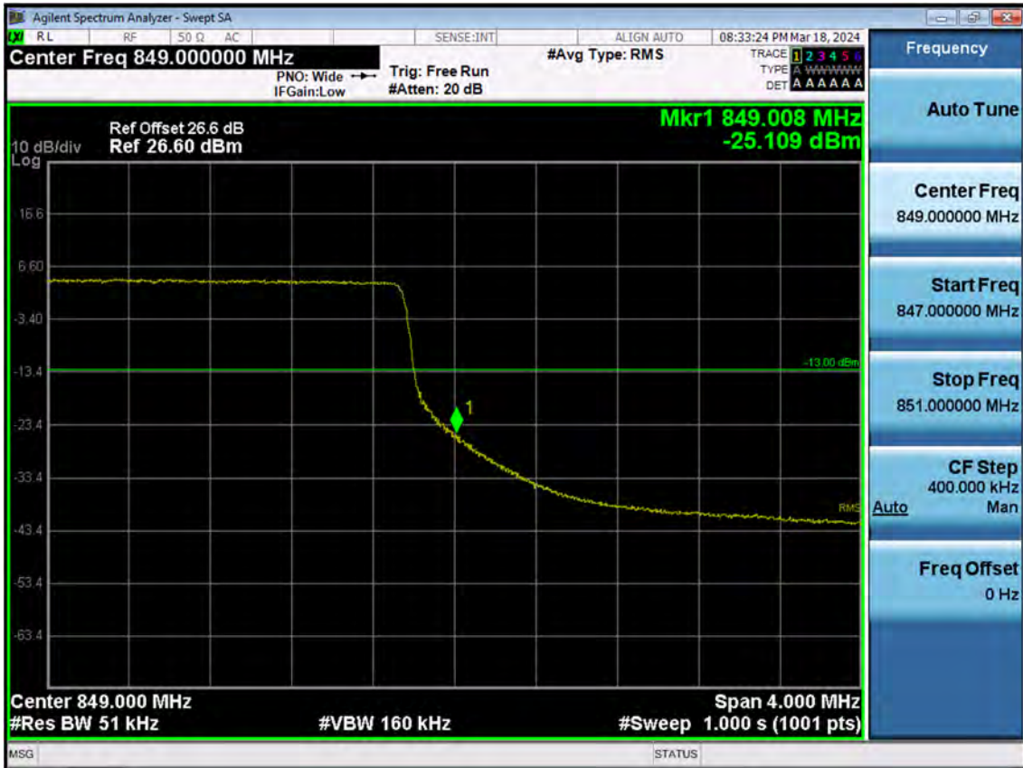
BAND5/26. Upper Band Edge Plot (5 M BW Ch.27015 QPSK_RB25_Offset 0)
