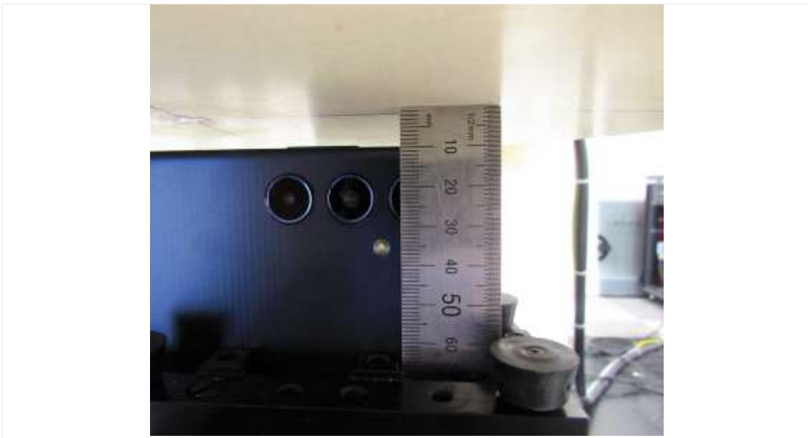
Distance of 10 mm from the EUT
