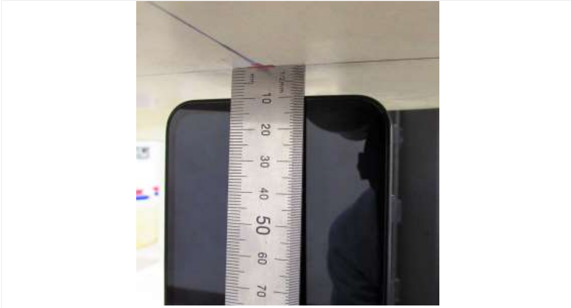
Distance of 10 mm from the EUT
