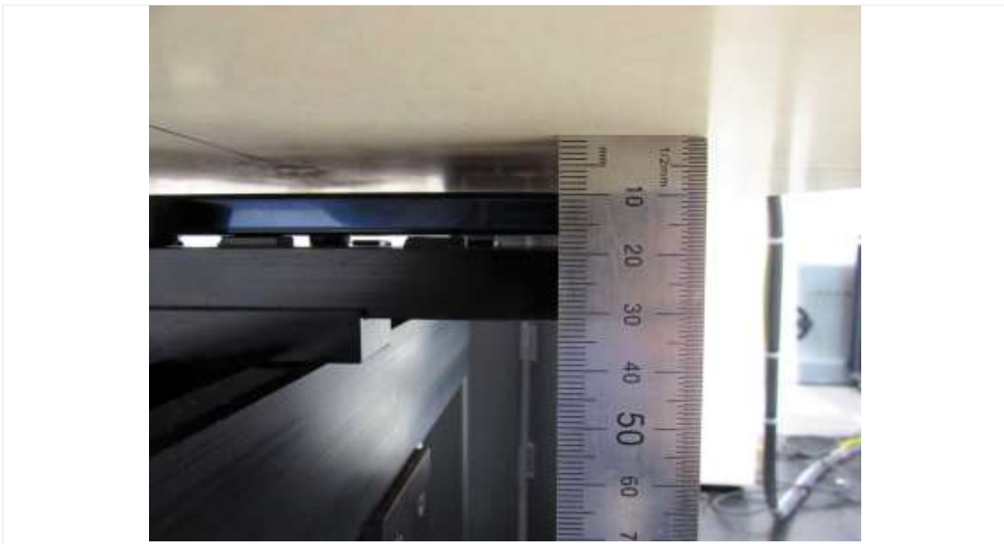
Distance of 10 mm from the EUT
