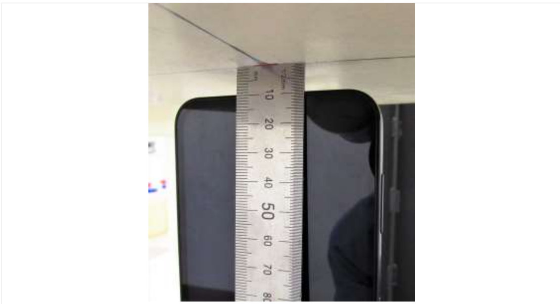
Distance of 10 mm from the EUT
