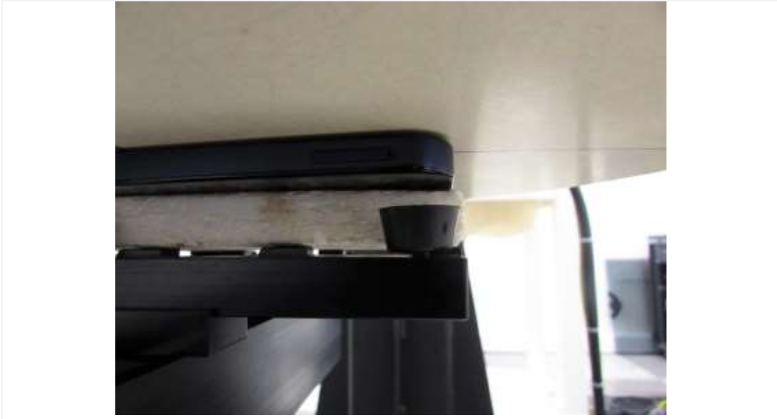
Distance of 0 mm from the EUT
