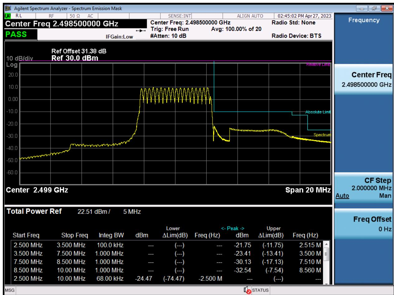
LTE41\_5 M\_BandEdge\_Lower\_Low\_2498.5 MHz\_QPSK\_1RB
