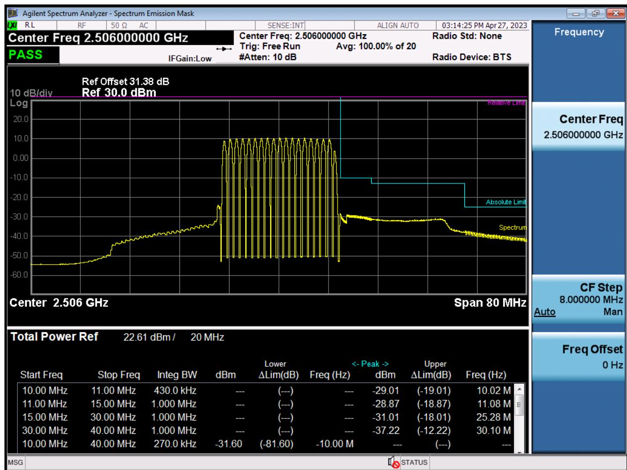
LTE41\_20 M\_BandEdge\_Lower\_Low\_2506 MHz\_QPSK\_1RB
