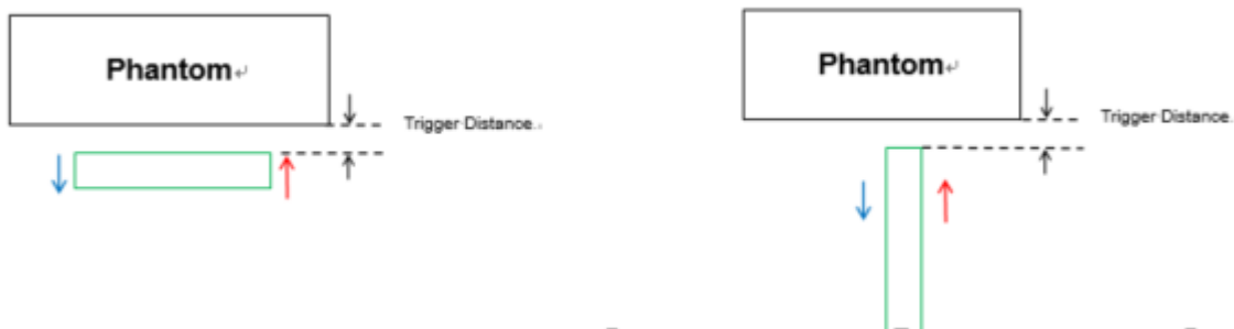
Proximity Sensor Trigger Distance Assessment KDB 616217 D04§6.2
