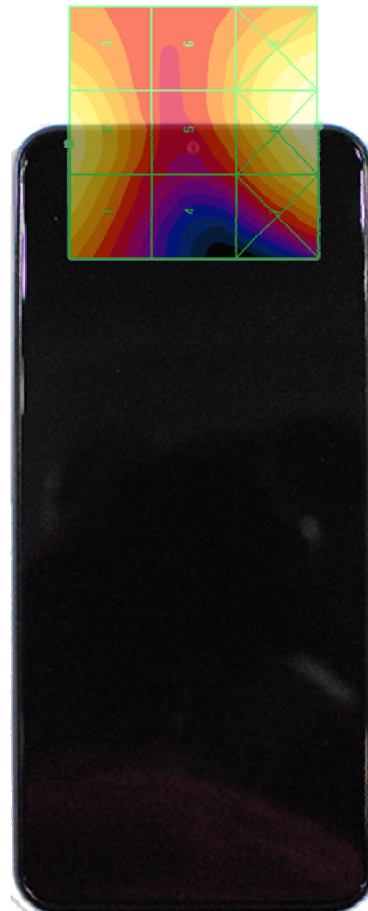
Figure 18-4 E-Field WD Scan overlay
