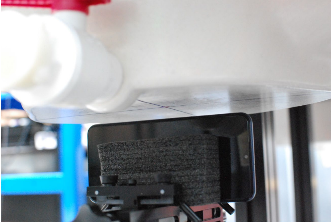
SAR Test Setup Photo 17 – Hotspot, Left Edge at 10 mm
