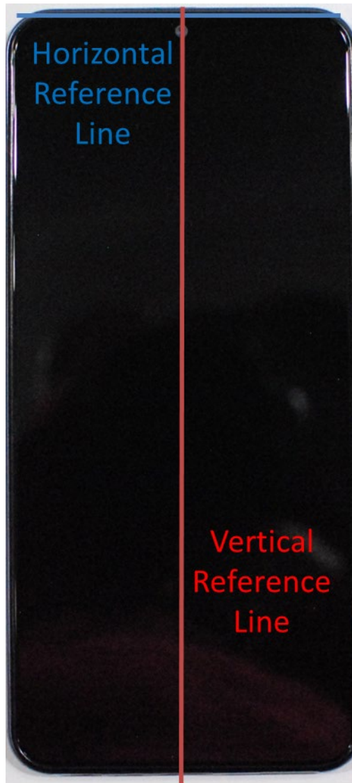
SAR Test Setup Photo 19 – Horizontal and Vertical Reference Lines
