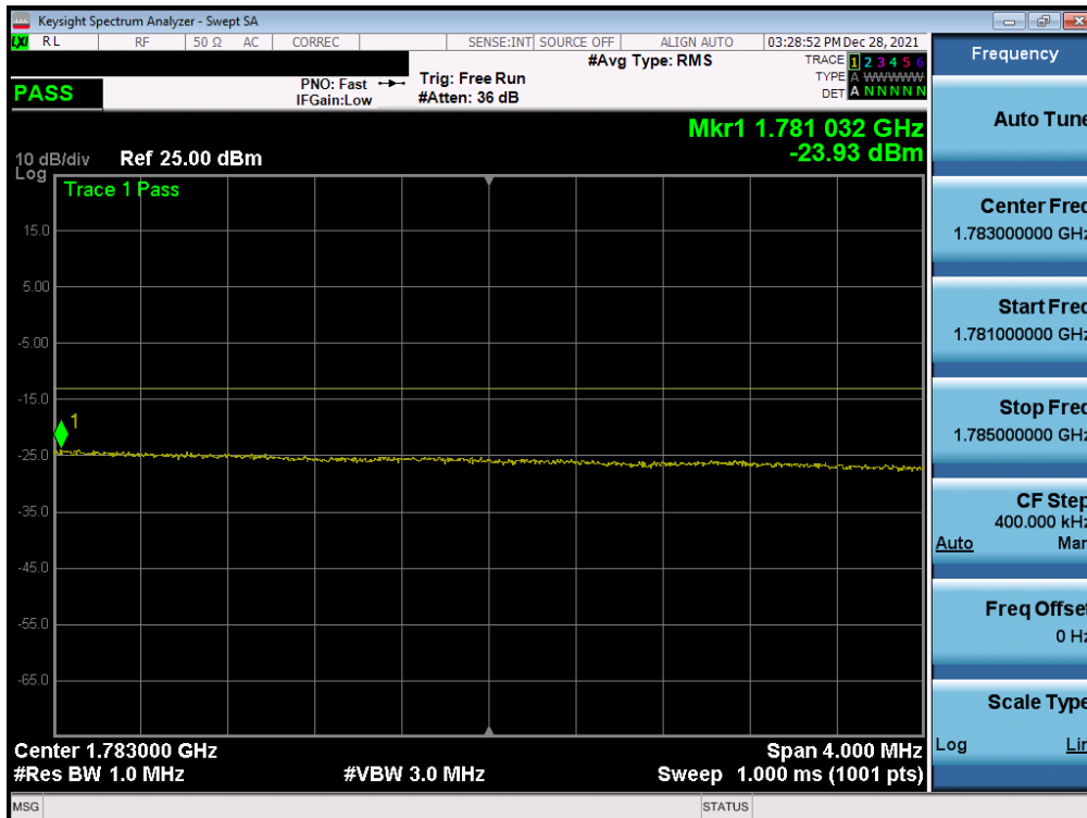
Plot 7-91. Upper Extended Band Edge Plot (LTE Band 66 - 15MHz QPSK – Full RB)
