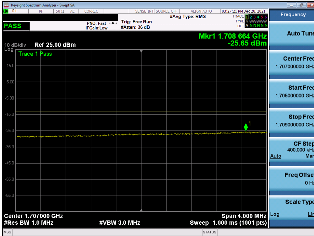
Plot 7-81. Lower Extended Band Edge Plot (LTE Band 66/4 - 20MHz QPSK – Full RB)
