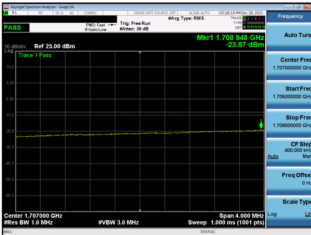
Plot 7-87. Lower Extended Band Edge Plot (LTE Band 66/4 - 15MHz QPSK – Full RB)
