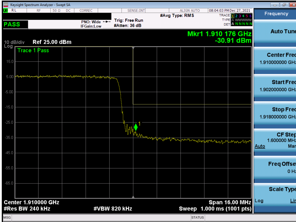
Plot 7-45. Upper Band Edge Plot (LTE Band 2 - 20MHz QPSK – Full RB)
