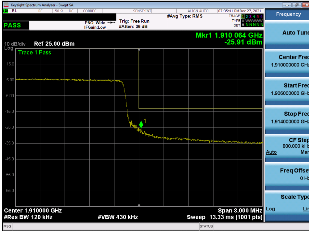
Plot 7-53. Upper Band Edge Plot (LTE Band 2 - 10MHz QPSK – Full RB)
