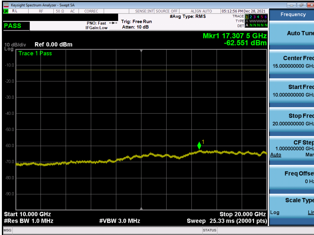
Plot 7-42. Conducted Spurious Plot (WCDMA Ch. 9538)
