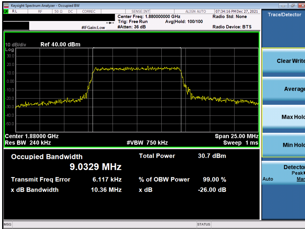
Plot 7-5. Occupied Bandwidth Plot (LTE Band 2 - 10MHz QPSK - Full RB)
