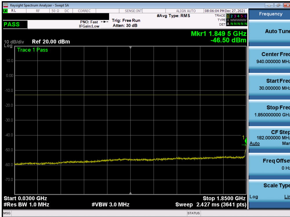
Plot 7-19. Conducted Spurious Plot (LTE Band 2 - 20MHz QPSK - 1RB - Mid Channel)
