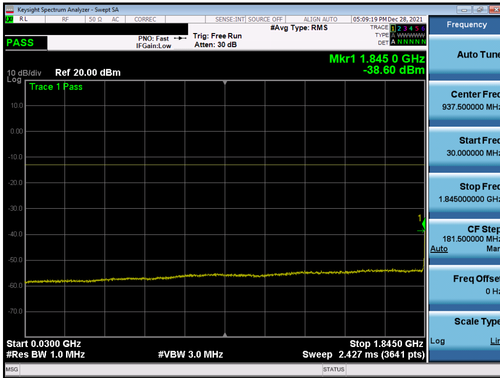
Plot 7-34. Conducted Spurious Plot (WCDMA Ch. 9262)
